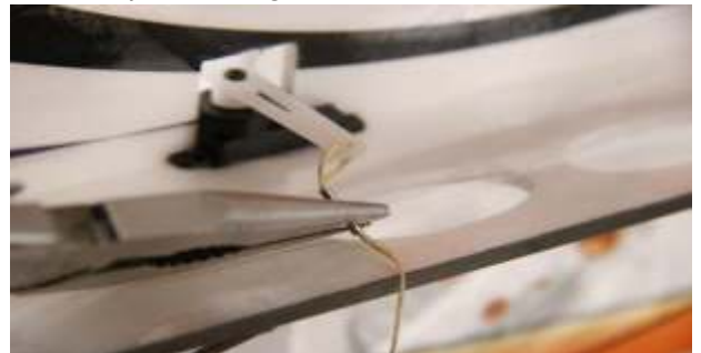
29. Then thread through the hole on rudder servo arm. Stave steel tube with plier and fix with CA.
