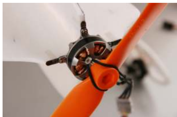
21. Fix propeller with o ring.
