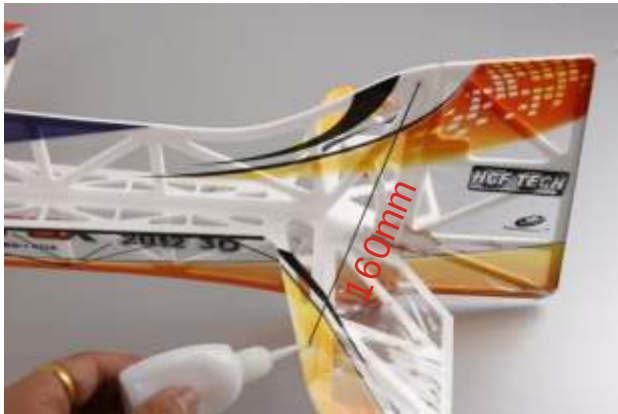
14. Install carbon fiber bracings between two wings.
