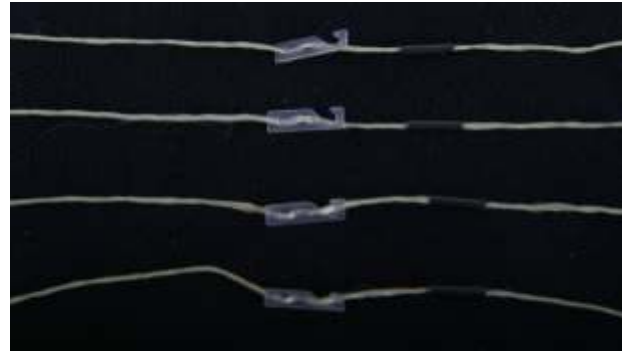
27. Across thread through 3 holes on pull-pull thread adjustor.
