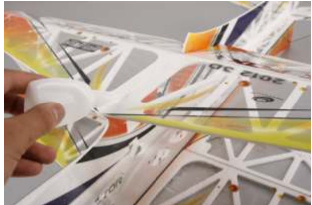
8. Insert upper vertical fuselage into the slot of horizontal fuselage, then use CA to fix. Notice: make sure both fuselages are perpendicular to each other.
