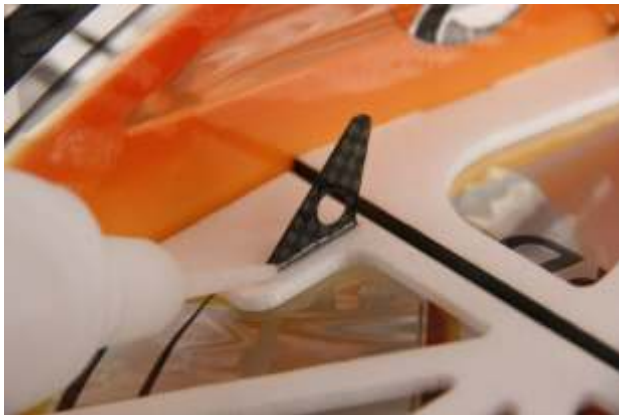
17. Install 2pcs aileron control horns on back wings.
