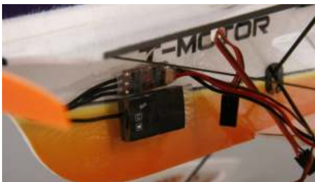
36. Connect servo and ESC to receiver, then power on and do equipment test.
