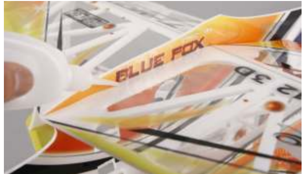
10. Install wing fences on corresponding places of bottom wing and fix with glue.
