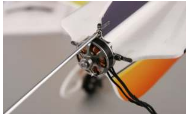
20. Install motor on motor mount with 4pcs self tapping screws.
