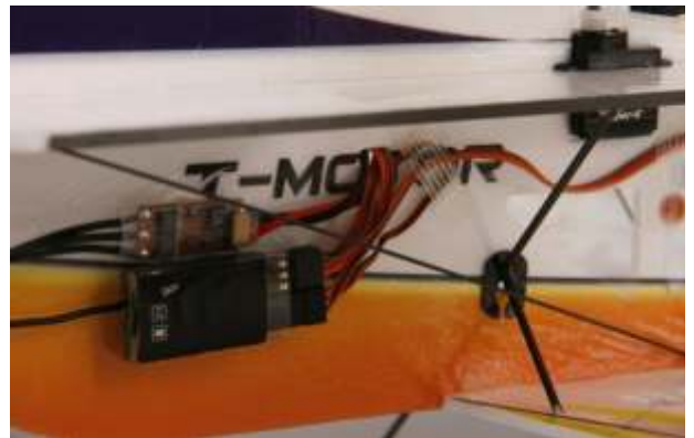
35. Pass all servo wires through fuselage and place them close to receiver.
