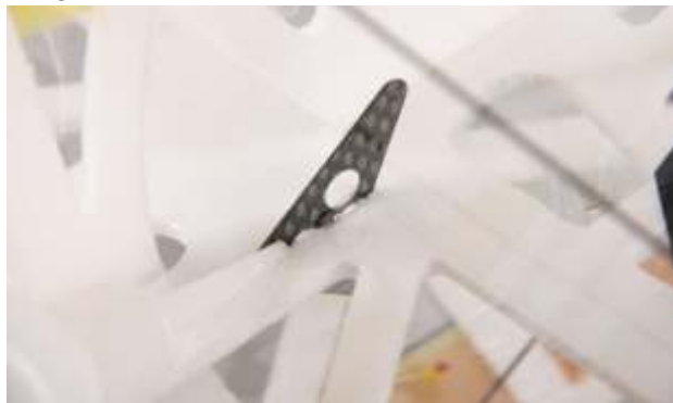
18. Install elevator control horns.
