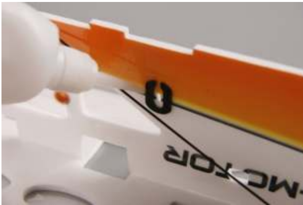
6. Fix landing gear reinforcements to corresponding hole with glue.
