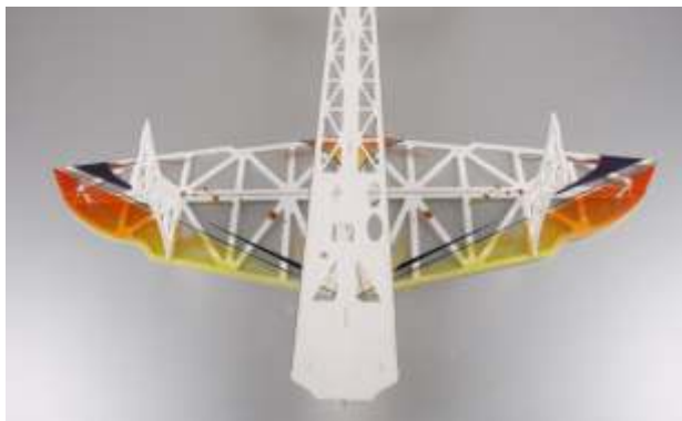
7. Fix left and right wing supporting foam with glue.
