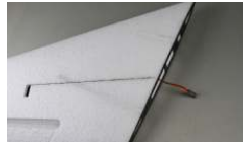
7. Embed the servo wire into slot.
