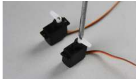
2. Install servo arm as picture shown.
