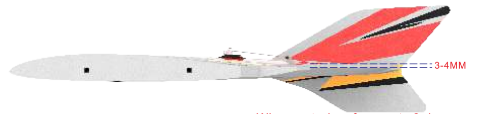
Wing control surface up to 3-4mm
