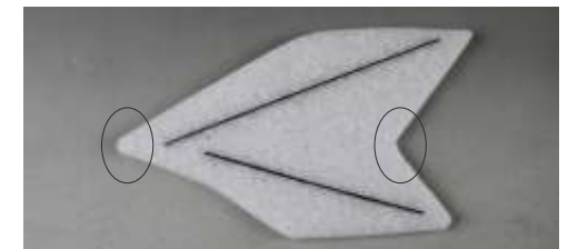
12. The pointed position in black circle is the adhesive position of wing fence, which would be glued on the wingtip.
