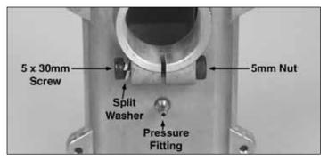
Install the 5mm x 30mm screw, split washer and 5mm nut in the muffler, but do not tighten. Slide the muffler over the
