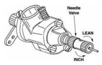
4. Gently turn the high-speed needle valve clockwise until it stops. Do not tighten it. Then open it 4 turns. Turning the high-speed needle in a clockwise direction is called "leaning" the mixture, and turning it counterclockwise is called "richening" the mixture.
