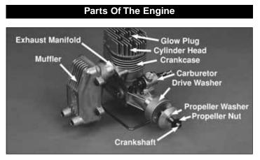
**Crankshaft:** The crankshaft transforms the reciprocating motion of the piston into rotational motion. The propeller is mounted on the portion of the crankshaft protruding from the crankcase. The portion of the crankshaft protruding past the drive washer is known as the "prop shaft."
