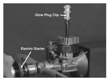
**Securely** attach the glow plug clip to the glow plug. If using a glow plug clip connected to the power panel of a field box,
