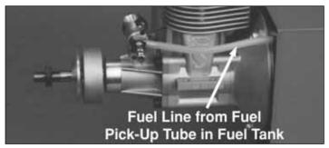
Connect a medium or large size silicone fuel line from the fuel inlet on the carburetor to the fuel pick-up tube that is connected to the clunk in the fuel tank. We suggest that a fuel filter be installed in the fuel line between the carburetor and the fuel tank. The filter will prevent any contaminants in the fuel from clogging the carburetor.
