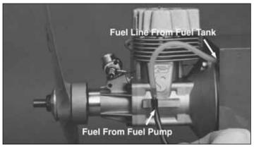
3. Fill the fuel tank by removing the fuel line from the fuel inlet on the carburetor, and connecting it to the fuel tubing from the fuel pump. Remove the pressure line from the pressure fitting on the muffler and direct this fuel into an "overflow bottle." Start filling the fuel tank. When the tank is full, fuel will overflow out of the pressure line. Disconnect the fuel pump from the fuel line and reconnect it to the carburetor. Reconnect the pressure line to the muffler pressure fitting.
