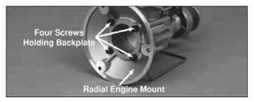
If the G3250 engine is to be mounted on the radial mount provided with the engine, remove the four screws holding the backplate. Remove the rubber O-ring on the backplate and install it on the radial mount. Attach the radial mount to the engine using the four longer screws and split washers provided. Install the radial mount to the firewall of the airplane with three 8-32 screws, three split washers and three blind nuts. (Not Included.)
