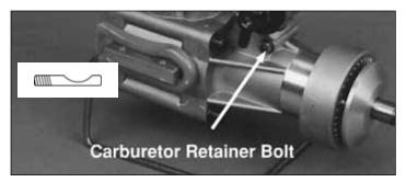
Insert the carburetor retaining bolt (the bolt has a curved area removed from its center) into the hole in front of the carburetor opening. Rotate the retaining bolt so that the removed area in the bolt matches the curve of the carburetor opening. Install the split washer and the brass nut on the threaded end of the bolt. Insert the carburetor in the carburetor opening and press down on the carburetor while tightening the nut.
