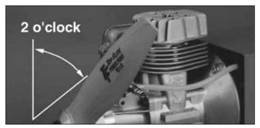
2. Locate the correct propeller for your airplane from the propeller chart on page 18. Ream the propeller hole to the appropriate diameter using a prop reamer. Balance your propeller using a prop balancer. To install the propeller on the engine, remove the propeller nut and propeller washer. If installing a spinner, install the spinner backplate first, following the manufacturer's instructions. Trim the spinner cone as
