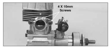
Use two 4mm x 10mm size screws and split washers to attach the exhaust manifold to the engine. Make sure to install the gasket between the manifold and the engine and tighten the screws securely.
