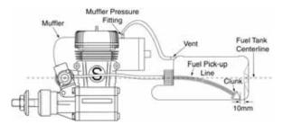
When the engine is mounted in the upright position, the centerline of the fuel tank should be at the same level as the
