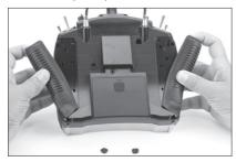
Step 2. Using a Phillips screwdriver, adjust the stick tension screw for the desired control. Clockwise to tighten and counterclockwise to loosen.
