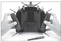
Step 2. Remove the back case noting that a wire harness connects the back to the main case. Carefully set the main case to the left side of the transmitter being careful not to damage the wire harness.
