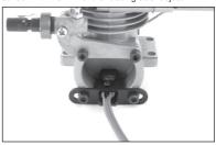
**Note:** On some engines you may need to space the sensor further away from the backplate. The sensor picks up the crankpin only; on some engines if the sensor is too close, it will not distinguish the crankpin from the crank weight.
