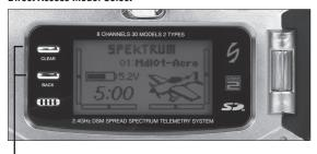
Press the Clear and Back buttons simultaneously to access the Model Select screen
