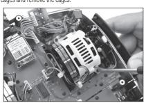
Step 7. Most pilots prefer having a throttle with less stroke as it provides a more natural feel when giving rudder commanded (mode 2) at full or low throttle. When changing throttle position from right to left it's necessary to switch the throttle limiting wedges positions. Using a Phillips screwdriver remove the throttle limiting wedges from their current position and reinstall them on the opposite gimbal.
