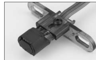
Bracket adjusted for 90-size engine
