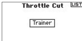
Program a Throttle Cut position. Note that 0%= low throttle, mid trim and negative values are available. To test the Throttle Cut function, activate the programmed switch. Note the throttle servo position or the position of the throttle channel in the servo monitor. The system should drive the servo position to the low throttle position when you activate Throttle Cut.
