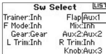
Rotate the roller to select the desired channel or function you wish the switch, knob or trimmer to operate. Press the roller to accept. Note that the channel or function can only be assigned once.
