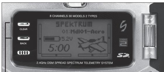
Press the Clear and Back buttons simultaneously to access the Model Select screen
