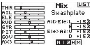
Verify that the Swash mix is working properly and in the correct direction by placing the flight mode switch in one of the active positions. Then, move the programmed cyclic master channel aileron or elevator to its full travel and hold this position. Now change the flight mode to a position that the swash mix is inactive in. Note the movement of the slave channel on the left side of the monitor.
