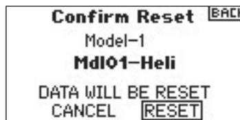
Verify that the model displayed on this screen is the model you wish to reset. If not then see page 14 Model Select to access the desired model. Rotate the roller to highlight Reset and then press to access the Confirm Reset screen.
