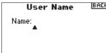
Highlight the desired character position then press the roller to access that position. Rotate the roller to change to the desired character. Press to accept. Repeat the process until the name is complete. Note that the User Name displays on the lower left of the startup screen.
