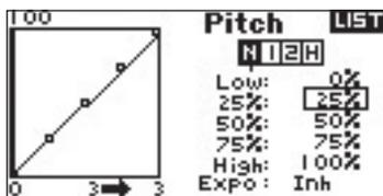
Rotate the roller to adjust the selected point to the desired output position. Note the position on the graph at the left of the screen.
