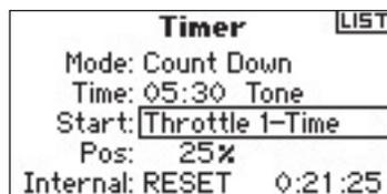
Rotate the roller to select the desired Start method (Trainer, Throttle, Throttle 1-Time, L Trim, R Trim). Press to accept.
