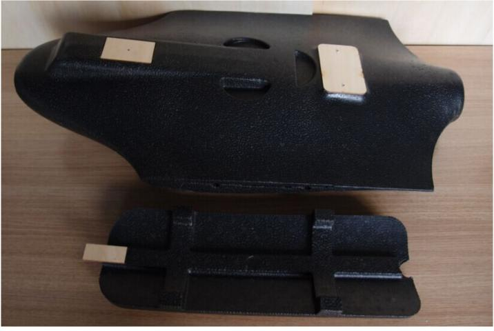
1. Install the fuselage connection plastic parts accordingly (L and R). Notes: Insert the 2pcs carbon tube to the fuselage
