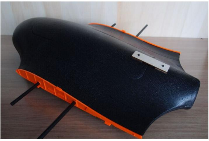
2. Fuselage assembly. Glue the plastic parts to the wing separately. Then install the servos, servo horns and push rods.
