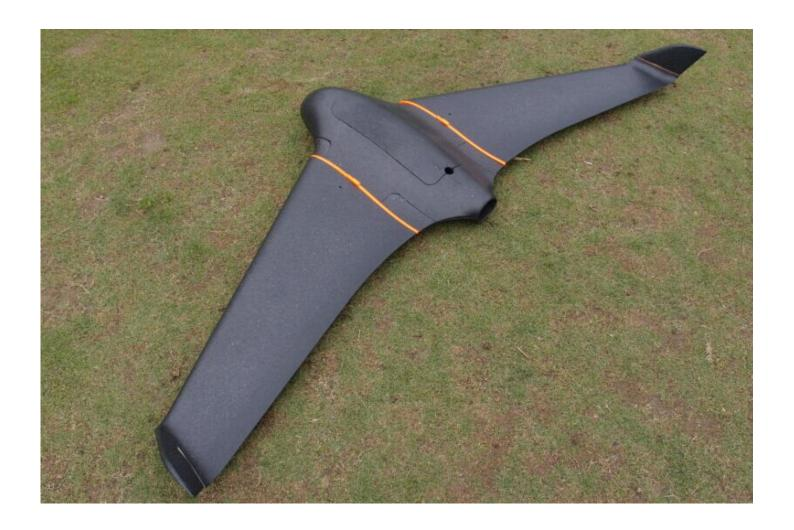
Finally, Please note that , control X - 8's flight speed within 85 km/H. If you need a high speed flight, please strengthen wings. please control the machine load within 3200 g, if exceed the limit, please strengthen wings. Thank you again for choosing skywalker series products. If there are technical problems or suggestions, please email us for consultation. Or consult your local dealer.
