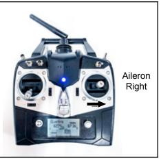
When the aileron stick is moved to the right of the transmitter the right aileron should move up and the left one move down. This will roll the wing to the right.
