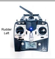
PLEASE NOTE: The throttle/rudder stick must be raised a few clicks from bottom position in order to activate the rudder operation. The throttle stick at the fully off position is reserved for arming and disarming of the motors as shown on page 11.
