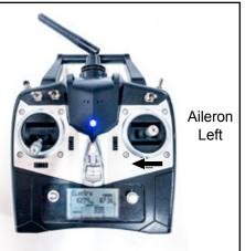
When the aileron stick is moved to the left of the transmitter the left aileron should move up and the right one move down. This will roll the wing to the left.
