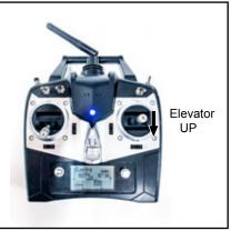
The PASS switch on the upper right of the transmitter should be in the OFF (toward back of transmitter) for these tests.
