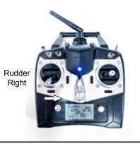
When the rudder stick is moved to the right of the transmitter both rudders should move right. When in flight this will yaw the tail to the left (the nose of the aircraft will move to the right).
