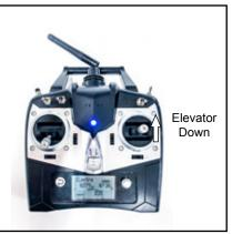
When the elevator stick is moved toward the top of the transmitter both elevators should move down. When in flight this will lower the nose.
