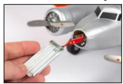
The nose of the fuselage is held in place by magnets. Remove the nose by gently grasping the sides and pulling forward. Once nose is removed, plug the charged flight battery into the lead, being careful to align the red dots to ensure correct polarity. Slide the battery into the aircraft with the battery lead facing the rear of the aircraft. The battery will be held firmly in place in the battery box.
