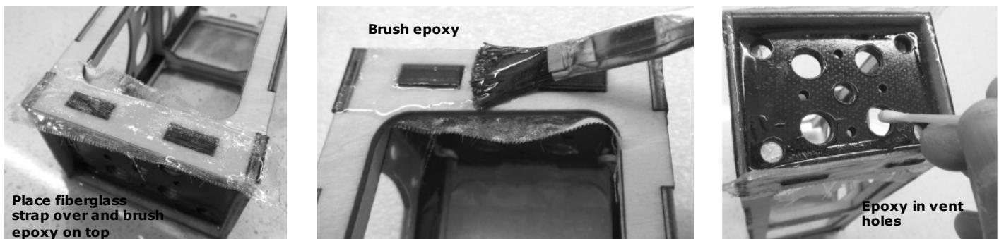
7. Using a cotton bud apply a thin layer of epoxy in the firewall vent holes except the mounting holes . wipe off any excess where the motor is mounted
