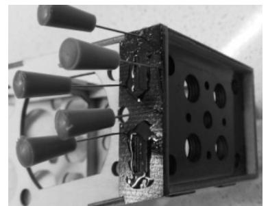
Apply some epoxy over the firewall tabs and along the rear seam of the plates, especially if there is some gap between the plates and ply.
