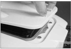
2. Remove the radio box cover from the hull by lifting it up using the tab at the rear of the cover.
