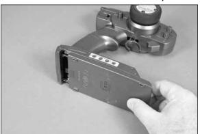
3. Install the four AA batteries in the battery holder. Match the polarity of the batteries to the molded markings in the battery holder.
