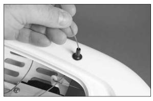
O 5. Use clear tape to secure the shorter feed antenna under the lip of the hull. Make sure the tape will not interfere with the installation of the radio box cover.
