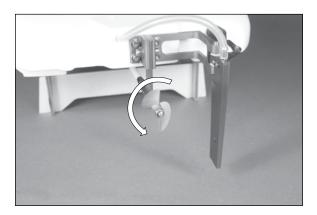
O 5. Check the operation of the steering in relationship to the steering wheel. When the wheel is rotated clockwise, the rudder must move right as shown. If not, follow the instructions from the radio to set the servo reversing for the steering.
