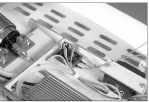
4. Pass the longer antenna wire through the fitting on the top of the hull. The antenna wire is then inserted into the antenna tube. Place the antenna tube in the fitting to complete the main antenna installation.
