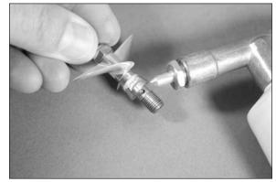
O 7. Reverse the previous steps to reassemble the flex drive in the motor. You will need to rotate the parts slightly so they key back together correctly during assembly.
