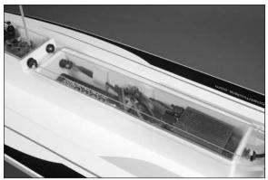
G. Check the operation of the steering in relationship to the steering wheel. When the wheel is rotated clockwise, the outboard motor must move right as shown. If not, follow the instructions from the radio to set the servo reversing for the steering.
