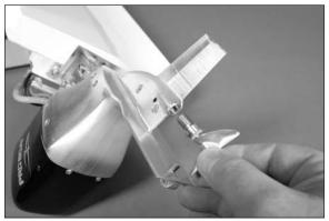
• 3. Use needle nose pliers to grab the flex shaft, removing it from the lower end.
