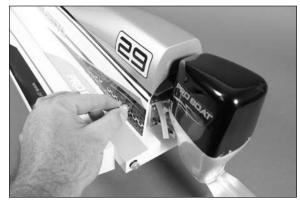
• 3. Remove the clear battery cover from the hull. Place the motor batteries in the hull. The rear battery fits under the speed control, and the forward battery lays flat in the radio compartment. This keeps the center of gravity low for the best handling of your model. Use the hook and loop tape supplied with your model to keep the batteries from moving in the hull.
