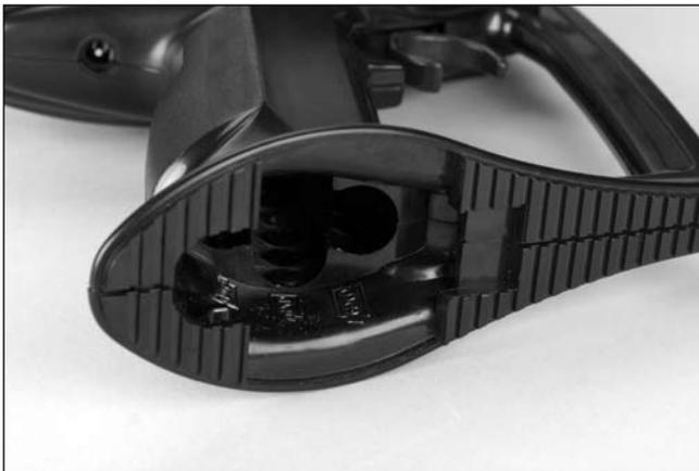
3. Install the AA batteries into the transmitter. Be aware of the proper polarity when inserting the batteries.
