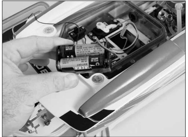
4. Place the battery holder back into the radio box. Confirm the switch is in the "off" position after installing the batteries.
