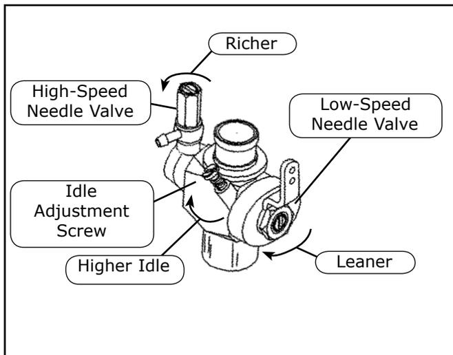
The Nitro engine comes equipped with the Pro Mix Carburetor. Each Pro Mix Carburetor is pre-adjusted at the factory. This setting should be approximately 3-1/2 turns open for the high-speed and 2-1/2 turns open for the low-speed needle. This should give you a slightly "rich" mixture of fuel to the engine. This setting is the safest way to break in your engine. For further details regarding the Pro Mix Carburetor, please consult the included engine manual.
