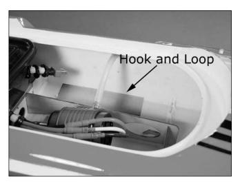
Confirm that the switch inside the boat is in the "OFF" position. Install two fully charged 7.2V Ni-MH battery packs into the hull.
