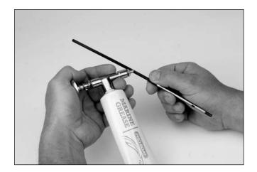
**Note**: Running the Formula Fastech 26 Brushless EP RTR in salt water could cause some parts to corrode. If you run the boat in salt water, rinse it thoroughly in fresh water after each use and lubricate the drive system.
