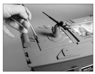
Carefully lift the rear cover at the rear. A tab holds the cover at the front, so pull the cover rearward to release the tab. Set the cover aside in a safe place.
