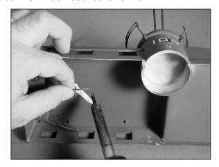
Use heat-shrink tubing or electrical tape to insulate the connection made in the previous step.
