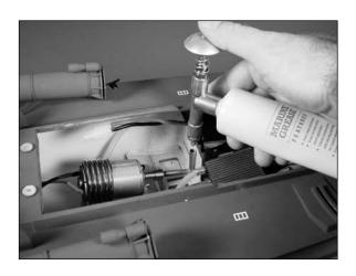
Periodically, you may have to remove the driveshafts to remove build-up. Lubricate the shaft prior to installation.
