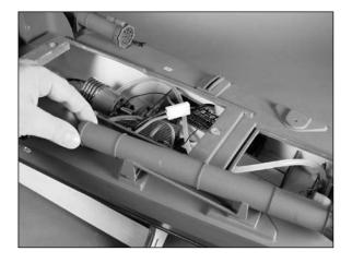
Slide the rear mast into the tube at the rear of the hull.
