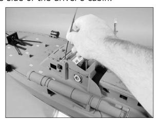
Slide the spotlight into position in the tube next to the driver's seat.
