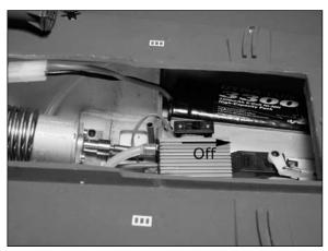
Plug the connectors from battery packs to the connectors from the ESC.
