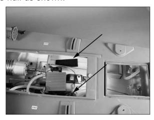
Install the battery packs into the hull as shown. Batteries are located on the left and right side of the hull.
