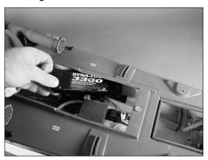
Confirm the receiver switch has been set to the "OFF" position at this time.
