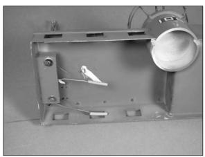
The switch to turn the accessory lighting on is located on the left side of the hull near the motor. The lighting will only power on when the batteries are connected to the speed controller. With the batteries plugged in, turn on the lighting and place the forward hatch in place. Sit back and enjoy the glow from the scale lighting of your PT-109.
