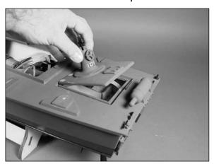
The torpedos are attached to the hull using a tab at the front and a piece of rubber tubing at the rear. Once the torpedos are in place on the hull, you will need to slide the tubing onto the threaded studs from inside the hull.
