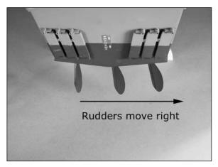
It may be necessary to adjust the Steering Trim so the rudders are centered prior to operation. Use the Steering Trim to center the rudders prior to operation. You may also need to fine-tune the steering trim to make sure the boat runs straight during operation. This can only be accomplished when operating the boat in the water and is detailed in a following section.
