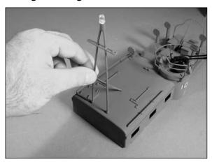
Carefully solder the wires together to power the navigation light, making sure to connect the red wire to the red wire and the black wire to black wire. The electrical connection to power the light is made at the front magnets when the hatch is mounted to the hull.
