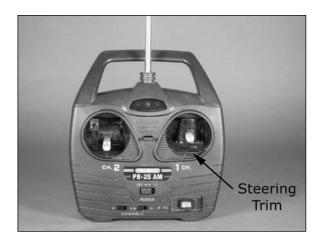
After you have completed checking your radio system, turn the PT-109 receiver off FIRST by sliding the switch to the "OFF" position. After the model has been turned off, turn off the transmitter.
