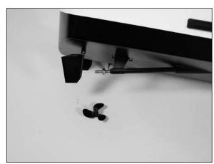
Use a 1.5mm hex wrench to loosen the setscrew that secured the drive shaft to the motor adapter.
