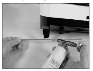
Slide the shaft back into the stuffing box. Use a paper towel to remove excess grease near the propeller that oozes out when inserting the shaft.
