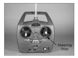
After you have completed checking your radio system, turn the Motor Lifeboat receiver off FIRST by sliding the switch to the "OFF" position. After the model has been turned off, turn off the transmitter. Turning off the transmitter first may allow the radio to accept stray signals and the boat may run out of control.
