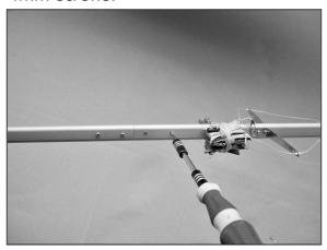
3. Locate the main sail boom and connect it to the main mast with a screw and nut.
