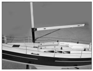
O 6. Remove the masthead crane and slide the unrolled main sail to the bottom of the mast.
