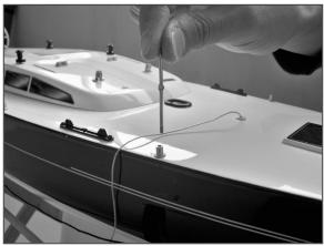
O 6. Insert the line into the hole of the railing.
