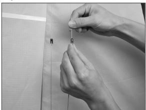
O 12. Pass the rigging line of the jib sail through the eye plate on the mast and then thread the line into the jib stay. Thread the line through the swivel and tie an overhand knot to the jib stay to secure. Connect "I" to "I" as shown in the picture.
