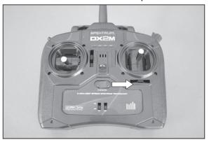
4. Move the stick on the transmitter to the right. The rear edge of the rudder will move to the right as shown. Actuate the STR (steering) reversing switch if the direction is reversed.
