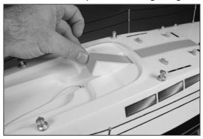
2. Remove the nylon bolt that secures the hatch cover to the hull.
