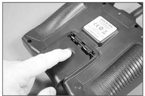
2. Install four AA-size batteries in the transmitter. Make sure to match the polarity of the batteries to the polarity molded into the battery compartment of the radio. Slide the cover back into position on the radio.
