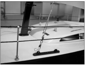
O 11. Pull up carefully on the jib stay to adjust the tension of the lines.
