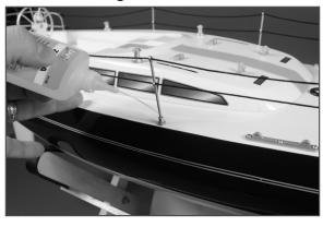
11. Apply a drop or two of thin CA to each of the points where the stern railing fits into the railing stands on the hull.
