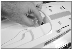
O 3. Set the hatch cover aside. The cover cannot be fully removed as the line to the sail passes through the hatch cover.
