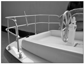
• 5. Put the railing into the railing stand.
