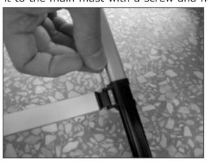
4. Install the adjust support which connects the main mast and main sail boom.
