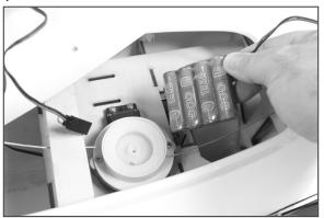
3. Check the switch harness to make sure it is in the OFF position. Plug the receiver battery into the switch harness. Make sure to match the polarity of the plugs so the black and red wires align with each other.
