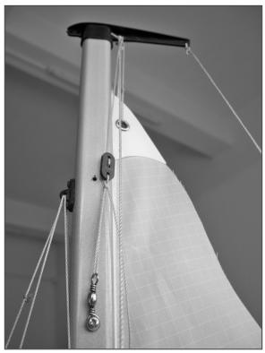
O 16. Pull up the jib stay on the jib boom to adjust the tension of the lines.
