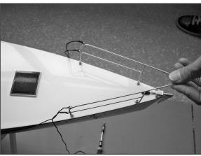
• 4. Locate the stern railing and insert it into the railing stands.
