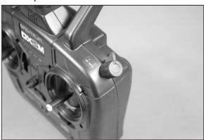
O 5. With the radio system on, move the left stick on your transmitter "up" and manually push the main sail and jib sail open. You should be able to open the sails to at least a 60-degree angle. If you cannot do this, it will be necessary to adjust the length of the line (allowing more slack) by adjusting the jib stays located underneath the main sail and jib sail booms.
