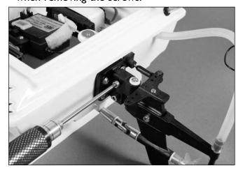
• 4. Move the rudder assembly and slide the drive shaft out of the stuffing box.
