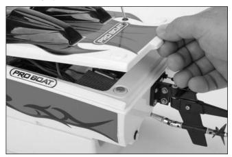
Make sure the receiver switch is in the "OFF" position. Install a fully charged 7.2V Ni-Cd battery pack into the radio box. Follow the instructions included with your fast charger to ensure a safe charge. Plug the battery into the female battery connector attached to the electronic speed controller.
