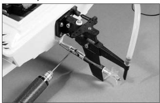
3. Remove the two 3mm screws from the outdrive to separate the rudder assembly from the mount. Make sure not to lose the 3mm nuts when removing the screws.
