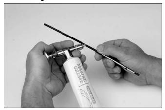
**Note**: Running the Apache 24 EP RTR in salt water could cause some parts to corrode. If you run the boat in salt water, rinse it thoroughly in fresh water after each use and lubricate the drive system.
