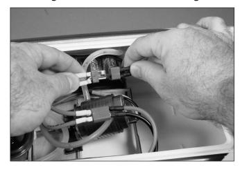
Attach the hook and loop material to the batteries and the battery boxes. Install two fully charged 7.2V Ni-MH battery packs into the hull.
