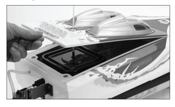
The Pro Boat water-cooled ESC comes pre-wired with a Deans-style connector. Use 2 6-cell battery packs listed below for optimum performance.
