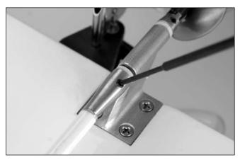
O 6. Carefully re-install the flex shaft and nylon bushing, making certain that you correctly tighten the collet nut. Next, re-install the drive shaft and propeller and tighten the setscrew on the flat of the drive shaft. Use screw locking compound to secure the setscrew.
