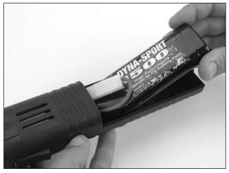
O I. Fully charge a 7.2V sub-C battery pack and install it in the starter as shown.
