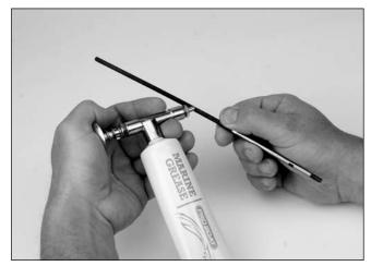
O 5. Liberally lubricate the entire length of the flex shaft with silicone cable grease as shown.
