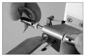
O 2. Loosen and remove the 1.5mm setscrew that holds the propeller shaft. Remove the propeller and shaft from the aluminum strut.
