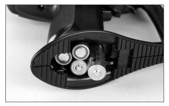
3. Install the "AA" batteries into the transmitter Be aware of the proper polarity when inserting the batteries.
