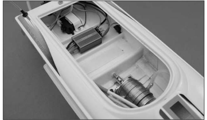
Install a fully charged battery pack into the hull.
