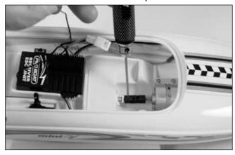
• 2. Loosen the 1.5mm setscrew connecting the universal joint to the drive shaft.
