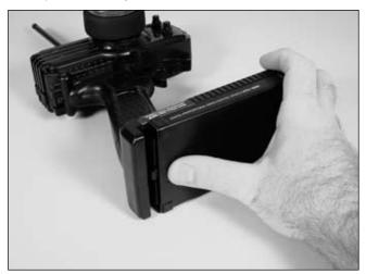
Install 8 "AA" alkaline batteries into the transmitter. Pay attention to the proper polarity (+ and -) for the batteries as marked on the battery holder.
