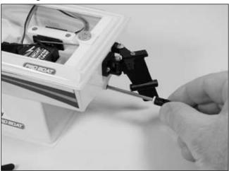
O 5. Lubricate the drive shaft and propeller shaft with water-proof grease (see your local hobby shop). Reinstall the drive shaft and propeller shaft in reverse order. Be sure to reinstall the nylon washers between the universal and the stuffing box at the motor, and between the propeller and rudder assembly for the propeller shaft.
