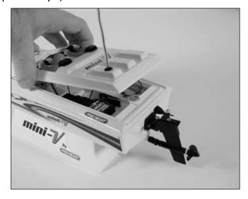
Remove the backing material from the hook & loop material and use it to secure the battery into the battery holder. Install a fully charged 7.2V Ni-MH battery pack into the radio box. Follow the instructions included with your fast charger to ensure a safe charge. Plug the battery into the female battery connector attached to the electronic speed controller.
