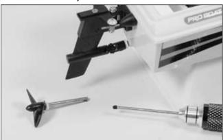
• 4. Move the rudder assembly to either full left or full right turn and slide the drive shaft out of the stuffing box.
