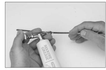
• 4. Lubricate the entire flex cable with waterproof grease as shown and then re-install the flex cable back through the liner and stuffing box and into the clutch.
