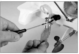
O 3. Find the flat spot on the rudder. Put screw-locking compound on the 2.5mm hex screw threads and tighten the screw on the flat spot as shown.
