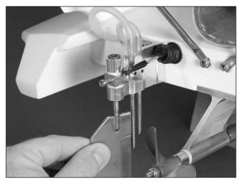
O 2. Carefully insert the rudder as shown.
