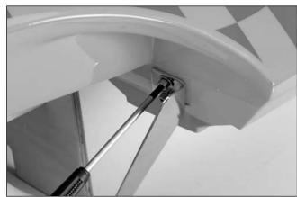
O 5. Carefully attach the turn fin onto the right sponson as shown and tighten the hex screws with a 3mm hex driver.
