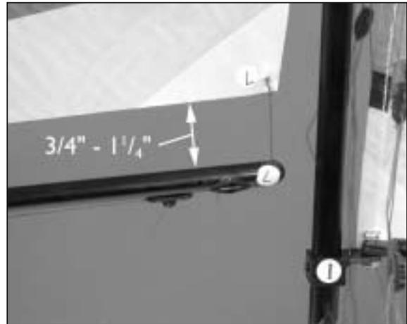
**Hint:** The jib boom will be parallel to the bottom of the jib sail once Steps 17 and 18 are complete.
