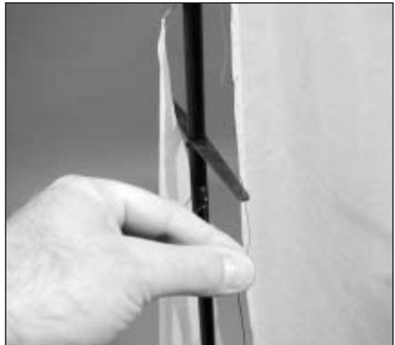
**Note:** The spreader has a small notch in the outer hole. The inner hole will not be used, making it easier to insert the line. Simply push the rigging line through the slot.
