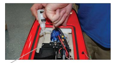
Carefully lift the radio tray up and apply CA between the tray and Hull <
