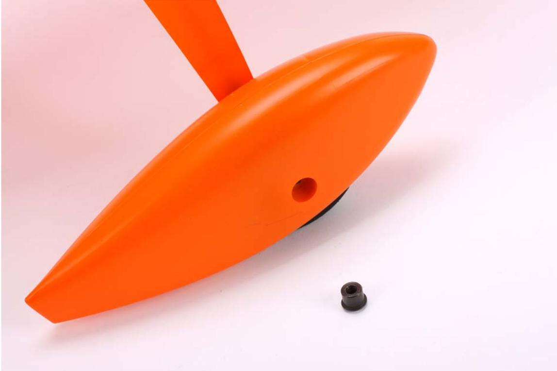
2. Apply a small amount of thread-lock to the inside of the wheel nut.
