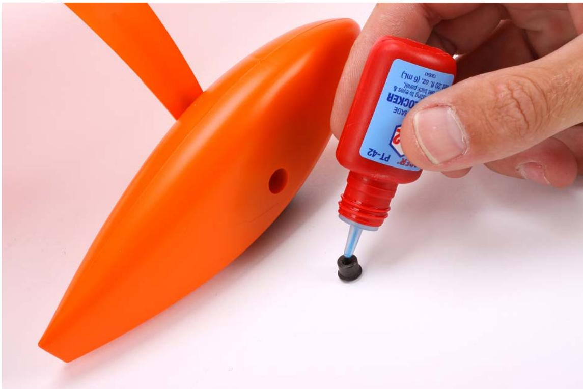
3. Install the wheel nut and allow the thread-lock to thoroughly dry.
