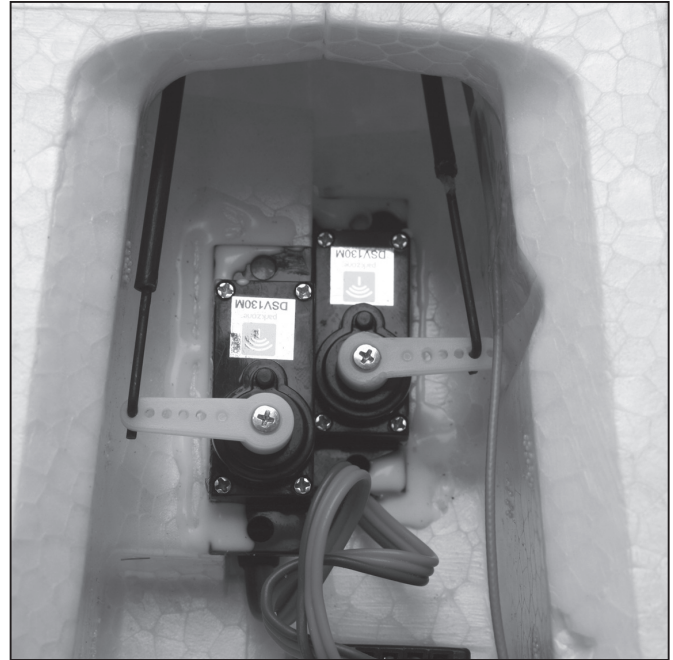
Extreme Setting for Rudder and Elevator Servo Arms and Pushrods
