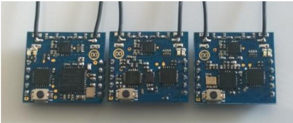
(From left to right: DSMX/DSM2-7CH compatible receiver; Futaba SFHSS-8CH compatible receiver; Flysky AFHDS-8CH compatible receiver)
