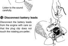
If the engine stops when battery leads are disconnected, close the needle-valve a little (approx, 45°) further, and restart the engine.
