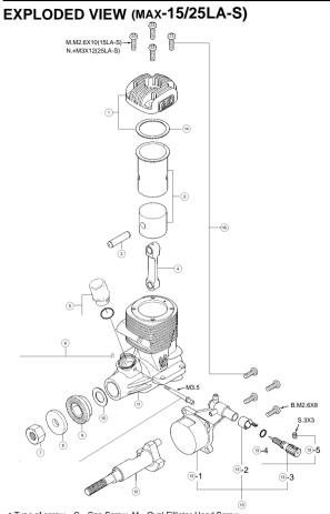
\*Type of screw C···Cap Screw M···Oval Fillister-Head Screw F···Flat Head Screw N···Round Head Screw S···Set Screw
