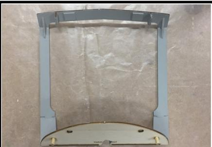
46. Glue the 5mm hatch retaining dowels in place.
