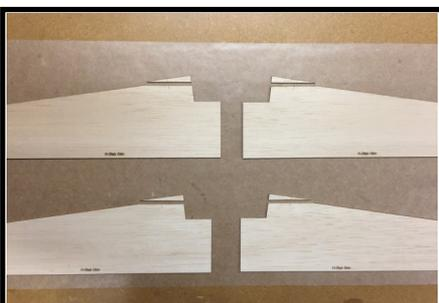
8. Remove the H-Stab Skins from the laser-cut sheets, including the little triangles; glue the little triangles in place on the leading edges of the H-Stab Skins.
