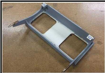
54. Assemble and install the servo cover magnet holders, one inside each front corner of the servo covers. Take care with magnet polarities to make sure they match the magnets in the fuselage floor.
