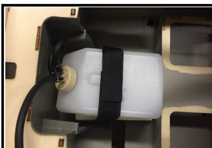
10. Assemble and install the fuel tank with a hook-and-loop strap and a piece of 1/2" (12mm) latex foam rubber as insulation against vibration (fuel tank and strap not included). Drill pass-through holes in the engine separator bulkhead for the fuel lines, offset from center if using a rear-carb engine such as the DLE-20.
