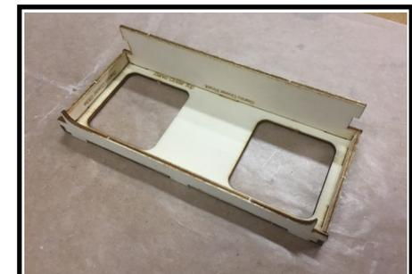
53. Build the servo covers inverted on the work table. Glue the sides first, then the front and back, and finish with the legs. Pay attention to the etched labels, whether you want them visible or not.
