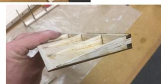
23. Place the elevator on the edge of your work bench. Using a sanding block, sand a bevel on the inside surface of the bottom Elevator Skins to match the ribs. The trailing edge of the sheeting needs to be about 1/2 the thickness of the sheeting or 1/32" at the trailing edge.
