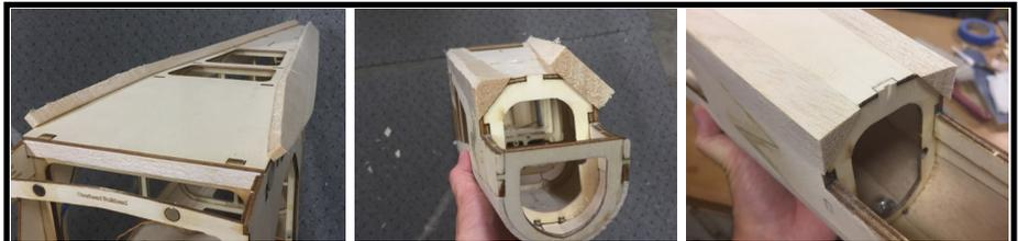
42. Glue the 10mm x 45mm sheets in place on the corners, then carve & sand to the proper radius. You may want to pre-trim some material away over the cabin area to reduce the amount of carving required.
