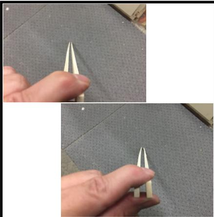
10. Inspect the spars for bow. Select, pair, and mark the spars so the bow of the upper and lower spars counteracts each other, meaning either the concave or the convex sides face each other. This step ensures the spars do not make the wing bow over time.
