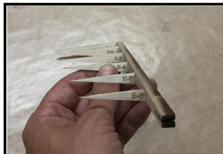
19. Using a sanding block, lightly sand the top and bottom of the LE to match the taper of the ribs
