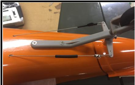
26. Flip the fuselage upside-down and slide a 1" length (25mm) of heat shrink tubing and a crimp onto each cable. Run the cables through the outermost holes in the control horn, back through the crimps, and then looped again through the crimps.
