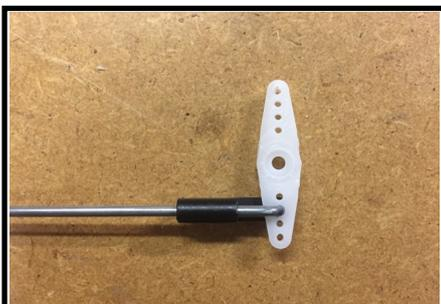
5. Remove the pushrod, bend at the mark, install onto the servo arm using a snap connector and cut to length.
