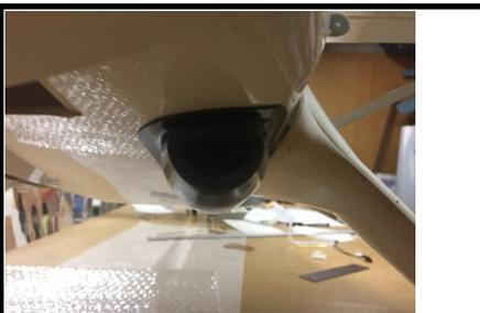
39. Install the oil cooler using either double-sided tape or medium CA. Refer to the plans for positioning.
