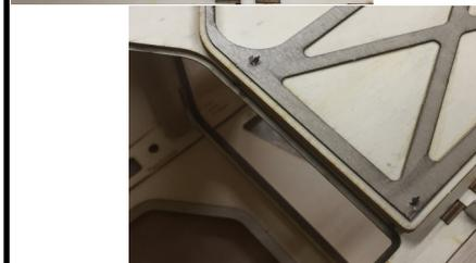
59. Hinge the doors using the small round hinges. The lower hinge should be about 1/4" (6mm) from the bottom edge, and the upper hinge should be in line with the bottom edge of the window cutout. Do not glue at this time.
