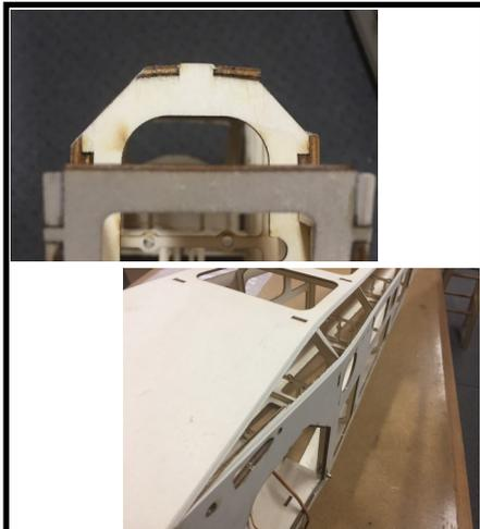
41. Sand an angle in the top and sides to match the angle in the top corners of the bulkheads.
