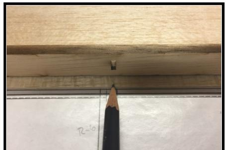
6. Again using the laser-cut trailing edge, mark the center location of the cap strips on the leading edge and trailing edge sheeting.
