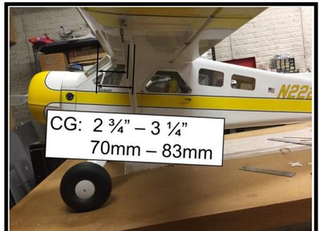
42. Assemble the airplane completely and check cg. CG has been tested between 2 3/4" and 3 1/4" (70mm - 83mm) aft of the leading edge, measured outboard of the taper at the root LE. This equates to 28% - 33% of MAC. CG is easiest to measure at the flap servo cover.
