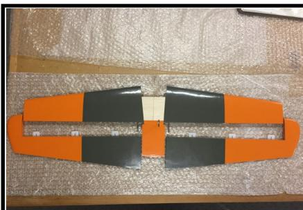
43. Hinge the elevators to the stab using the supplied CA hinges. Glue into the elevators first, then use epoxy to glue to the elevator joiner. Be sure to keep the elevators aligned, and use a wax paper barrier to prevent gluing the elevator joiner to the stab. Finally, glue the CA hinges into the stab.
