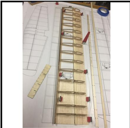
19. Glue all ribs from R-2 outboard into place from the spar to the trailing edge. Use the Ply Shear Web as a tool to keep ribs R-2 – R-5 aligned properly.
