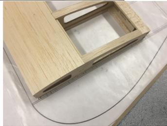
40. Trim and sand the upper and lower leading edge sheeting flush with the Sub LE. Also sand the sheeting flush with the root and tip ribs at this time.
