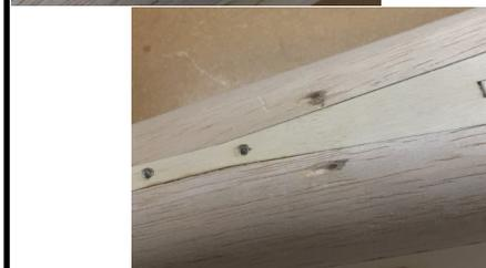
62. Install the 3mm cable guide tubes, poking them through the holes and gluing with medium or thick CA. Trim and sand flush with the outside surface, then trim to length on the forward end about 3/4" (20mm) forward of Bulkhead 4.
