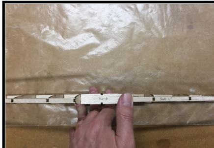
5. With the Spar/TE on the work bench and the ribs facing up, look down on the stab and check for any twist. If the stab is twisted, hold a corrective twist in place while gluing each HS-2a to the Stab Doubler.
