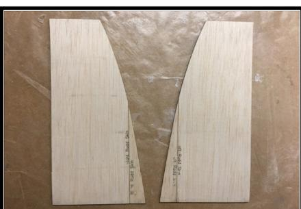
29. Remove the rudder skins from the 1.5mm balsa laser cut sheets.
