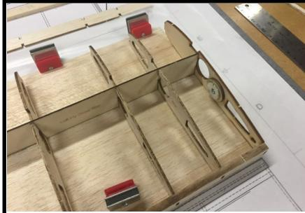
20. Glue the Ply Shear Web in place against the aft edge of the bottom spar.
