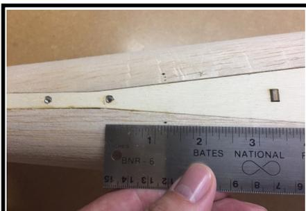
61. Drill two 1/8" (3mm) exit holes for the tail wheel steering cable guide tubes on the bottom of the fuselage, approximately 1 1/4" (30mm) forward of the front tail wheel mounting hole and straddling the tail wheel mounting doubler. The holes should go through the balsa and not the plywood.
