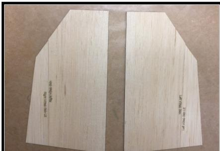
9. Remove the vertical stab skins from the 1.5mm laser cut sheets.
