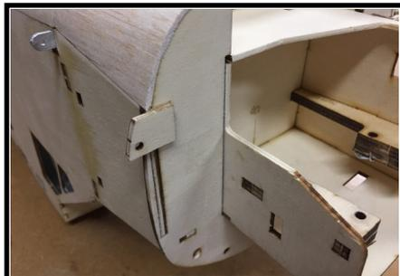
67. Glue the fuselage-mounted cowl mounting tabs to Bulkhead 1 in the location shown by the etch marks.
