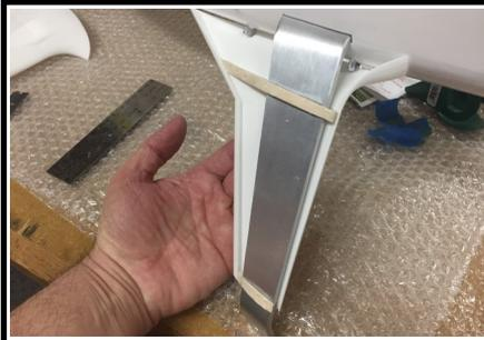
33. Slide the upper and lower LG Ribs onto the landing gear and tape in place. The lower LG Rib should be right at the end of the fairing and the upper Rib should be as shown in the photos. Exact placement is not required.
