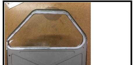
29. Trim the windows to about 1/8" (3mm) wide and glue in place in the fuselage and doors using Pacer Formula 560. Scrap balsa sticks can be used to help hold them in place while the glue dries.
