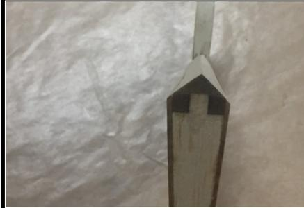
37. Carve & sand the bevel on the rudder leading edge.
