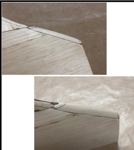
22. Sand leading edge and Dorsal Spine LE pieces to shape. Refer to the plans to aid in achieving the right profile. Any gaps can be filled with filler before covering.
