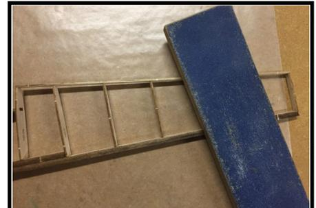
7. Using a sanding block, gently sand a bevel in the Spar/TE and the Sub LE to match the airfoil.
