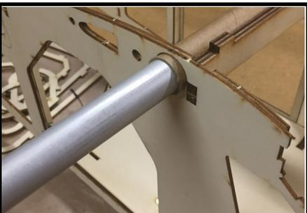
31. Install the wing tube sleeve. It should be flush to the fuselage sides on both sides.
