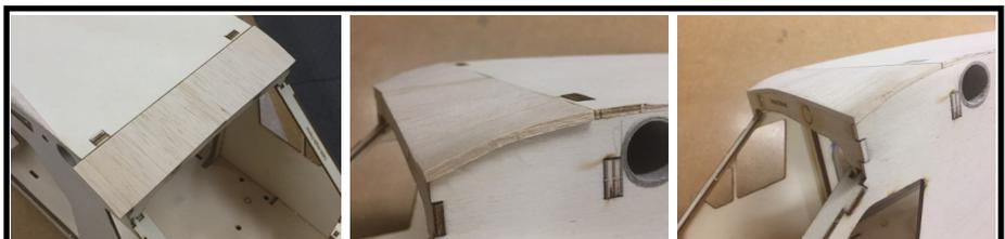
44. Glue the forward cabin roof in place, made from the 3mm x 100mm x 100mm balsa sheet
