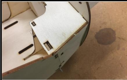
28. Install Bulkhead 1, etched label forward. Note the fuselage sides insert into the long tabs on either side of the bulkhead.
