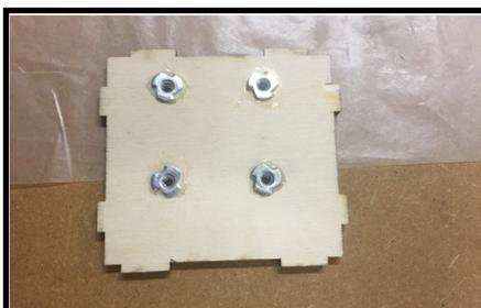
15. Install the 4mm blind nuts on the back side of the firewall, the side without etching. Glue the blind nuts in place with epoxy. NOTE: The holes provided in the firewall are for an E-flite Power 60 X-mount. If using a different motor, different holes may need to be drilled. The center location of the motor is etched on the front of the firewall to aid in properly locating the motor. Both right and down thrust are accounted for in that location.
