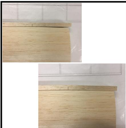
43. Glue the leading edge in place against the Sub LE and the upper and lower sheeting. The relief cut from the previous step goes inside against the Sub LE at rib R-3. Glue the outboard section first, then bend the inboard section into place. Trim and sand the ends flush with the root and tip ribs.
