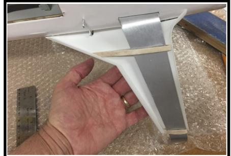
34. Fit the lower half of the gear fairings in place and note where the LG Ribs need to be trimmed and sanded for a proper fit. Also note the lower fairing will need to be trimmed to clear the float mounts. The fairings were designed to have about 1/16" (1.5mm) clearance from the fuselage. (The photos show 3D printed prototype fairings, but the included fiberglass fairings fit the same)
