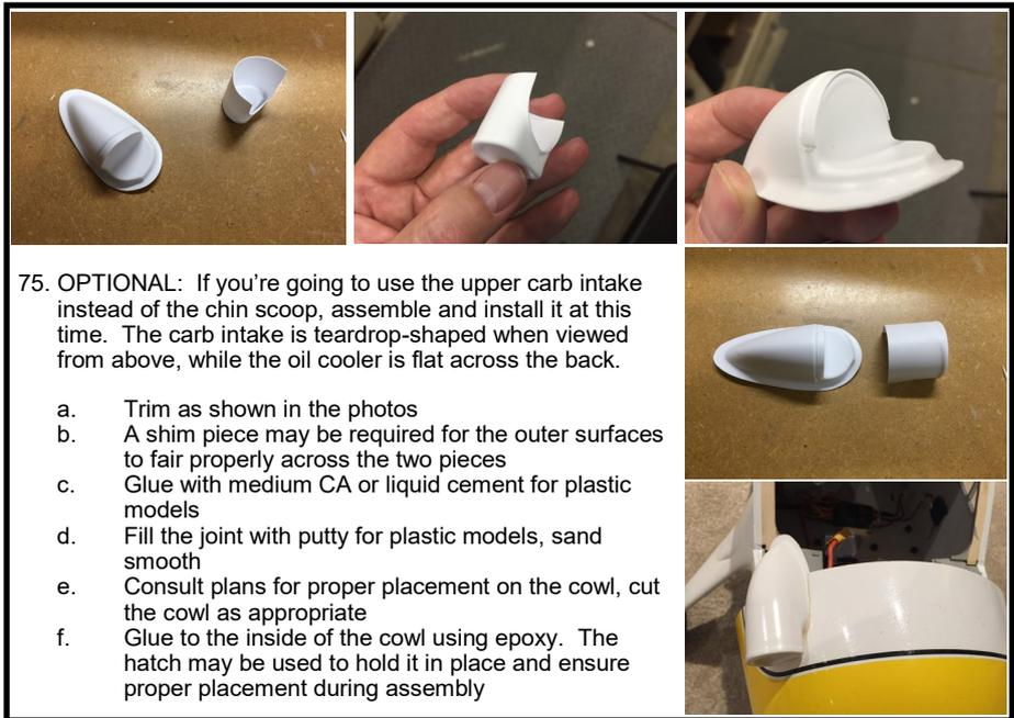
75. OPTIONAL: If you're going to use the upper carb intake instead of the chin scoop, assemble and install it at this time. The carb intake is teardrop-shaped when viewed from above, while the oil cooler is flat across the back.
