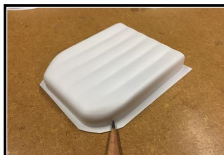
11. Rough-cut the seat parts leaving about a 1/4" (6mm) flange.
