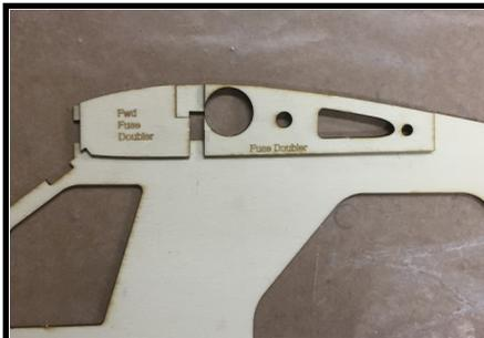
12. Glue the Fuse Doublers and Fwd Fuse Doublers into place on the fuselage sides. Use Bulkhead 3 to help get them properly positioned.
