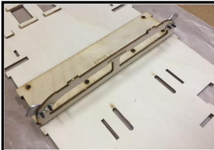
9. Glue Bulkhead 2.5 to the floor and the landing gear mount. Make sure the float mounts are on the aft side of the bulkhead!
