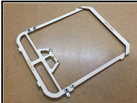
1. Remove the bulkheads from the 3mm lite ply sheets. Use a hobby knife to cut through the joining tabs holding the parts in the sheets. Also remove Bulkhead 3 from the 6mm ply sheet.
