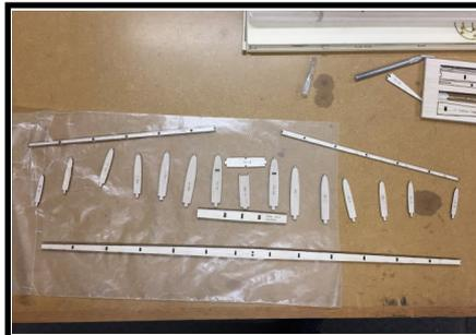
1. Remove all the horizontal tail parts from the laser-cut sheets
