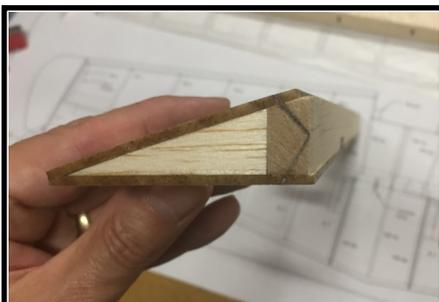
9. Mark a centerline down the leading edge of the aileron, then mark a bevel on each end to serve as a guide for carving and sanding the required bevel into the leading edge. It can also help to draw spanwise lines on the top and bottom of the aileron back from the leading edge to guide how far back to carve and sand.
