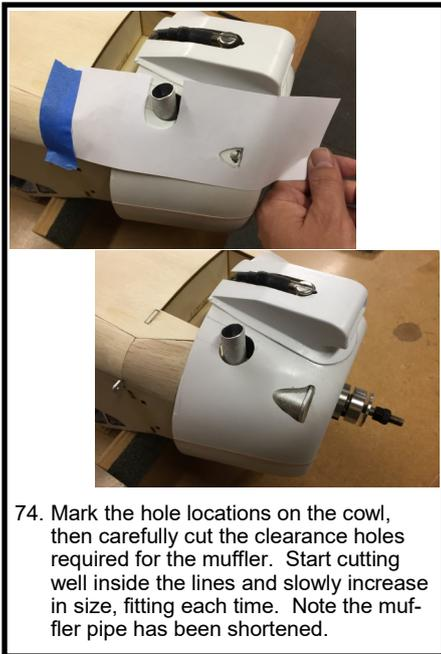
74. Mark the hole locations on the cowl, then carefully cut the clearance holes required for the muffler. Start cutting well inside the lines and slowly increase in size, fitting each time. Note the muffler pipe has been shortened.
