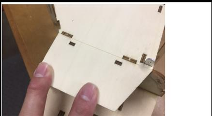
27. Bend the sides inward and glue to the Motor Box Top. You will hear a slight cracking of the wood as it bends.
