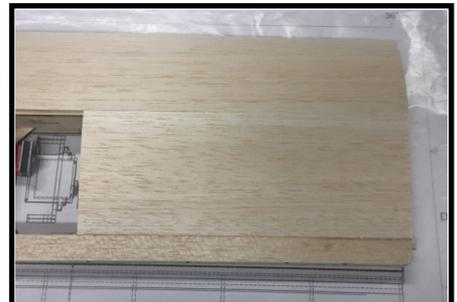
38. Cut another 9 3/4" (248mm) section from the 2.5mm x 4" x 48" sheet for the center section upper sheeting (root end of the wing). Carefully trim & sand to width to fit into place between the LE and TE sheeting, then glue into place.
