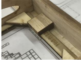
31. Glue the flap hinge support blocks in place (6mm laser-cut balsa). See plans for locations. For the middle block, you may want to cut a notch out as for a rabbet joint so the block will fit over the hatch liner.
