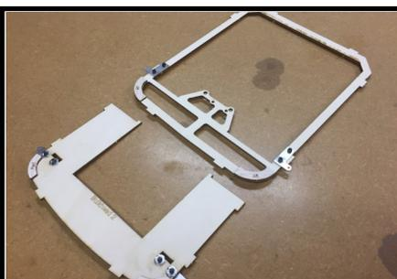
5. Glue the 2.5mm balsa sheeting helpers to the aft side of Bulkhead 4 (labeled "AFT") and the forward side of Bulkhead 2 (labeled "FWD").
