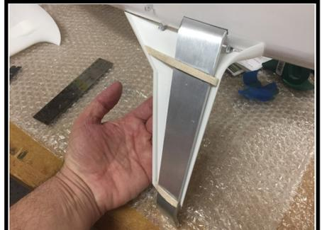
37. Glue the fairing lower half in place using a mixture of epoxy and microballoons applied to the LG Ribs.
