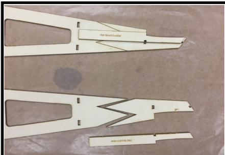
11. Glue the aft fuselage tips onto the ends of the fuselage sides, followed by the Stab Mount Doublers.
