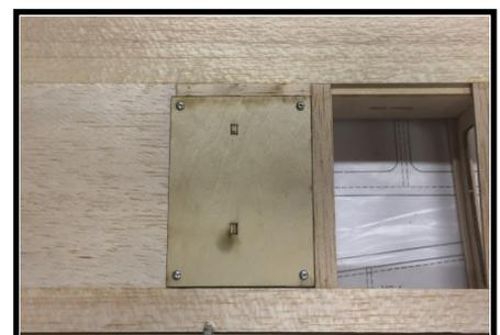
55. Mount the hatches using 2mm x 10mm button head screws.
