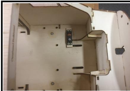
55. Install the throttle servo. Etch marks have been provided on the floor for one possible location showing both mini servo and standard servo sizes. The unused flap and aileron servo mount doublers can be used as doublers for mounting the throttle servo.
