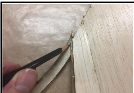
13. Fit the 1mm ply Dorsal Spine in place and mark the thickness of D-1 along the edge on both sides.
