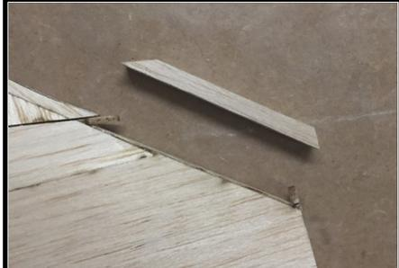
20. Sand the ends of the Vertical Stab leading edge to fit between the tabs on VS-6 and VS-7. NOTE: the tabs on VS-6 and VS-7 are used to serve as guides when sanding the leading edge to shape.
