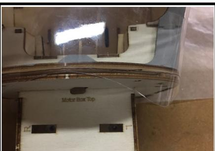
49. Put the windshield back in place, mark and trim the forward trim line about halfway between the hatch bulkhead and the fuselage Bulkhead 1. This will be a rough cut which will be trimmed closer in a later step.
