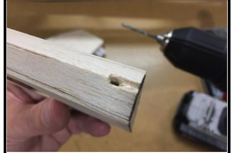
38. Drill a 1/8" hole (3mm) for the rudder torque rod, 5/16" (8mm) from the bottom of the rudder. Cut a groove from that hole to the root to allow the torque rod to nest into the rudder leading edge. Cut or file a radius between the hole and the groove to get a better fit.
