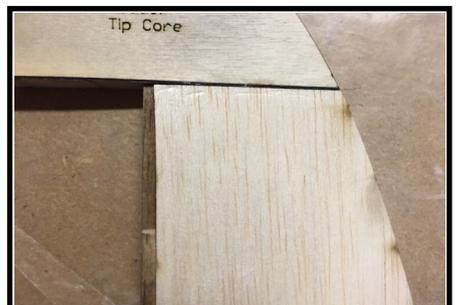
31. Glue one side of the rudder skin in place. Use the tip plywood rib as a guide; match the trailing edge of the skin to the trailing edge of the tip core. Note the leading edge of the skin is not straight: the leading edge of the skin at the tip will rest about 1/8" aft of the edge of the 2nd Leading Edge, while the lower front corner of the skin falls about 1/4" aft of the same edge. (see photos in next box)
