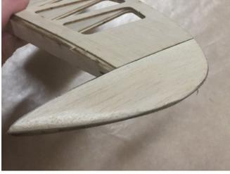
36. Carve and sand the tips to shape. Note the tip radius transitions to a flat trailing edge where the tip cores meet the skins at the trailing edge.
