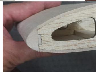
44. Carve and sand the leading edge to shape as shown on the plans. We find it easiest to do this in two steps. First, carve & sand the top and bottom of the LE to an angle that's tangent to the top and bottom sheeting. Second, sand to the final shape. The Tip Mounting Rib can be used to trace the proper outline onto the ends of the leading edge to help achieve the proper shape.
