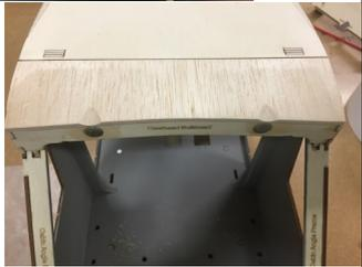
64. Using a bit of medium/coarse sandpaper wrapped around the wing tube, sand a small divot in the roof of the cabin just above each hatch magnet. These divots will provide grip points for hatch removal.
