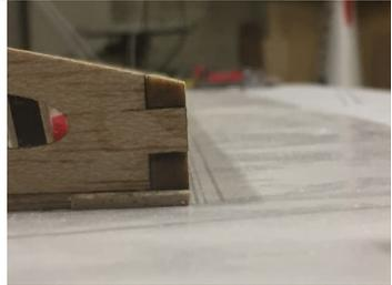
35. Use a sanding block to sand the trailing edge and the Sub LE flush with the upper contour of the ribs so the upper sheeting will glue properly in place.
