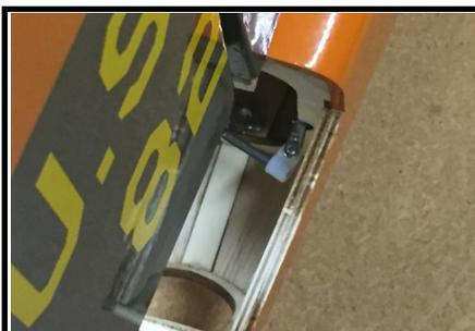
7. Glue the vertical stab & rudder to the fuselage before installing the horizontal stab. First install a 3mm nut on the rudder pushrod and adjust the clevis by turning in or out to center the rudder with the servo centered. Once satisfied, tighten the nut, connect the pushrod to the rudder and glue the vertical stab into place using epoxy. Site from front and rear to assure vertical alignment.
