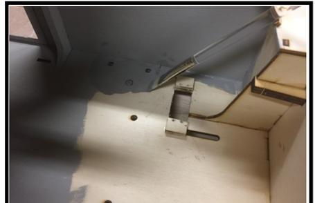
60. Paint the interior of the fuselage back to bulkhead 5 an appropriate color for your scheme. A light/medium gray acrylic craft paint was used in the prototypes.
