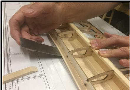
34. Glue the lower leading edge sheeting to the ribs and the Sub LE. To do this, slide a thin, strong, and flexible item like a steel rule under the sheeting. While holding the wing flat to the table with one hand, bend the sheeting upward to meet the ribs & Sub LE with the steel rule. Use medium or thick CA and glue one rib at a time, working your way down the wing. You may want to start in the middle and work toward each end.
