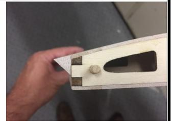
50. Sand the upper surface of the triangle stock to match the curvature of the upper surface of the wing. You may want to use masking tape to protect the wing while rough sanding.
