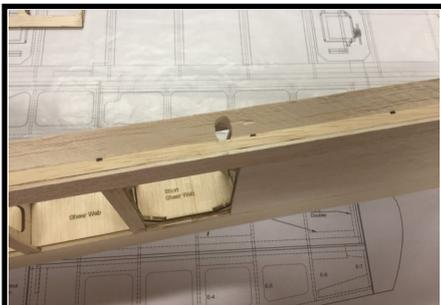
51. Drill and file the hole for the flap pushrod into the triangle stock.
