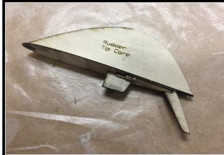
25. Assemble R-6 and the plywood rib to the Rudder Tip Core.
