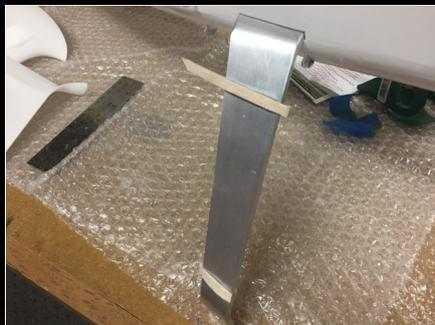
36. Once satisfied with the fit of the LG Ribs and fairings, glue the ribs in place on the gear using medium CA.
