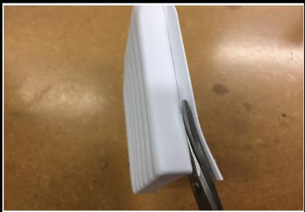
13. Cut the seat parts to these lines using body scissors. If necessary, clean up the edges using a fine sanding block.
