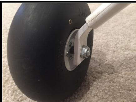
40. After painting the LG fairings and main gear, install the landing gear axle shafts to the aluminum main gear using the included lock nut.
