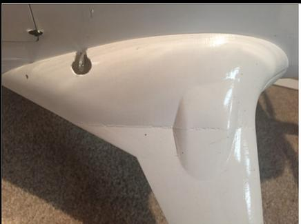
35. Fit the upper half of the fairing in place. Cut a clearance slot to provide access to the fuselage strut mount.
