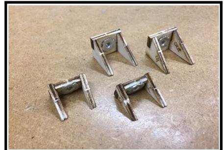
66. Assemble the cowl mounting tabs that will glue to the inside of the cowl. Install 4-40 blind nuts on the back sides using epoxy.
