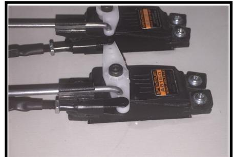
25. Cut the openings in the covering for the tail wheel steering cables where they exit the fuselage, then install the cables from the front. Attach the clevises to the outermost holes on the rudder servo arm.
