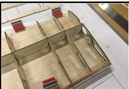
17. Before gluing the ribs in place, perform a dry assembly of the ribs, upper spar, Sub LE, Ply Shear Web, and wing tube sleeve to familiarize yourself with how everything fits together. Points to note:
