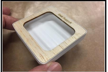
18. Glue the 2.5mm balsa seat supports into the seat bottoms using medium CA, flush with the bottom edges.
