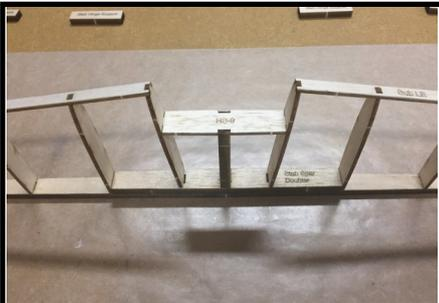
4. Assemble both HS-2as onto the stab, as well as HS-9 and both Sub LEs
