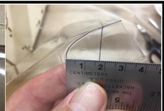
48. Carefully trim the windshield to fit the hatch. A pair of curved "body scissors," sold by brands such as Dynamite and Duratrax, make this task much easier. Take it slowly to achieve a proper fit.
