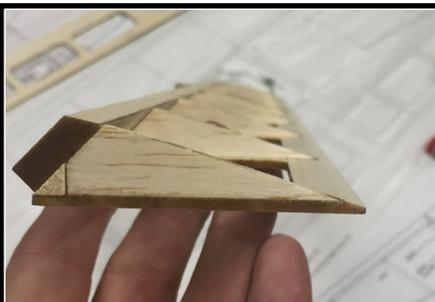
9. Sand the leading edge and trailing edge to match the contour of the ribs. Note that the upper surface of the flap has a slight contour – the upper surface is not flat.
