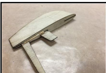
20. Glue E-8 and E-7 onto the Stab Tip Cores
