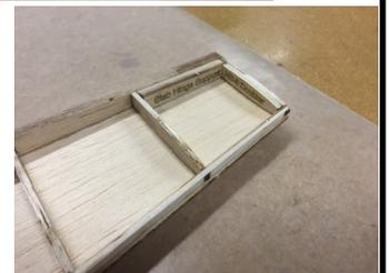
10. Glue in the hinge reinforcement blocks, as well as the HS-8 Doublers (3mm lite-ply).
