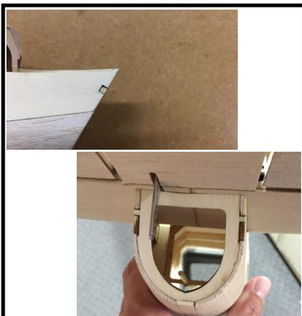
43. Sand the top of the Canted Bulkhead flush with the fuselage sides at the stab saddle, then sand a slight "V" shape in the same location (when viewed from behind) so the horizontal stabilizer mates properly to the fuselage.
