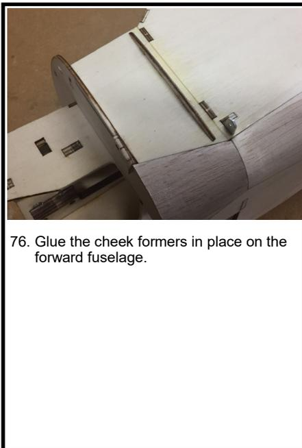
76. Glue the cheek formers in place on the forward fuselage.
