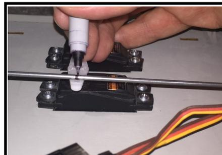
4. Assemble a clevis onto the rudder pushrod and slide the pushrod through the guide tube. Attach the clevis to the rudder and set the vertical stab & rudder in place on the fuselage. With the rudder centered, mark the pushrod for bending at the servo arm.
