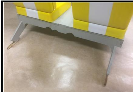
28. Once the tail wheel cables are installed, sand and/or file the back of the aft servo cover to provide clearance for the pushrod and cable linkages.
