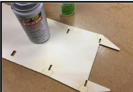
32. Flip the fuselage upside-down to install the Fuselage Bottom. Apply a small shot of CA accelerator to the circled locations of the bottom sheet before assembly to help the CA "grab" as the sheeting is wrapped around the slightly curved Bulkheads 2.5 and 2.
