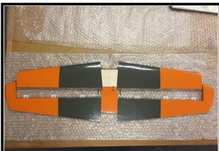
41. Cover the stab and elevators with your favorite iron-on film covering. Leave the bottom side of the stab center section uncovered for gluing into place on the fuselage.
