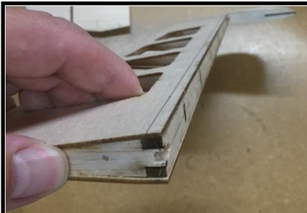
37. Mark a line down the center of the elevator leading edges. This is easier with a simple hinge marking tool like the Great Planes GPMR4005.
