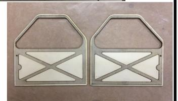
13. Glue the 1mm ply door frames in place on the fuselage sides.
