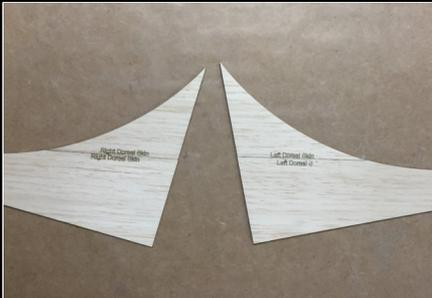
17. Remove the Dorsal Skins from the 1.5mm laser-cut sheets and assemble the same way as the vertical stab skins, matching the edges with text labels for both left and right skins.
