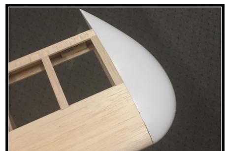
47. Glue the wingtip in place using medium or thick CA if you're confident with your positioning skills, or epoxy if you're not.
