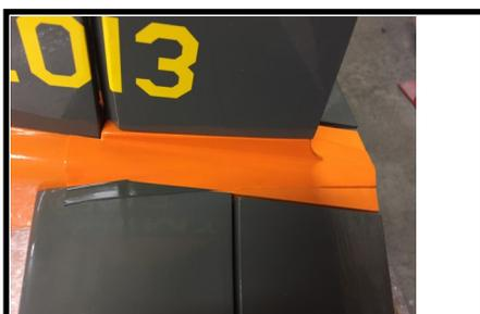
9. Install the rudder fairing and the tail cone using double-sided tape.
