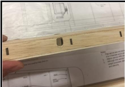
48. Cut a hole in the trailing edge for the flap pushrod. This hole needs to be about 1/4" – 5/16" (6-8mm) wide and about 3/8" (9-10mm) tall, located almost to the upper trailing edge sheeting. See plans for spanwise location; on the left wing the hole is centered 10" (254mm) from the root, and on the right wing it's centered 11 3/4" (298mm) from the root. You may want to wait until the flaps are finished before completing this step.
