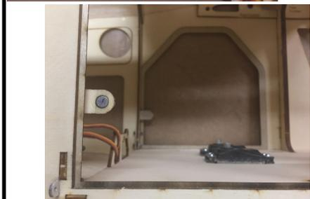
58. Using the doors as a guide, glue the fuselage door magnet holders in place.
