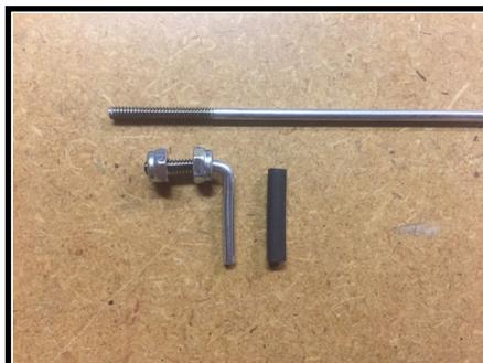
30. Make the door handles using 3mm pushrods and lock nuts. The handle length is about 3/4" (18-19mm). Bend the pushrod about 1/8" (3mm) from the threads, as the pushrod will break if you try to bend it exactly at the end of the threads. Cover the handle with a length of black heat shrink tubing.
