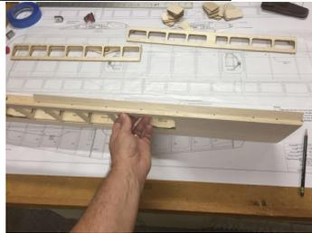
49. Cut a length of the 1/2" (13mm) triangle stock to 21 5/8" (549mm) and glue in place on the trailing edge of the wing.
