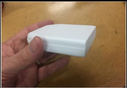
16. Glue the front and back halves together, overlapping the front part over the back about 1/16" (1.5mm). Medium CA can be used, but liquid cement for plastic models provides a little more time for positioning.
