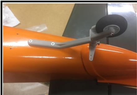
23. Attach the tail wheel assembly to the bottom of the fuselage using 3mm flat-head screws.
