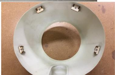
70. (Continued) Fill any remaining gaps between the mounting tabs and the cowl with epoxy and milled fiber.
