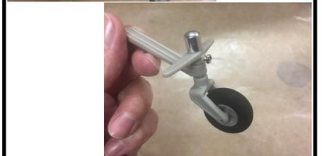
21. File a small flat on the tail wheel shaft to provide a seating surface for the control arm set screw.
