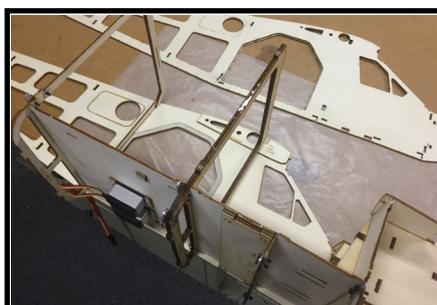
21. Glue Bulkheads 3 and 4 in place on the floor. Use a square to keep them approximately perpendicular to the floor.
