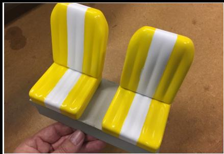
17. If you're planning to paint the seats with a pattern, as we did in our first prototype, you may want to paint them now, before gluing the seat backs to the seat bottoms. Make sure to mask off the contact area between them for a good glue joint.
