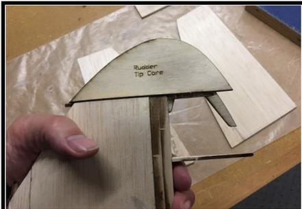
27. Using the vertical stabilizer as a guide, now glue the tip assembly to the rudder leading edges. Be careful not to glue the rudder to the vertical stabilizer.
