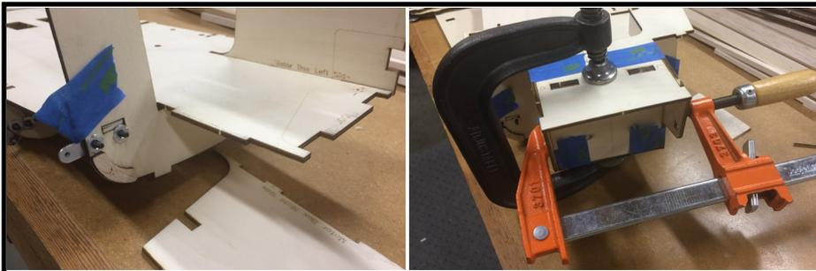
17. Place the firewall and the motor box top in place to get comfortable with how it fits together.
