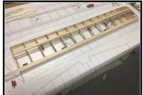
36. Glue the trailing edge upper sheeting in place (2.5mm x 3/4" x 48"). Trim to length either before or after gluing in place.
