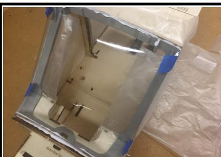
51. Remove the hatch frame and place wax paper or plastic wrap dams in place to prevent gluing the hatch permanently to the fuselage. Replace the hatch frame and glue the windshield in place using canopy glue such as Formula 560.
