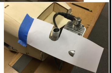
72. If using an engine, mount it to the fuse and cut a clearance slot for the spark plug cap & wire. (DLE-20 shown)
