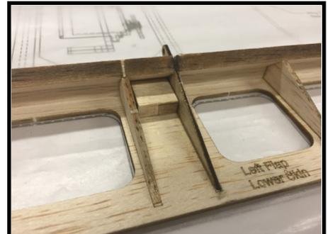
7. Fit and glue the Flap Horn into place. You will have to deepen the slot in the leading edge with a file, hobby knife, or razor saw to get a proper fit.
