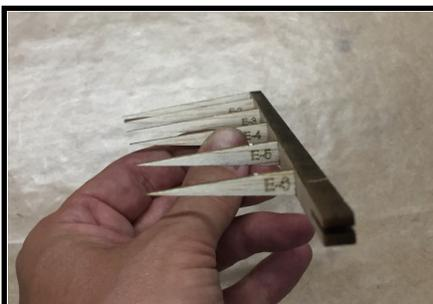
18. Glue the ribs E-1 through E-6 to the leading edges. Take care to center the ribs vertically on the LE. As you did on the horizontal stabilizer, use a scrap piece of lite-ply with a 90 degree corner to ensure the ribs are perpendicular to the LE.
