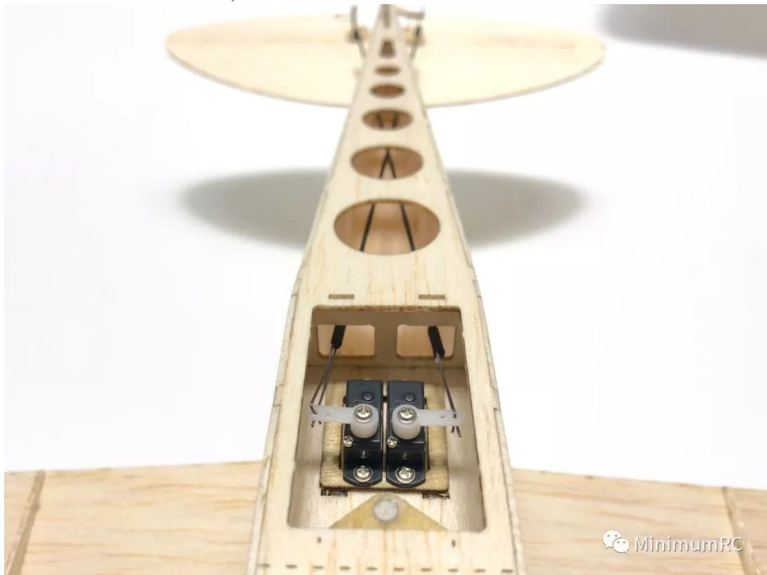
49. Installation of the pushrods.
