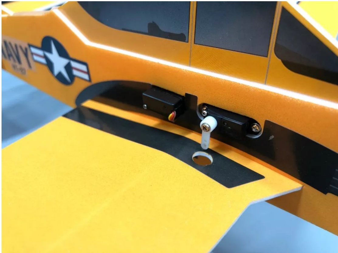
17. Installation of the servos.
