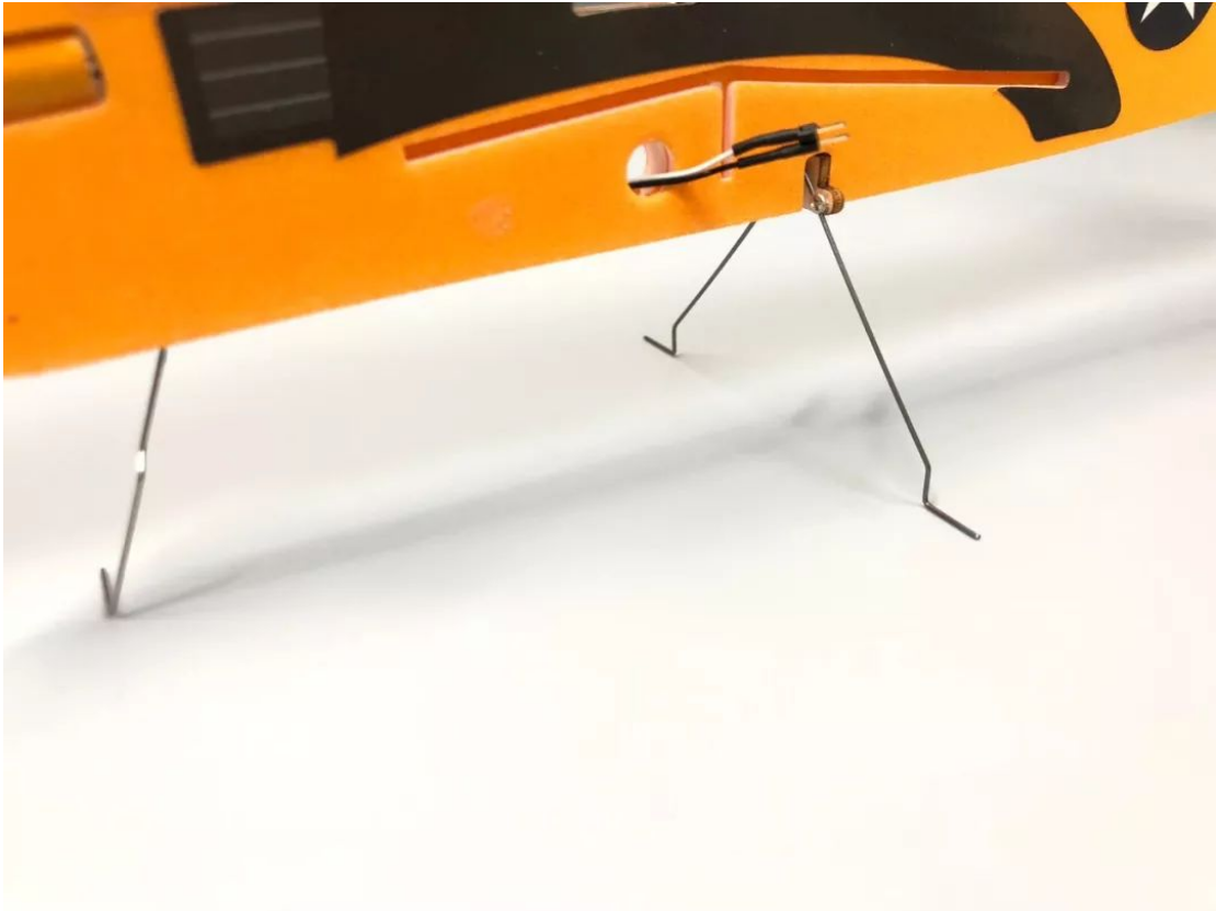
10. Installation of main landing gear base.
