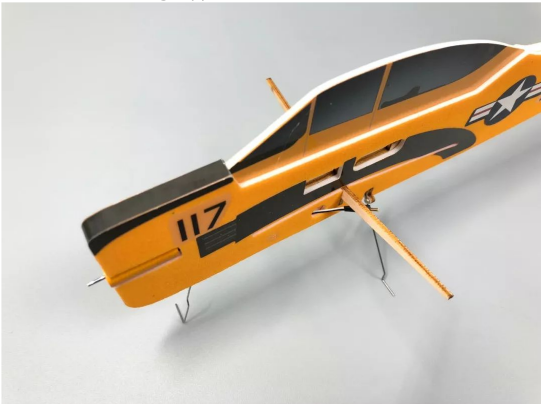
11. Installation of wing support.
