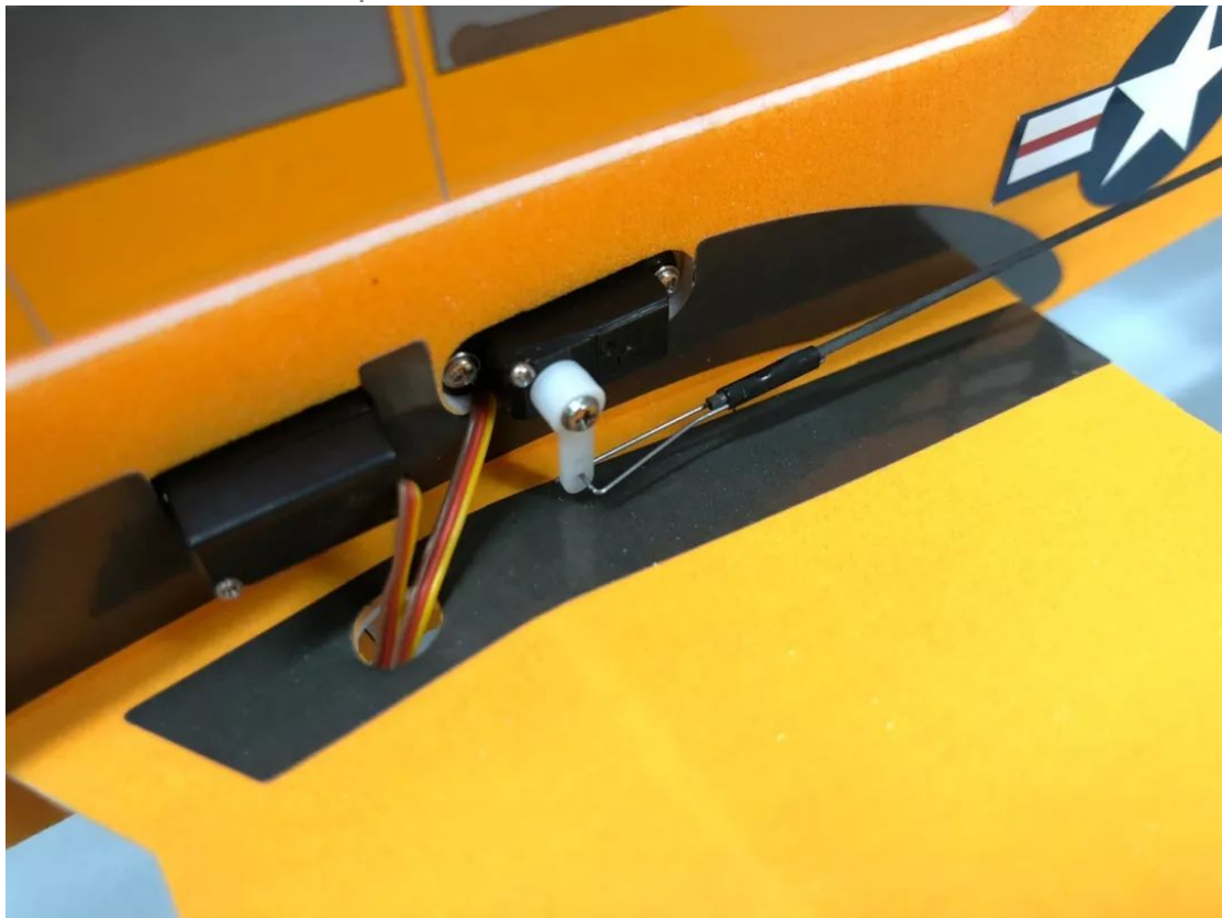
19. Installation of the pushrods.
