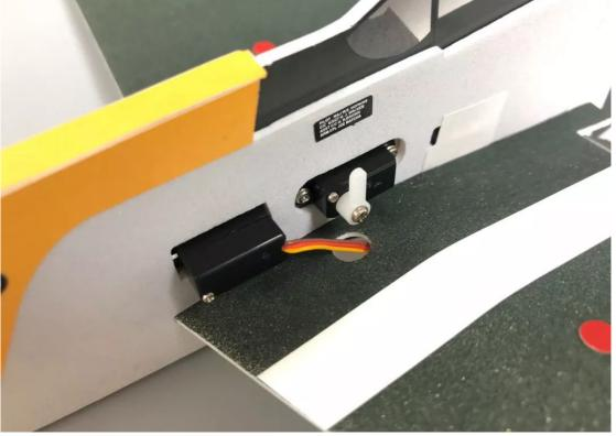
20. Connect the pushrod clips & pushrods with heat shrinkable tube and fix them with glue.
