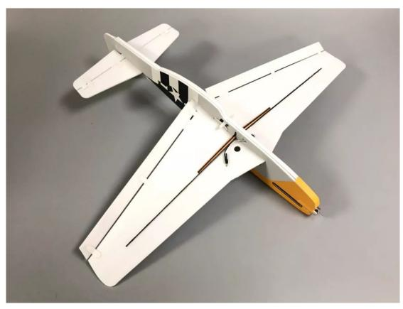
15. Reinforce the wing with  $\Phi$  1mm carbon rods.
