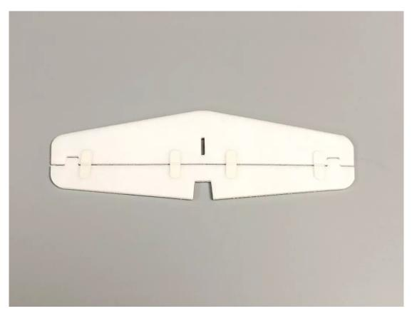
10. Install the horizontal tail, the elevator needs to move freely.
