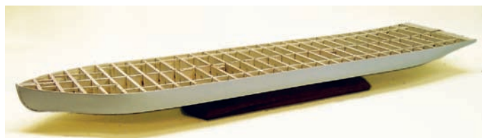
Photo 11: hull finish painted and mounted ready for the main deck
