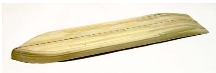
Photo 10: hull filled and sanded ready for finish
