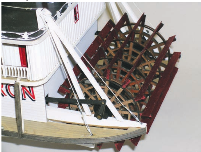
Photo 18: Paddle wheel, stern timbers, cranks and pitmans
