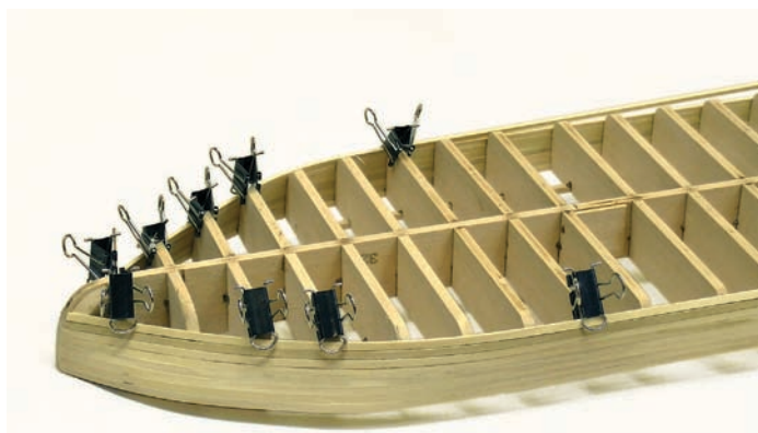
Photo 5: 8th plank being installed at bow
