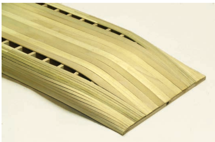
Photo 9: the bottom planking at the stern
