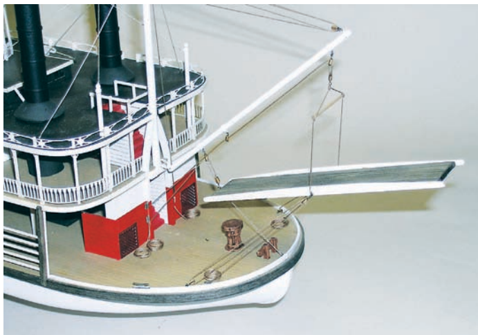
Photo 20: stage and stage boom rigging
