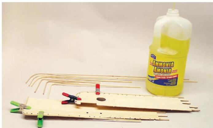
Photo 13: bending the boiler deck capstrips
