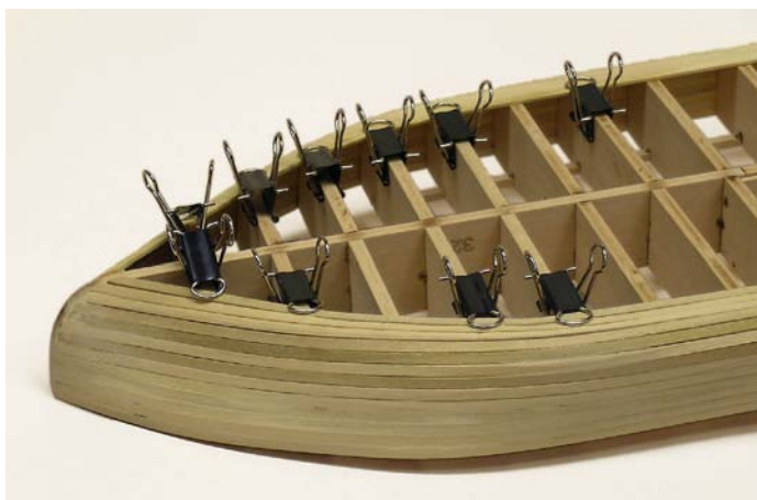
Photo 7: the 13th plank run being installed
