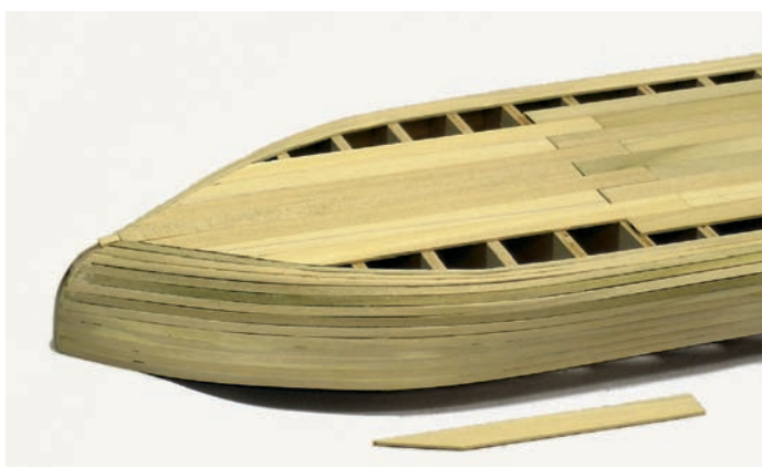
Photo 8: installation of the bottom planking. Note fairing block and staggered joints
