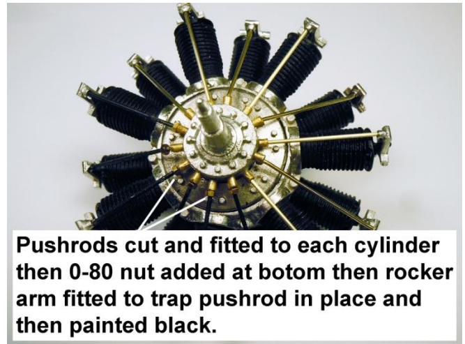
Making pushrods using 1/32" brass rod angle bent at each end, then cut to fit front and rear.
