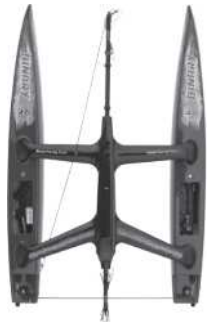
BINARY catamaran hull (Servos, receiver & battery box pre-installed)
