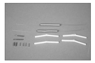
$\Box$  2. Apply a thin coat of petroleum jelly to the hinge point of each of the four hinges. This will keep epoxy from entering the hinge, which could restrict their movement.
