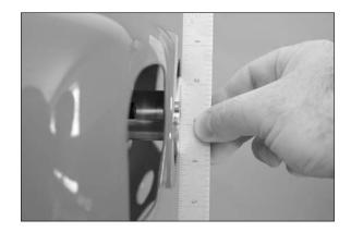
**Note**: The previous step only works when using a spinner with a flat backplate. If the backplate of your particular spinner will be recessed on the driver washer, use the backplate to set the gap between the cowl and spinner backplate.
