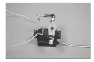
$\Box\Box$  10. Use string or dental floss to secure a 36-inch (915mm) servo extension to the rudder servo lead. Mark the lead so it can be easily identified when the servo is installed in the fuselage.
