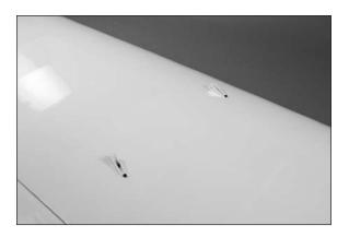
$\Box$  3. Install the threaded wing strut fitting in the wing so threads are flush to the wing surface. It will be at an angle when installed so it aligns with the strut support.
