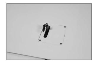
$\square$   $\square$   $\square$  20. Slide the 8-32 x 2<sup>1</sup>/<sub>4</sub>-inch countersunk machine screw into the hole in the aileron. Mix a small amount of 30-minute epoxy and apply it to the last 1/2inch (13mm) of the screw. Once the screw is in position, Use isopropyl alcohol and a paper towel to remove any excess epoxy.
