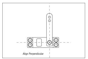
□□□□ 5. Prepare both the right and left aileron servos at this time. Note the position of the servo horn on the servos shown.
