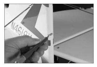
$\Box$  7. Use 30-minute epoxy to glue the hinges to the fin. Allow the epoxy to fully cure before proceeding.
