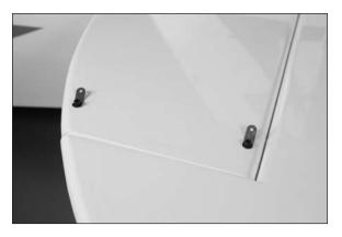
$\Box$  4. Attach the last two brass strut fittings to the bottom of the fuselage by removing the screws that hold the servo cover in position. Tighten the screws using a 3/32-hex wrench.
