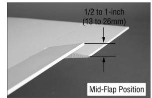
**Note**: If you are using a 2-position flap switch, still set the center position as a starting point for the flap linkage installation.
