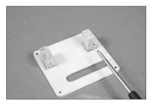
□□□□ 12. Apply 2–3 drops of thin CA in each hole to harden the surrounding wood. Allow the CA to cure before proceeding.
