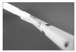
□ 4. Use a toothpick and 30-minute epoxy to glue the hinges in the rudder. Make sure to apply epoxy to both the hinges and into the holes in the rudder. Use isopropyl alcohol and a paper towel to remove any excess epoxy. Allow the epoxy to fully cure before proceeding.
