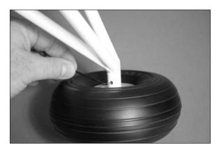
*Hint*: Place a drop of silicone adhesive on the inside edge of the hub cap if you find it is not secure when in position.
