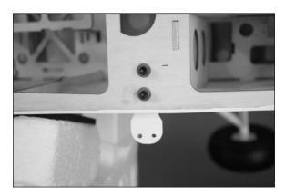
$\Box$  3. Thread a 4mm nut and a strut end on each of the struts. The final position of the ends will be adjusted once the wing is on the fuselage.
