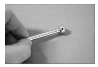
$\Box$  10. Remove the hub cap from the wheel using a small flat blade screwdriver. Place a drop of light machine oil on the axle, then slide the axle through the wheel from the side with the hub cap as shown.
