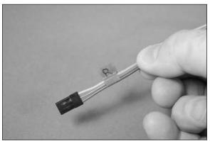
$\Box$  11. Repeat step 10 to secure a 36-inch (915mm) extension on each of the elevator servos. Again, remember to mark the leads of the servos so they can be easily identified.
