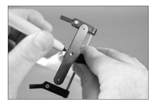
$\Box$  6. Use a pin vise and 1/16-inch (1.5mm) drill bit to drill the two holes for the tiller arm mounting screws.
