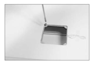
□□□□ 17. Apply 2–3 drops of thin CA in each hole to harden the surrounding wood. Allow the CA to cure before proceeding.
