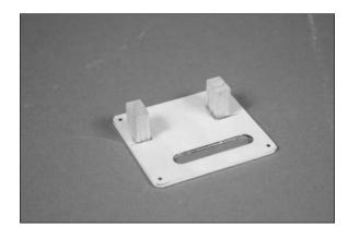
D 9. Place the servo between the blocks. Position the servo so there is a 1/32-inch (.5mm) gap between the servo and cover. Use a pencil to mark the location for the servo mounting screws on the servo mounting blocks.
