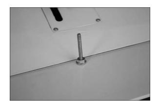
$\square$   $\square$   $\square$   $\square$  22. Thread the short control horn on the screw for the aileron until it is 1<sup>1</sup>/<sub>8</sub>-inch (29mm) from the control surface as shown. Use the short control horn for the aileron, and the long control horn for the flaps.
