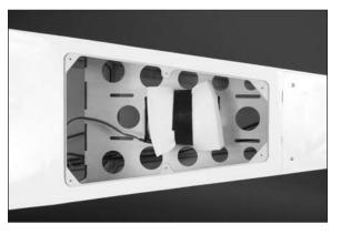
$\Box$  2. Once the receiver battery has been installed, use six 2mm x 8mm sheet metal screws and a #1 Phillips screwdriver to secure the cover over the battery compartment.
