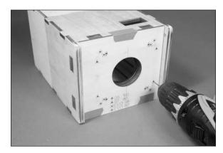
$\Box$  3. Remove the template and use a drill and 5/16-inch (8mm) drill bit to enlarge the mounting holes. You will also need to drill a hole for the fuel tubing suited to your particular engine.
