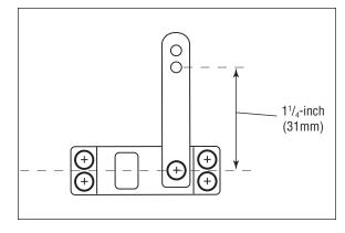
□ 3. There is a right and left stabilizer and elevator assembly. When installing them, make sure the countersunk hole for the elevator control horn screw faces toward the top of the airframe.
