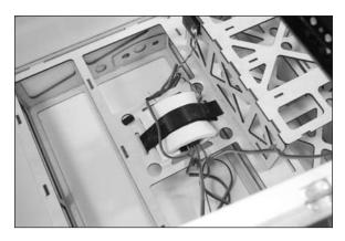
□ 3. Use hook and loop tape (not included) to mount the remote receiver as far away from the main receiver as possible. Make sure the antenna on the remote receiver is positioned vertically in comparison to the horizontal positioning of the main receiver antenna.
