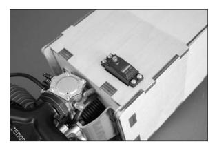
$\Box$  8. Attach the servo arm to the throttle servo. Install the two ball links and the 4-40 x  $1^{3}/_{4}$ -inch adjustable linkage. Use the radio system to check the operation of the throttle servo to make sure it operates the carburetor correctly.
