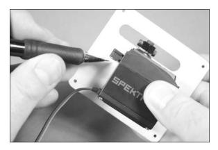
□□□□ 7. Use medium grit sandpaper to scuff the end of the servo mounting block to provide a better surface for the adhesive.
