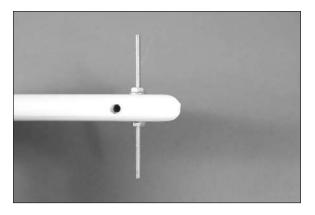
$\Box$  4. Thread a control horn on each end of the threaded rod so the measurement from the control surface to the clevis is 1<sup>1</sup>/<sub>8</sub>-inch (28mm) as shown in the drawing.
