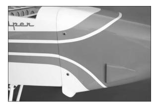
$\Box$  12. Use a straight edge on the drive washer of the engine to check the gap for the spinner. Adjust the position of the engine box in the fuselage until there is a 3/32-inch (2mm) gap between the straight edge and cowl as shown.
