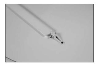
$\Box$  5. Attach short wing strut to front fitting with 4-40 x 5/8-inch socket head cap screw and 4-40 lock nut. Use 1/4-inch nut driver and 3/32-inch hex wrench to tighten hardware. Make sure the airfoil on strut matches wing, and jury strut fitting faces to wing.
