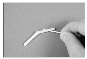
$\Box$  5. Thread a cable fitting into each of the ball ends. To make sure the fitting is secure, turn the fitting 12 rotations in the ball end.
