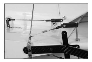
$\Box$  9. Use the smaller brass crimps to secure the tail wheel springs to the rudder tiller arm and the tail wheel arm. Use crimping pliers to secure the crimps in position.
