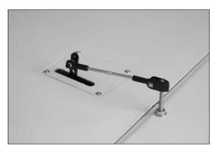
$\Box$  25. Use a 4-40 x 2-inch adjustable link for the flap servo installation. Adjust the linkage to achieve the mid-flap position as shown. The servo horn can be angled toward the leading edge to achieve mechanical differential.
