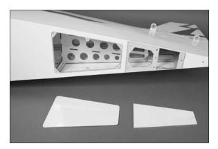
$\Box$  13. Installing the screws for the servos can be difficult. Use a small piece of fuel tubing to hold the servo mounting screw on a #1 Phillips screwdriver so it can be installed in the fuselage.
