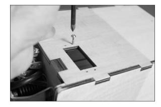
$\Box$  6. Place 2–3 drops of thin CA in each hole to harden the surrounding wood.
