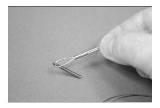
□□ 5. Loop the cable back through the crimp. This will make the cable secure when it is crimped in the next step.
