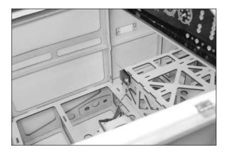
$\Box$  4. Use a hobby knife with a #11 blade to remove the covering from the fuselage for the switch harness. Mount the harness using the hardware provided with the harness.
