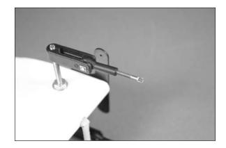
$\Box$  6. Test fit the rudder to the fin. Trim the holes as necessary to fit the rudder tightly to the fin.
