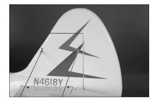
$\square$  8. Use brass crimps to secure the cable to the cable fittings. Make sure the radio system is on and the rudder servo centered before using crimping pliers to secure the crimps to the cable.
