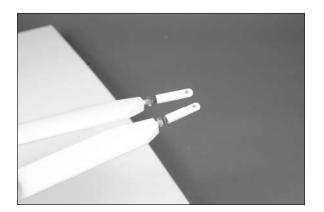
$\Box$  4. Slide the aluminum wing joiner into the pocket in the wing. Slide the joiner in only as far as it will easily slide, as forcing it could cause damage to the wing. Note the joiner faces up toward the top of the wing.
