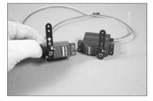
□□□□ 6. Place the servo on the cover, centering the servo arm in the opening. Use a pencil to mark the location of the servo mounting tabs.
