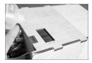
$\Box$  7. Install the grommets and brass eyelets in the throttle servo. Secure the servo using a #1 Phillips screwdriver and the hardware included with the servo. Make sure to prepare and harden the holes as described through the earlier sections of the manual for servo installation.
