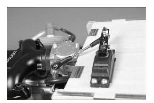
$\Box$  9. Slide the engine mount box into the fuselage as shown.
