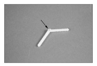
$\Box$  3. Place the hinges in the rudder. When positioned to full throw, they will be perpendicular to the hinge line. They also will be inserted so the hinge point is aligned with the hinge line of the rudder. Use a hobby knife and #11 blade to trim the rudder as necessary to fit the hinges.
