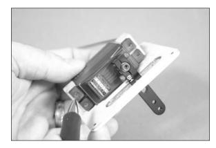
$\Box$   $\Box$   $\Box$   $\Box$   $\Box$  10. Use a 5/64-inch (2mm) drill bit to drill the four holes for the servo mounting screws.
