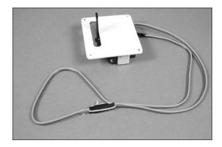
**Note**: Use a 3-inch (152mm) servo extension when preparing the flap servos for installation.
