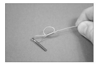
$\Box$  6. Pull the slack cable taut. Use a crimping tool to secure the cable and crimp in position.
