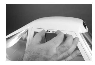
$\Box$  2. Use foam rubber and a hook and loop strap to secure the receiver in the fuselage. Make sure to plug the servos into the correct ports of the receiver, as well as the 12-inch (305mm) extensions into the aileron and flap ports of the receiver.
