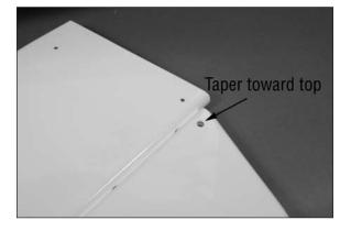
$\Box$  4. Slide the aluminum tubes for the stabilizer into the stabilizer. Note the longer tube is closer to the elevator as shown in the photo below.
