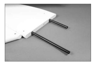
$\Box$  5. Slide the stabilizer assembly into the slot at the rear of the fuselage.
