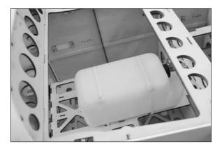
**Note**: We use a Fuel Filler with a "T" Fitting and Overflow Fitting (HAN116) to allow fueling of the model without the necessity of removing the cowl.
