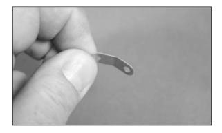
$\Box$  3. Use six 4-40 x 1-inch socket head cap screws, six 4-40 lock nuts and twelve #4 washers to attach the brass strut fittings to the fin and stabilizer. The larger hole is used to attach the strut fitting, while the smaller hole is used to attach the clevises. Tighten the hardware using a 3/32-inch hex wrench and 1/4-inch open-end wrench.
