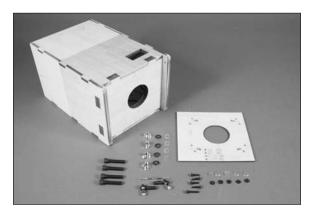
$\Box$  2. Tape the plywood template to the front of the engine mount box. Make sure the top of the template faces the side of the box with the opening for the throttle servo. Use a drill and 1/16-inch (1.5mm) drill bit to drill the holes for your particular engine.
