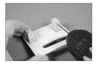
□□□□ 11. Use a #1 Phillips screwdriver to thread a servo mounting screw into each of the holes to cut threads in the surrounding wood. Remove the screw before proceeding to the next step.
