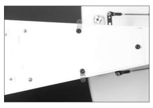
$\Box$  5. Thread a 4-40 nut on each of the threaded rods. After sliding a silicone clevis retainer on each of the clevises, thread the clevis on the rod until the end of the rod can be seen between the forks of the clevis. Make sure to set aside the two longer 4-40 x 11<sup>7</sup>/<sub>8</sub>-inch threaded rods so they can be installed in the correct location on your model.
