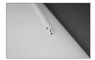
$\Box\Box$  6. Slide safety tubing onto the strut pin. Prepare three pins at this time.
