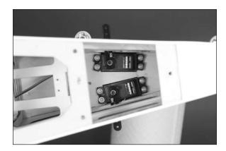
□ 17. Mount the rudder servo in the fuselage using a #1 Phillips screwdriver and the screws supplied with the servo. Make sure the servo lead falls through the fuselage toward the cockpit. Note the position of the rudder servo in the fuselage. Guide the cables for the rudder through the openings in the sides of the fuselage. Note that the cables cross inside the fuselage.
