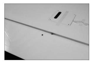
A Remove the aileron servo cover from the wing. Remove the cover for the flap servo at this time as well. Make sure to mark the covers so they can be placed back into the wing in the correct locations.
