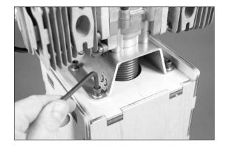
$\Box$  5. Thread the servo mounting screw into the holes for the throttle servo. Remove the screw before proceeding to the next step.
