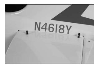
$\Box$  7. Slide the remaining stabilizer into position. Start the screws that secure the stabilizer. Once all the screws have been started, use a 1/8-inch hex wrench to fully tighten the screws, securing the stabilizer to the fuselage.
