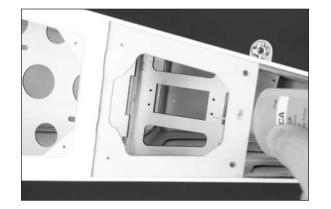
□ 16. Mount the elevator servos in the fuselage using a #1 Phillips screwdriver and the screws supplied with the servos. The servos arms can then be installed through the side of the fuselage. Access the pinch bolts on the servo horns by using the radio to move the servo arms 45-degrees to gain access through the slot in the fuselage. Make sure the servo leads fall through the fuselage toward the cockpit. Note the position of the servos in the fuselage.
