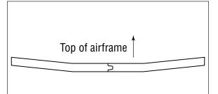
$\Box$  5. Slide the wing into position on the fuselage. Make sure to guide any wiring from the wing into the fuselage so the wing panel will rest tightly against the fuselage. Use two 1/4-20 x 2-inch nylon wing bolts to secure the wing to the fuselage.
