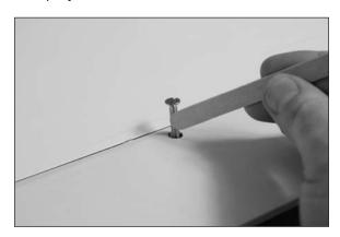
□□□□ 21. Apply a drop of threadlock on the screw near the aileron surface. Use an 11/32-inch open-end wrench to tighten the 8-32 flanged nut against the wing to secure the position of the screw.
