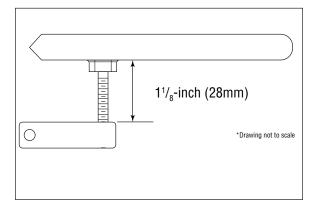
$\Box$  4. Install the 4-40 x 4<sup>1</sup>/<sub>2</sub>-inch adjustable link between the control horn and ball end. With the servo centered, adjust the link so the elevator is aligned with the stabilizer.
