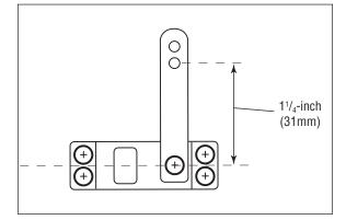
$\square$  16. Use a #1 Phillips screwdriver to thread a 2mm x 10mm wood screw into each of the holes to cut threads in the surrounding wood. Remove the screw before proceeding to the next step.
