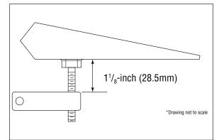
□□□ 23. Repeat Steps 2 through 22 to install the remaining aileron servos, as well as the flap servos.
