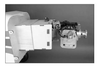
$\Box$  10. Prepare the five cowl mounting screws using five tapered washers, five foam disks, four 4-40 x 1/2-inch button head screws and one 4-40 x 3/4-inch button head screw. Note that the tapered washers will have the cone facing out toward the head of the screw.
