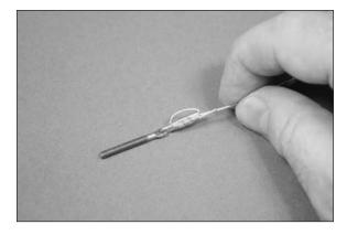
$\Box$  7. Thread the cable fitting in the ball end. To make sure the fitting is secure, turn the fitting 12 rotations in the ball end.
