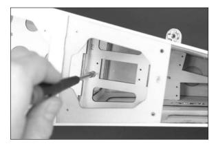
$\Box$  15. Place 2–3 drops of thin CA in each hole to harden the surrounding wood.
