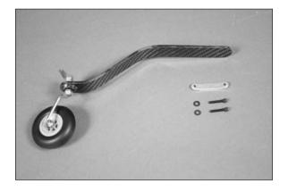
**Note**: Always use threadlock on metal-to-metal fasteners to prevent them from vibrating loose.
