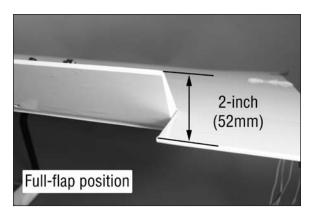
$\Box$  27. Set the flap switch to the up flap position. Use the travel adjustment to move the servo so the flap is aligned with the wing as shown.
