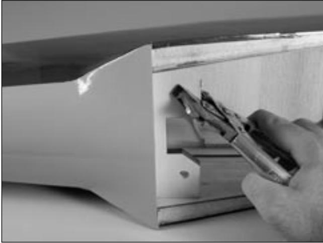
**Note:** Make sure no epoxy gets into the threads of the blind nut.
