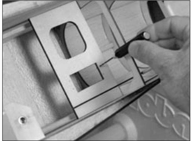
**Hint:** Place a drop of thin CA onto each screw hole to harden the wood around the hole. Allow the CA to fully cure before installing the servos.
