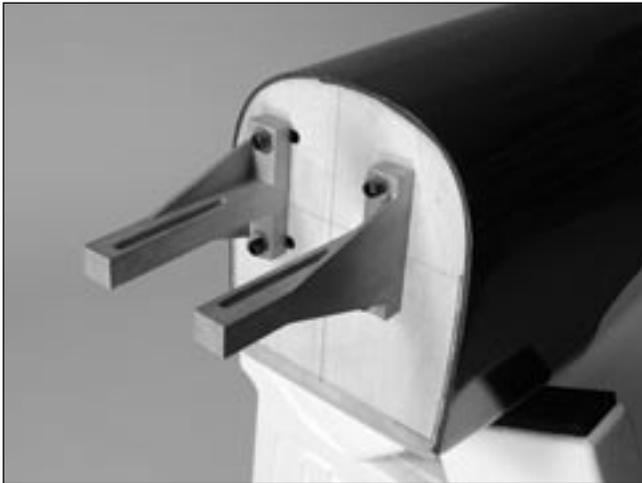
**Hint:** You can also install the blind nuts backwards to prevent them from pulling into the wood on the backside of the firewall. Just remember to move them to their correct positioning before moving to the next section.
