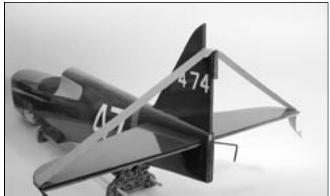
**Note:** Check the alignment of the fin periodically to make sure it isn't moving while the epoxy cures.
