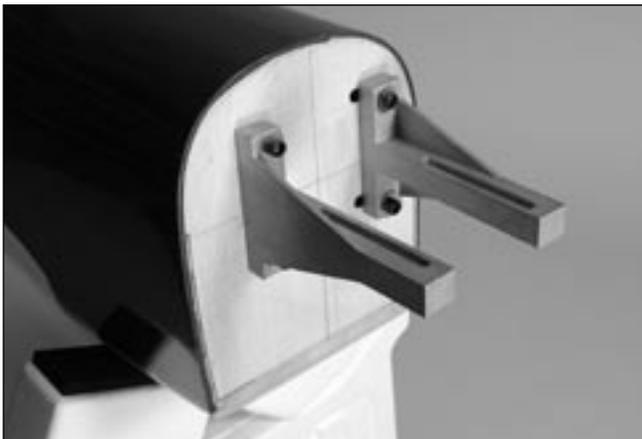
**Hint:** You can also install the blind nuts backwards to prevent them from pulling into the wood on the backside of the firewall. Just remember to move them to their correct positioning before moving to the next section.
