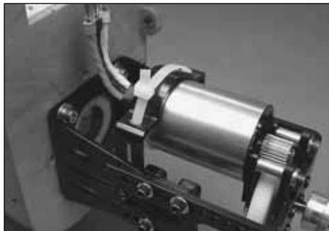
The Large Motor Mount comes with an optional Motor Bracket. If you have installed a 40mm or longer motor in the Motor Mount; we recommend installing the optional Motor Bracket. Attach the Motor Bracket to the sides of the Motor Mount using two 4-40x1/2" SHC screws, #4 flat washers and 4-40 lock nuts. Position the Motor bracket as far back on the motor as possible. Once the Motor Bracket is installed, secure the motor to the Motor Bracket using the nylon strap.
