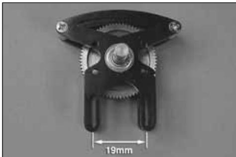
The ElectriFly Ammo motors have high kVs meaning that they like to run at very high rpm. A gear drive is used in order to reduce the rpm allowing a larger, more efficient propeller to be used. Great Planes ElectriFly offers a **36mm Large Gear Drive (GPMQ0515)** with several pinions that allow for the following gear ratios:
