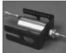
In-runner motors that will be run direct drive or gear drive and are mounted inside the front plate.
