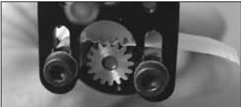
Loosely mount the motor to the back of the back plate with two 3x23mm SHC screws and two 3mm flat washers. Place a piece of notebook paper between the pinion gear and the spur gear. Squeeze the two gears together while
