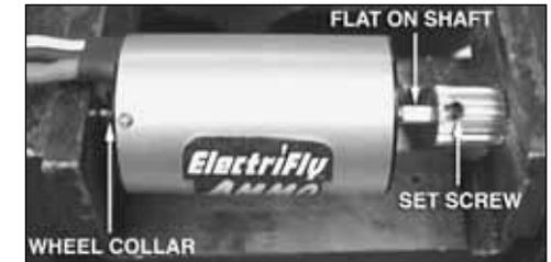
If you do not have a drill press a small vise can also be used. Place the motor between the jaws of the vise with the end of the motor shaft supported and the pinion gear centered on the motor shaft. Heat the pinion gear and slowly close the jaws of the vise. You may need to use a second wheel collar so that the pinion gear can be pressed on past the end of the motor shaft.
