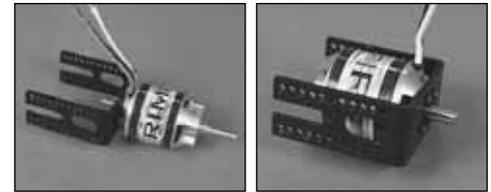
Out-runner motors can be mounted inside the Front Plate in some situations using four 3x8mm SHC screws, but most of the time they will be mounted on the front of the Front Plate.
