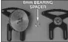
To remove the spur gear, loosen and remove the two 2.5x17mm flat head machine screws and 5.5mm aluminum spacers. Remove the backplate, being careful to not lose the 6mm bearing spacer.
