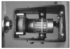
The 28mm Motor Mount comes with an optional Motor Bracket. If you have installed a 45mm or longer motor in the Motor Mount we recommend installing the optional Motor Bracket. Attach the Motor Bracket to the sides of the Motor Mount using two 4-40x1/2" SHC screws, #4 flat washers and 4-40 lock nuts. Position the Motor bracket as far back on the motor as possible. Once the Motor Bracket is installed, secure the motor to the Motor Bracket using the nylon strap.
