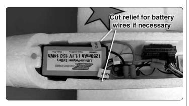
☐ 11. Apply a piece of the included self-adhesive hook and loop material to the battery tray and a mating piece to your flight battery. Test fit the battery onto the battery tray. The exact position of the battery on the tray will be determined when you balance the plane. Depending on the battery you have
