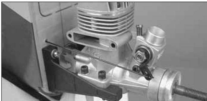
14. Cut off the excess pushrod tube 1/2" [13mm] behind the third fuse former.
