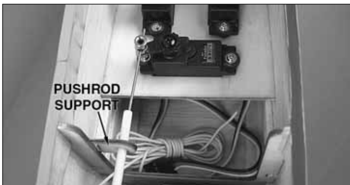
15. Install the .039" x 13-3/4" [1mm x 350mm] throttle pushrod with Z-bend into the outer pushrod and connect the Z-bend to your engine throttle arm (you may need to remove the arm from the carburetor to do this). Install a screw-lock pushrod connector into the outer hole of the throttle servo arm and test fit it onto the servo. A pushrod support is provided and can be glued to the former just in front of the throttle servo. You may need to sand or cut this part to length depending on the pushrod position. When satisfied, slide the support onto the pushrod tube and glue it in place. Tighten the aft end of the throttle pushrod in the screw-lock pushrod connector (do not cut off the excess length of pushrod until you have used your radio system to center the servo and have made your adjustments to the pushrod length).
