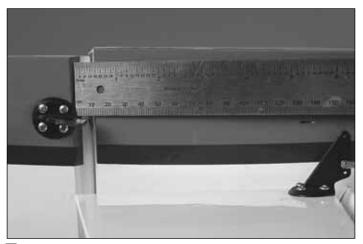
☐ 15. Use a ruler to position the control horns on each side of the rudder. Align the holes in the control horn with the hinge line. Drill 1/16" [1.6 mm] pilot holes in the rudder at the screw mounting locations. Attach the rudder control horns using four #4 x 1/2" [13 mm] sheet metal screws on each control horn. Remove the screws and harden the screw holes with some thin CA. Allow the glue to fully harden before permanently installing the mounting screws.
