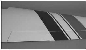
☐ 7. Fit the hinges in the wing and aileron. Tape the aileron to the wing and set aside until the epoxy has cured.
