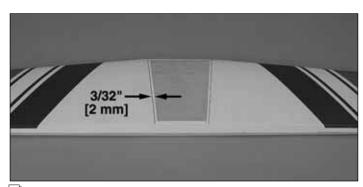
☐ 6. Remove the covering from the center section of the stab 3/32" [2 mm] inside the marked line, being careful not to cut into the wood structure.
