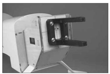
☐ 5. Mount the engine mount to the firewall as shown using four 8-32 x 1-1/4" [32 mm] SHCS, #8 flat washers and #8 lock washers.
