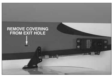
☐ 13. Remove the covering from the two teardrop shaped pull-pull cable exits at the rear of the fuselage.
