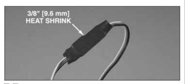
□ □ 1. Connect a 12" [305 mm] servo extension to the aileron servo and secure the connections with heat shrink tubing or some other method such as tape or clamps designed to hold servos together (not included).
