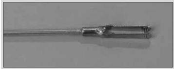
☐ E. This is what a properly soldered clevis looks like; shiny solder with good flow, no blobs, flux removed.
