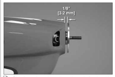
■ 5. Slide the cowl over the engine and onto the fuselage. Use a Dremel tool with a cutting bit to trim the cowl if necessary so you can get it to fit over the engine. Mount the spinner back plate to the engine. Position the cowl so that there is a 1/8" [3.2 mm] gap between the cowl and the spinner back plate.
