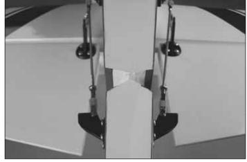
☐ 5. Use the same procedure as done with the elevator halves to create pushrods and align the control horns. Final installation will resemble the picture above.
