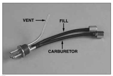
□ 3. Attach gasoline safe fuel line with clunks to the tubing as shown; remember to bend the vent line upwards towards the top of the fuel tank. The clunks should move freely. One clunk is for the fill line and one is for the carburetor line.
