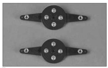
10. Install two screw lock connectors into the third hole on each side of the servo arm extension as shown.
