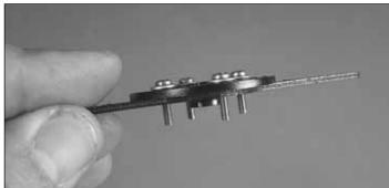
☐ 7. Use four 2-56 x 3/8" [9.5 mm] machine screws and #2 washers to attach the extender to the wheel as shown. Be sure to add a drop of threadlocker to the screws.
