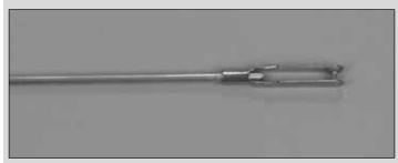
☐ B. Apply a few drops of soldering flux to the end of the pushrod. Position the clevis so that 1/8" of the pushrod protrudes into the open area of the clevis.
