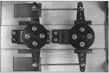
☐ 12. Locate the two 5-1/4" [133 mm] 4-40 pushrod segments. Cut each pushrod to 4" [102 mm]. Then insert the two pushrods through the screw lock connectors on both rudder servo arms. Lock the pushrods in place using 4-40 x 1/8" [3.2 mm] SHCS. Add a drop of Threadlocker to each screw to hold in place.
