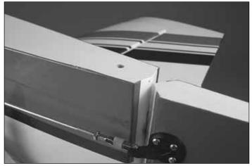
■ 8. Locate the small cutout on the tail of the fuselage for the tail gear bearing. Remove the covering using a sharp hobby knife.
