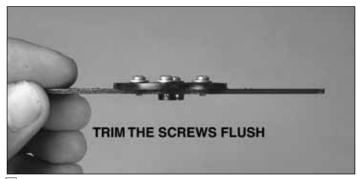
■ 8. Trim the 2-56 screws flush with the bottom of the extender using a rotary tool such as a Dremel, or a pair of heavy-duty wire cutters.
