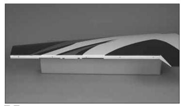
1. Cut the covering away from the five predrilled holes in the left **aileron** and left **wing panel**.
