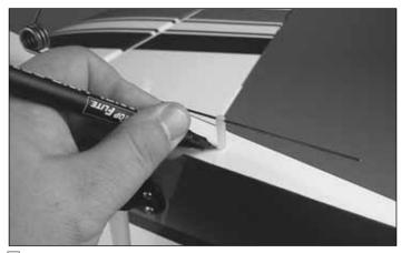
☐ 12. Slide the nylon rudder post onto the tail gear as shown. Move the post to the approximate midpoint of the gear wire. Be sure the rudder is centered and mark the location that the rudder post touches the rudder. Drill a 5/32" [4 mm] hole at this mark.
