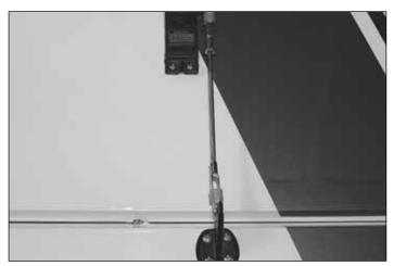
☐ 7. Reattach the pushrod assembly as shown. Be sure to slide the silicone retainers over the clevises.
