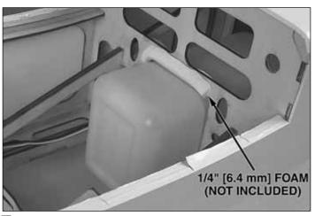
☐ 3. Cut two small strips of 1/4" [6.4 mm] foam (not included) approximately 1/2" [13 mm] wide. Insert these strips between the fuel tank and the former. Glue them in place using CA. Begin with the bottom piece of foam. You may need to temporarily remove the tank to glue in the bottom foam.
