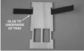
☐ 3. Overlap 2" of the hook and loop sides of the tape and press together. Loop around the plywood radio tray as shown.
