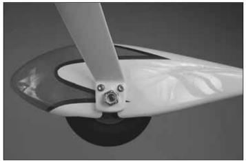
□ 5. Slide the **fiberglass wheel pant** over the main wheel and align the holes in the main gear with the holes in the wheel pant. Using two 4-40 x 1/2" [13 mm] SHCS, #4 lock washers and #4 washers, attach the wheel pant to the gear leg. Add a drop of Threadlocker to each 4-40 SHCS. Note the direction of the gear leg in relation to the pant in the photo.
