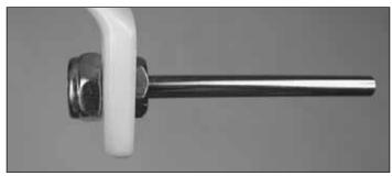
☐ 1. Attach one 3/16" [4.8 mm] x 2" [51 mm] axle to a main gear strut. Use a 5/16" [8 mm] nylon lock nut on the back side of the axle as shown.
