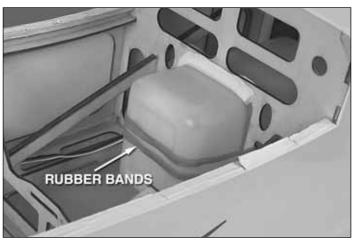
4. Secure the tank using the supplied rubber bands.
