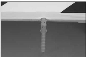
□ 2. Locate five **point hinges**. Test fit each hinge by temporarily attaching the aileron to the wing. Note the "wings" on each hinge near the pivot. These are designed to align the hinge and prevent it from rotating. It will take a small amount of force to push these wings into the wood.
