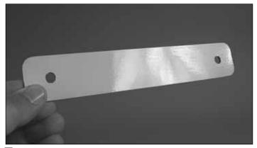
7. Locate the **wing bolt plate**. Remove the covering from the holes in the plate using a sharp hobby knife.
