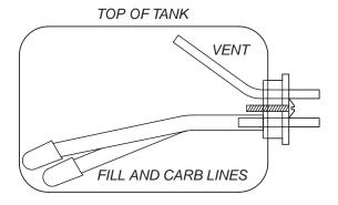
1. Insert the stopper and check the length of the fuel line and fill lines. The clunks should rest almost against the back of the tank when the stopper is in place but move freely inside the tank. Adjust the length of the fuel line until the proper length has been reached. Once you are satisfied with the fit, secure the stopper using the Phillips head screw in the stopper assembly. Be careful not to over tighten the stopper.
