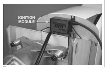
6. Mount the electronic ignition unit as shown.
