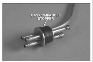
☐ 2. Assemble the stopper using Du-Bro #813 1/8" [3.2 mm] I.D. fuel line barbs (DUBQ0670) and 1/8" [3.2 mm] brass tubing as shown. Solder the barbs to the brass tubing but be careful not to overheat the assembly as it could cause damage to the rubber stopper.
