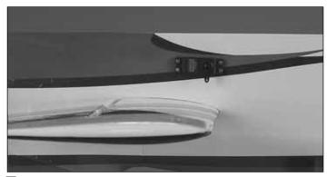
☐ 11. Route the servo lead through the fuselage and install the servo with the output spline toward the nose of the plane as shown. Center the servo by temporarily connecting it to the radio system and attach a servo arm. Remove the servo mounting screws and harden the holes for the servos with thin CA. Allow the CA to fully dry before reinstalling the screws.
