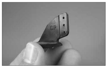
☐ 14. Trim the two rudder control horns as shown. This is necessary to allow the elevator halves to clear the horns.
