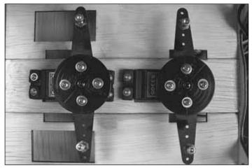
☐ 11. Attach both servo arms to the servo, ensuring they are perfectly parallel.
