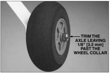
□ 4. Reinstall the wheel collars and main wheel. Apply a small amount of thread locking compound to the wheel collar set screws and tighten them in place. Trim off the excess axle, leaving 1/8" [3.2 mm] extending past the wheel collar. A rotary tool and cut off disc or flat file works best for this.
