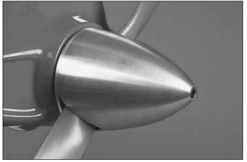
☐ 3. Mount the spinner cone to the back plate using one of the supplied spinner bolts
