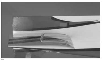
■ 9. Locate the two elevator servo bays in the rear of the fuselage, one on each side of the fuselage. Remove the covering from these bays using a sharp hobby knife. Note there are two cutouts on each side that can accommodate a servo. Cut the covering from the servo bays closest to the top of the fuselage, nearest the stab.
