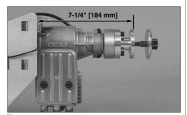
☐ 5. Mount the engine to the firewall so that the distance from the firewall to the drive washer is 7-1/4" [184 mm].
