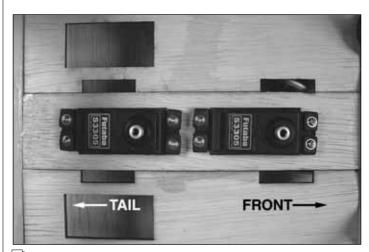
☐ 2. Install two rudder servos in the servo tray as shown using the hardware provided by your manufacturer. Be sure each servo's output shaft is pointed towards the front of the fuselage.
