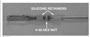
□ □ 2. Fit a silicone retainer, one 4-40 nut, another silicone retainer and the clevis on the end of a 4-40 threaded one end pushrod. Screw the clevis on 14 turns and temporarily connect it to the aileron servo arm.
