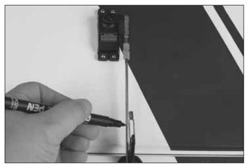
□ □ 4. Align the pushrod with the clevis on the control horn and make a mark using permanent marker or Panel Line Pen where the pushrod extends 1/8" [3 mm] into the open area of the clevis. Trim the 4-40 rod to length.
