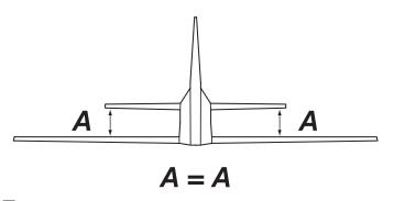
□ 3. Test fit the **stab** into the opening in the back of the fuselage. Stand back and look at the stab in relation to the wing. The stab should be parallel with the wing. If not, sand the stab saddle until the stab and wing are aligned.
