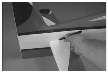
5. Trace the outline of the fuselage onto the stab using a felt tip marker or Panel Line Pen. Do this on both the top and bottom of the stab.
