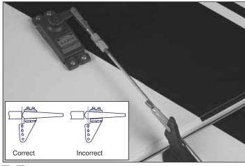
☐ ☐ 3. Attach one solder clevis to a black nylon control horn and position it on the aileron as shown in the sketch
