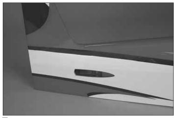
1. Locate the stab mounting slots near the rear of the fuse and remove the covering using a sharp hobby knife.
