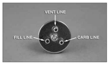
☐ 3. Slide the three aluminum fuel tubes into the rubber stopper as shown.
