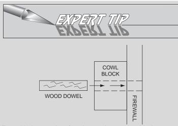
For added strength, after the cowl mounting blocks are all securely epoxied in place, drill 1/8" [3.2 mm] holes through the center of each block into the firewall. Insert an appropriate length of 1/8" [3.2 mm] wooden dowel (not included) into this hole and into the firewall. Glue this in place using thin CA. This modification is especially useful for high vibration engines.
