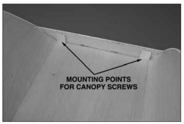
Attach the canopy to the fuselage using four #2 x3/8" [9.5 mm] screws and #2 flat washers. There are wooden reinforcement pieces on the inside edge of the cockpit area for the screws. If you wish to install a pilot figure (not included), you should do so now. This is also a good time to paint the interior cockpit area if desired.
