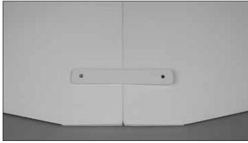
9. Glue the wing bolt in place using medium CA. After the plate is installed, run a bead of medium CA around the edges of the plate to prevent fuel from soaking into the balsa.
