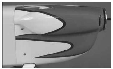
■ 8. Attach the cowl using six #4 x 1/2" [13 mm] screws and #4 flat washers. Be sure to harden the holes in the blocks with thin CA.
