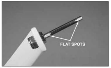
□ □ 3. File flat spots on the wheel axle where the wheel collar set screws will tighten down. A rotary tool with a flat grinding disc works well for this.
