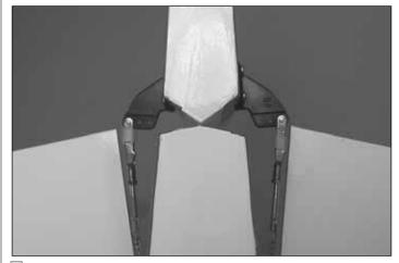
☐ 24. Fine tuning of the cable tension can be performed by adjusting the clevis on the coupler. When done adjusting the tension, secure the clevis by tightening the nut against the clevis. Be sure to apply a drop of thread locker to hold the nut in place.
