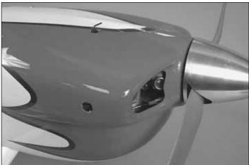
9. Once you have the cowl attached and aligned, make any necessary cutouts to access engine tuning screws, or
