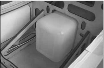
2. Insert the tank at a slight downward angle as shown in the first photo. Then level it out and slide it forward until the stopper assembly enters the cutout for it in the first former. When fully in place, it should rest as shown in the second photo.
