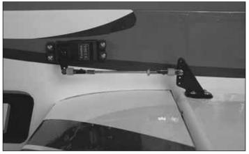
12. Follow the same procedure as the ailerons for connecting the pushrod and installing the control horns for both elevator halves.
