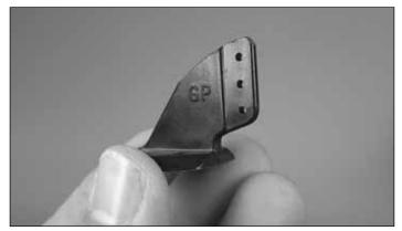
3. Trim the two rudder control horns as shown. This is necessary to allow the elevator halves to clear the horns.
