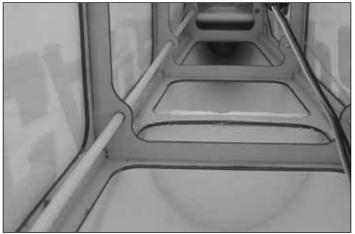
There is a pre-installed antenna tube in the fuselage of your CAP 232. Gently thread the antenna completely into this tube prior to flight.
