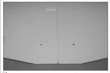
☐ 6. Locate the wing bolt holes in the aft center section of the wing. Remove the covering from these holes on the top and bottom of the wing using a sharp hobby knife.
