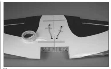
4. Mix another large batch of 30-minute epoxy, 1 oz should do. Coat the other half of the wing joiner, wing joiner pocket and the two wing roots with 30-minute epoxy. Join the two wing halves and hold them together with masking tape until the epoxy has completely hardened. Clean up any excess epoxy with alcohol and a paper towel.
