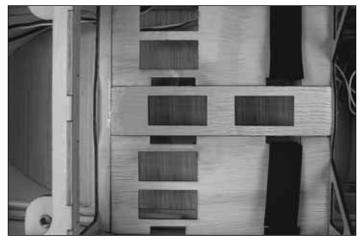
4. Align the radio trays as shown in the photo. Glue the radio trays in place using medium or thick CA. For added strength, epoxy may be used.
