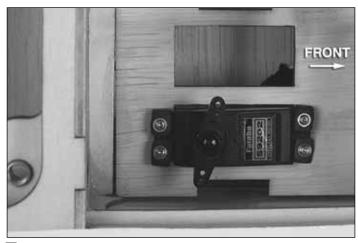
1. Install the throttle servo into the servo tray using the hardware provided by your servo's manufacturer. Choose the mounting position that gives you the most direct route to your carburetor. For the Fuji-Imvac 43cc gas engine, typically the servo location would be in the far right mounting position as shown.
