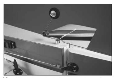
☐ 10. Slide the large wheel collar onto the tail gear wire and insert it into the tail gear bearing.
