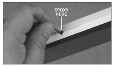
4. Mix approximately 1/8 oz of 30-minute epoxy. Use a toothpick to **thoroughly** apply the epoxy in the holes in the aileron. Use the toothpick to get the epoxy out of the outer edge of the opening of the holes in the aileron so it doesn't get into the hinge pins. Wipe away any epoxy around the outside of the holes with a paper towel.
