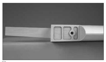
☐ 2. Test fit the wing joiner in one half of the wing. Sand as needed to allow the joiner to fit snug in the wing. Then slide the other wing half onto the joiner. There should be no gap between the wing halves when joined. Note the direction of the joiner. The "V" of the joiner should be towards the bottom of the wing.
