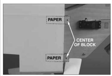
4. Mark the center of each hardwood block. From this mark, run a 2" [51 mm] piece of paper straight back onto the fuselage to use as templates.
