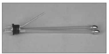
☐ 5. Attach silicone fuel lines 6" [153 mm] in length to the fill and carb tubes on the stopper. Install fuel clunks on each of these lines.
