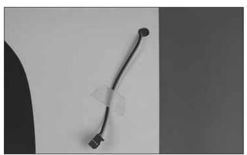
4. Located in the wing in the aileron servo compartment, a string is taped to the inside of the wing covering. Tie the string to the end of the servo wire. Then pull the servo wire through the wing with the string. Feed the servo wire out of the hole in the top of the wing. Tape the servo wire to the wing to prevent it from falling back into the opening.
