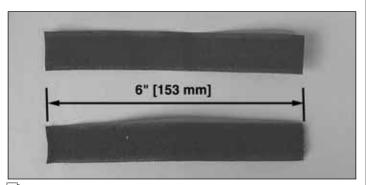
☐ 2. Locate the black hook and loop tape supplied with the ARF. Cut it into equal lengths of approximately 6" [153 mm].
