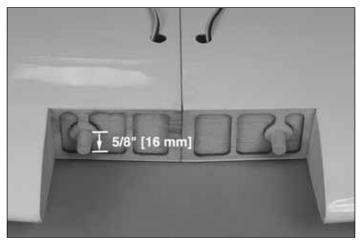
□ 5. Locate the two 3/8" [10 mm] x 2" [51 mm] wooden wing dowels. Round the edges of the dowels. Test fit the dowels into the holes in the forward center section of the wing as shown. Approximately 5/8" [16 mm] of the dowel should be sticking out of the wing. Glue in place using epoxy.
