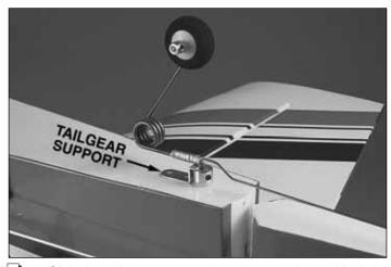
☐ 11. Slide the tail gear support into place as shown. Mark the location for the screw holes and drill 1/16" pilot holes at these marks. Attach the support to the fuselage using the supplied #2 x 1/4" [6 mm] screws. The height of the tail gear can be adjusted by loosening the set screw on the large wheel collar. The tail gear should not touch the top of the tail gear support when rotated. Lock the gear height in place using the wheel collar.
