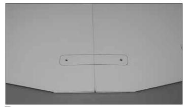
■ 8. Align the holes in the wing bolt plate with the holes in the wing. Trace an outline around the wing bolt plate. Trim away the covering approximately 3/32" [2 mm] inside the outline. Be careful not to cut into the balsa structure as this could weaken the wing.
