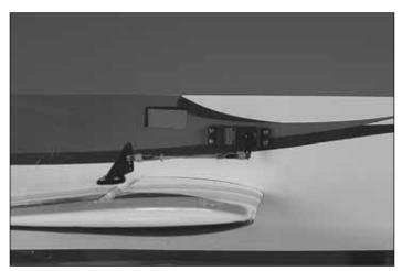
2. Remove the covering from the rudder servo bays using a sharp hobby knife.
