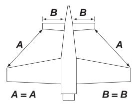
4. Measure the distance from the tip of the stab to the tip of each wing. Also measure the distance on each side of the fuselage. Adjust the position of the stab until A=A and B=B.
