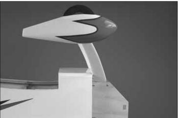
☐ 6. Mount the left and right landing gear assemblies to the fuselage using six 6-32 x 1-1/4" [32 mm] SHCS, six #6 washers, and six #6 lock washers as shown.
