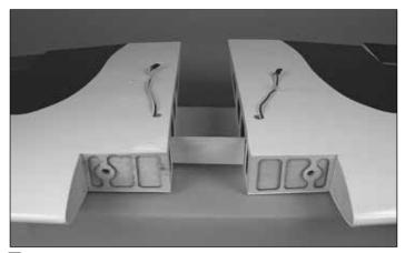
□ 3. When satisfied with the fit, separate the wing panels and remove the joiner. Mix a large batch of epoxy, enough to cover one half of the wing joiner and the inside of one wing joiner pocket. Half of one epoxy mixing cup, or 1/2 oz of epoxy should work fine. Coat half of the wing joiner and one wing joiner pocket with epoxy and insert the joiner. Clean up any epoxy that oozes out using a paper towel and denatured alcohol. Allow the epoxy to fully harden before proceeding.
