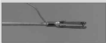
☐ C. Simultaneously heat the clevis and pushrod. Apply silver solder (GPMR8070) to the joint. The heat of the parts being soldered should melt the solder, thus allowing it to flow.
