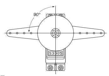
■ 5. Using your radio, center both rudder servos. Attach the servo wheels with the extender to the servo. Align the arm extender so that it is perpendicular to the servo as shown. Use a small drop of medium CA to tack glue the arm in place once you have it aligned correctly.
