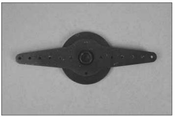
4. Test fit the servo arm extension as shown. The servo arm extension should self-center on the servo wheel.
