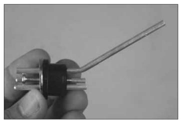
4. Cut the fill line and carb line tubes so that the tubes extend 1/2" [13 mm] out from both ends of the stopper. The vent line should be bent upwards and left uncut.
