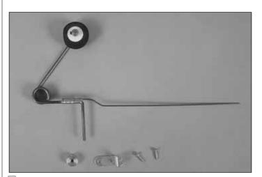
7. Locate the tailwheel assembly, nylon tail gear bearing, nylon rudder post, tail gear support, and large wheel collar. If it has not already been done for you, slide the 1" [25 mm] tailwheel and small wheel collar onto the tail wheel wire as shown. Grind a flat spot on the wire as you did with the main landing gear axles where the set screw tightens down.
