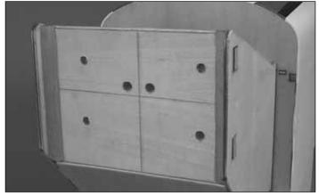
☐ 3. Remove the template and enlarge the holes using a 1/4" [6 mm] drill bit.
