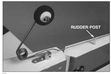
☐ 13. Glue the rudder post in place using a small amount of epoxy.
