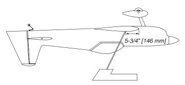
■ 2. With the wing attached to the fuselage, all parts of the model installed (ready to fly) and an empty fuel tank, place the model upside-down on a Great Planes CG Machine, or lift it upside down at the balance point you marked.
