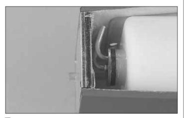
□ 11. Fit the tank into the fuselage. Mark the outside of the fuselage in the approximate location of the fuel lines from the tank. Remove the tank. Drill 1/4" [6mm] holes for the fuel lines. Harden the wood around the holes you just drilled with thin CA.
