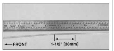
□ 10. Remove the pushrods. Make another mark 1-1/2" [38mm] in <u>front</u> of the first. At the forward mark make a slight bend. Reinstall the pushrods and attach the clevises. **Note:**
