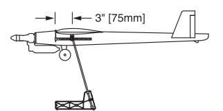
□ 2. With the wing attached to the fuselage, all parts of the model installed including the fuel tank hatch (ready-to-fly) and an empty fuel tank, place the model as shown above on a Great Planes CG Machine, or lift it at the balance point you marked.
