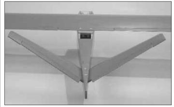
□ 4. Stand two to three yards or meters behind the plane and sight straight down the center of the fuse. Without moving side to side, approach the plane until you can see if the LE of the V-tail aligns with the TE of the wing. If they do not align, sand the high side of the wing saddle a small amount at a time until the wing and V-tail align with each other.
