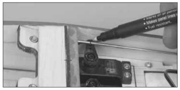
□ 13. Slide the ruddervator pushrods into the pushrod tubes and connect the clevises to the control horns. Keeping the ruddervator centered, mark the pushrod where it crosses the center of the servo arm.
