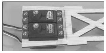
□ 3. Fit the tail servos into the servo tray. Drill 1/16" [1.6mm] holes for the servo screws and apply thin CA to the holes. Mount the servos to the tray with the screws provided with the radio gear.
