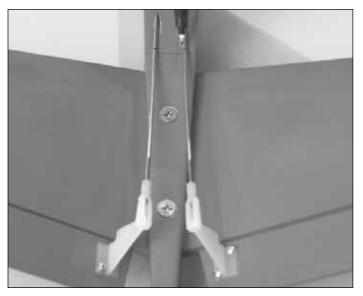
□ 9. Slide the 17-1/2" [445mm] pushrods into the guide tubes in the fuse. Connect the clevises to the outer hole on the control horns. With the elevators centered, mark the pushrods where they cross the V-tail joint.
