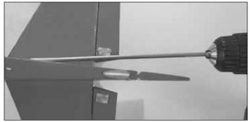
■ 9. Use the brass tube to drill a hole through the fuse in the approximate location and angles shown in the photo.
