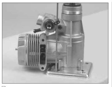
□ 2. Temporarily mount the engine to the backplate engine mount. Use a pushrod aligned with the carburetor arm to determine the location for drilling the hole through the engine mount. Mark the mount where the pushrod enters.
