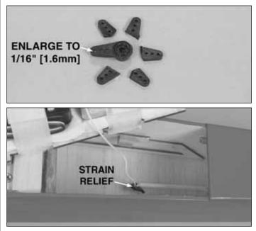
□ 10. Using an arm cut off the aileron servo, put a strain relief on the antenna and feed the antenna through the antenna tube. The excess antenna hangs out of the bottom of the airplane. **DO NOT CUT THE ANTENNA.**
