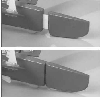
□ 7. Cut the hinge slots and mount the rudder with one long hinge.
