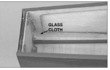
□ 5. Cut a 6" [150mm] piece off the 11-3/4" [300mm] outer pushrod tube. Roughen one end of the 6" [152mm] pushrod tube with coarse grit sandpaper. Glue the roughened end of the pushrod tube to the firewall with 1/8" [3mm] protruding from the front of the firewall.
