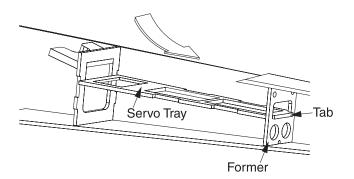
□ 6. Taking your time, slide the servo tray into the fuse. The back of the servo tray fits into a notch in the former. Because of this, the back of the servo tray needs to be lifted as much as possible while sliding the tray in place to get it positioned properly.
