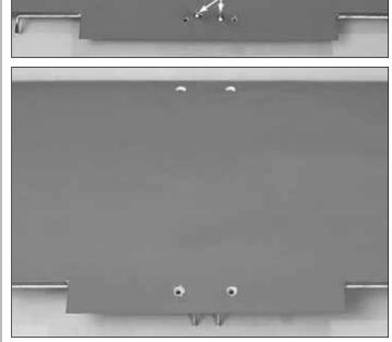
□ 1. Looking at the bottom of the wing as shown in the top photo (the aileron torque rods protrude from the bottom of the wing), cut the covering from the servo opening and the bottom of the four wing bolt holes. Turn the wing over and cut the covering from the top of the 4 bolt holes.
