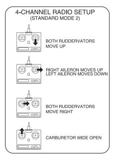
□ 3. Make certain that the control surfaces and the carburetor respond in the correct direction as shown in the diagram. If any of the controls respond in the wrong direction, use the servo reversing in the transmitter to reverse the servos connected to those controls. Be certain the control surfaces have remained centered. Adjust if necessary.
