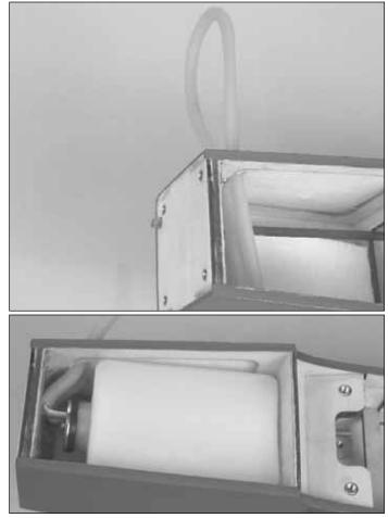
□ 12. Guide a 12" [300mm] piece of fuel line through the holes from the outside. Attach the lines to the tank and fit the tank in place.
