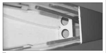
□ 10. Slide a 3/16" [5mm] plastic pushrod outer tube (not included) into the fuse from the rear, going through the large opening in the former and aligning the front of it with the rear of the servo mounts. **Note:** The servo tray is removed for clarity.
