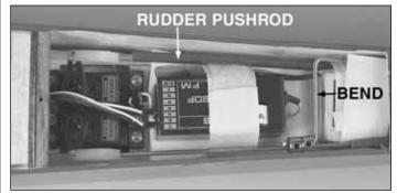
☐ 14. Attach the pushrods to the ruddervators. Bend the right ruddervator pushrod as shown. Connect the two ruddervator pushrods together with two 5/32" [4mm] wheel collars.
