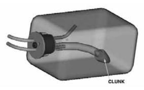
□ 9. Arrange the stopper and tubes as shown and insert them into the tank. Tighten the screw to expand the stopper, thus sealing the tank. Be certain the fuel line weight (clunk) at the end of the fuel line inside the tank does not contact the rear of the tank. Otherwise, the line may become stuck above the fuel level and discontinue fuel flow.
