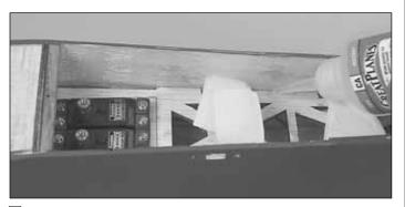
□ 7. Glue the servo tray to the fuse with thin CA, then with thick CA.
