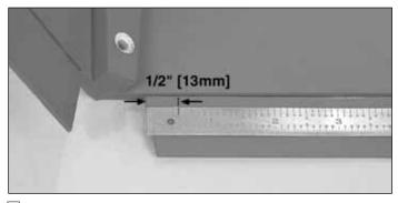
□ 5. Mark the top LE of both ruddervators 1/2" [13mm] from the inboard edge.
