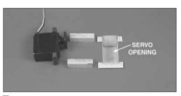
□ 1. Test fit the aileron servo and the  $3/8" \times 3/8" \times 1-1/4"$ [9.5 x 9.5 x 32mm] basswood aileron servo rails in the wing. Mark the covering around the rails. Remove the covering from the contact area between the rails and the wing. Epoxy the rails to the wing.
