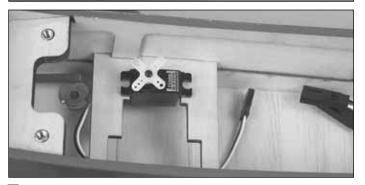
□ 21. Determine the size of the throttle servo you are going to use. Using the photos as a reference, mount the throttle servo in the tray so that it aligns with the throttle pushrod. Fit the tray in the airplane, being sure to leave at least a 1/16" [1.6mm] gap between the servo and the landing gear rail. Glue the servo tray securely to the fuse sides.
