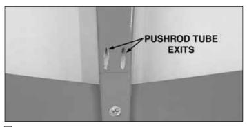
■ 8. Trim the covering from the pushrod tube exits that are in front of the V-tail on top of the fuse.
