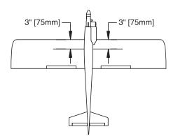
□ 1. Use a felt-tip pen or 1/8" [2mm] wide tape to accurately mark the C.G. on the bottom of the wing on both sides of the fuselage. The C.G. is located 3" [75mm] back from the leading edge of the wing.
