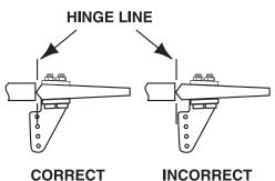
□ 6. Position the control horn centered over the mark. Mark the hole locations on the ruddervators. Drill 1/16" [1.6mm] holes through the ruddervators for mounting the control
