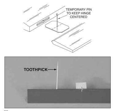
□ 6. Stick a pin through the center of each hinge. Fit the hinges into the ailerons. Use a toothpick to push epoxy into the torque rod hole in the aileron. Fit the ailerons to the wing
