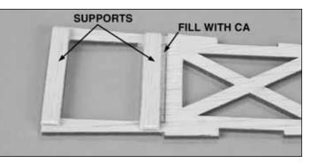
□ 2. Glue the V-tail servo supports to the servo tray. The side you glued the supports onto is now the bottom. **Note:** If you used servos smaller than standard, fill the cut lines with medium CA.
