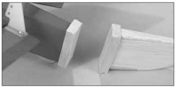
$\Box$  3. Glue 1/4" x 1/2" x 1-1/2" [6 x 13 x 38mm] balsa to the TE of the fuse and LE of the rudder
