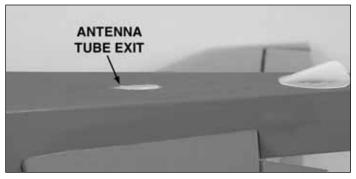
9. Remove the covering from the antenna tube exit at the rear of the fuse.
