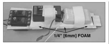
□ 5. Attach your receiver and receiver battery to the top of the servo tray. Use 1/4" [6mm] foam to isolate vibration, and the included hook-and-loop material to hold them in place. Remove the receiver and receiver battery.
