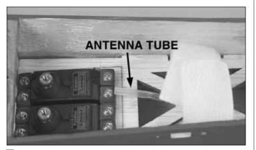
8. Lift the plastic antenna tube up through the servo tray. Reinstall the receiver and receiver battery.
