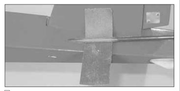
☐ 11. Mark the pushrod tube where is exits the fuse. Use course sandpaper to roughen the pushrod tube from the mark to 1-1/2" [38mm] forward of the mark.
