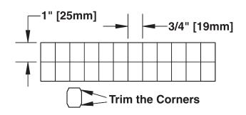
□ 2. Cut six 3/4" x 1" [19 x 25mm] hinges from the 2" x 9" [50 x 230mm] CA hinge strip. Snip the corners off so they go in the hinge slots more easily.
