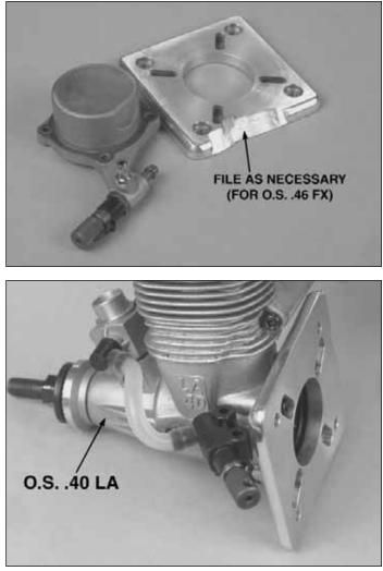
↓ 1. Remove the bolts from the engine backplate. Test fit the mount to the engine. If necessary, file the mount to accommodate the needle valve (required if using the O.S.<sup>®</sup> .46 FX), or relocate the remote needle to the engine mounting lug (required for the O.S. .40 LA), as shown in the photographs.
