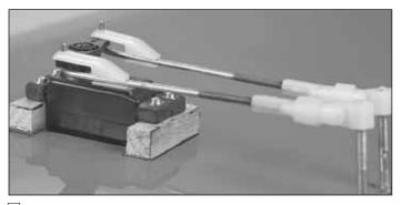
☐ 7. Slide the silicone retainers over the pushrods and onto the clevises. Bend the pushrod upward 90 degrees on the mark you made. Attach the pushrods to the servo arm with two Faslinks. Cut off the excess pushrod. Be certain to leave 1/16" [2mm] of wire protruding from the Faslink as shown.
