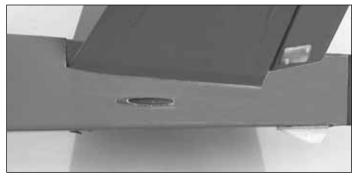
□ 12. Glue the tube to the fuse with thin CA. Allow the CA to cure and then cut off the excess tube.
