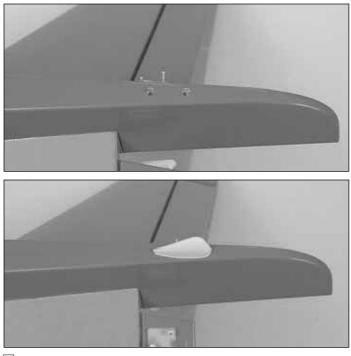
□ 3. Remove the covering from the two tail-skid mounting holes on the bottom of the fuse. Enlarge the tail-skid mounting holes with a 1/8" [3mm] drill. Glue the nylon tail-skid in place with medium CA.
