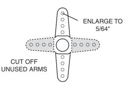
□ 3. Make a two-sided servo arm. Enlarge the holes in the arm with a Hobbico Servo Horn Drill (or a #48 or 5/64" [2mm] drill bit) so the aileron pushrods will fit.
