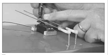
□ 6. Attach the clevises to the torque rod horns. With the servo centered, the servo arm parallel to the LE of the wings and the ailerons centered, use a fine-point felt-tip pen to mark the spot that the pushrods cross the outermost holes in the servo arm.
