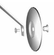
1. Mount the wheels to the landing gear with the 6-32 x 1/4" [6mm] bolts and axle as shown in the sketch.
