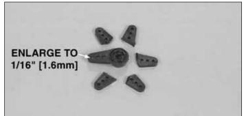
□ 12. Make three single-sided servo arms from three of the six-sided arms provided with the servos. Enlarge the outer two holes with a 1/16" [1.6mm] drill bit. **Note:** Even though some of the photos show servo wheels, servo arms are recommended.
