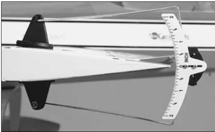
Moving the clevis inward on the control horn results in more throw.
