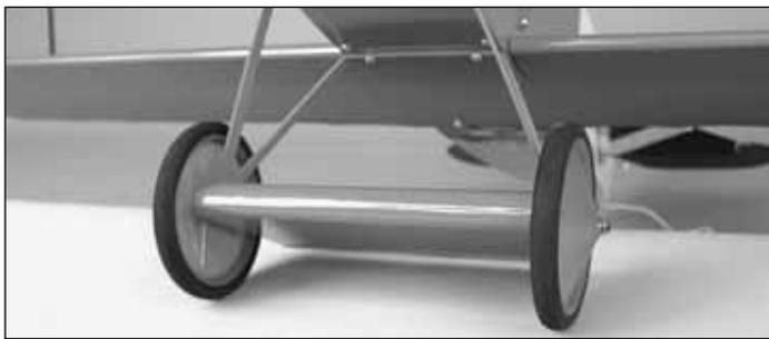
5. On each axle, place a 3mm [1/8"] washer and 3mm [1/8"] nut with threadlocker, followed by another 3mm washer and the wheel. Secure the wheel in place with a 3mm [1/8"] washer and 3mm [1/8"] nut. Apply a drop of threadlocker to the nut.
