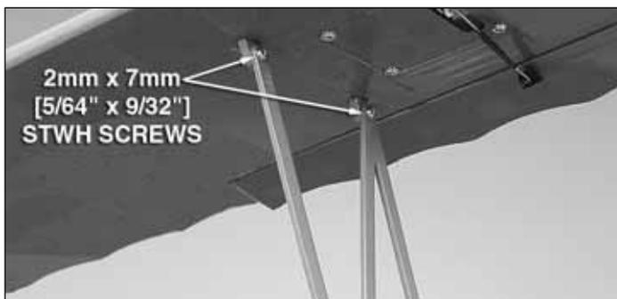
□ 8. Use four 2mm x 7mm [5/64" x 9/32"] self-tapping washer head screws to finish fastening the end struts in place as shown. Once you have determined that the wing is straight, with no twists, use thin CA to glue the strut mounts into the strut mount pockets. **IMPORTANT: Do not glue the struts to the strut mounts.**
