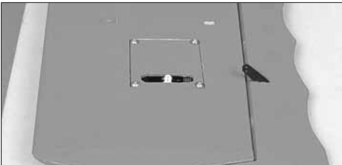
❑ 11. Test fit the control horns and when satisfied with their fit, CA them in place as shown.
