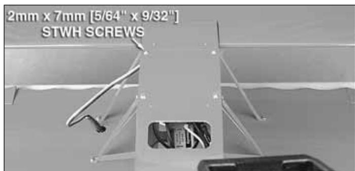
□ 1. Locate the radio compartment cover and secure it to the fuselage with four 2mm x 7mm [5/64" x 9/32"] self-tapping washer head screws as shown. Remove the screws and harden the holes with thin CA. Then, reinstall the screws.
