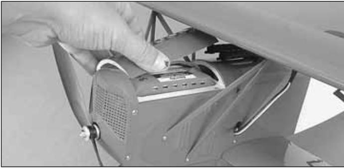
❑ 11. Remove the battery compartment cover. Note that the lip slides under the cowl and the aft end is held on with two magnets. Insert the battery in the battery compartment and replace the battery compartment cover.
