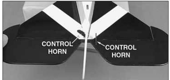
2. Test fit the control horns in the holes so that they are perpendicular to the control surface. Once satisfied with the fit, use CA to secure the control horns in place.
