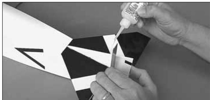
❑ 13. Use a small modeling square to make sure that the fin is perpendicular to the stabilizer and secure it in place with CA.
