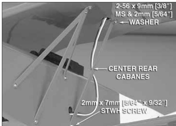
7. Put the center rear cabanes in place. Attach the cabanes with 2mm x 7mm [5/64" x 9/32"] self-tapping washer head screws at the sides of the fuselage and with 2-56 x 9.5mm [3/8"] machine screws and two 2mm [5/64"] washers in the bottom of the top wing.
