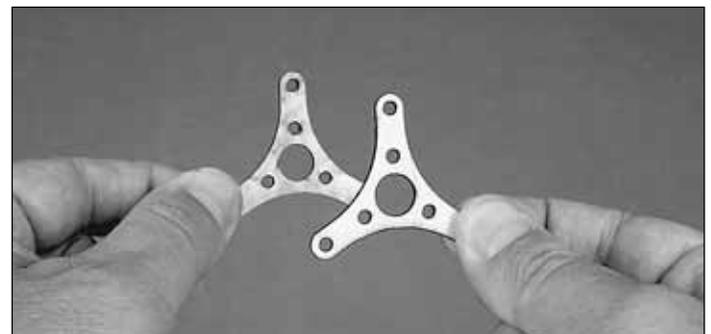
3. Use epoxy to join the two piece motor mount. Make sure all openings are flush.
