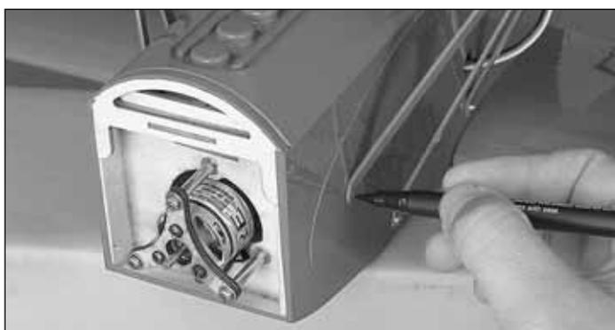
□ 9. Glue the cheek vents in place as shown. You will need to remove the screw from the front of the "V" strut and slide the cheek in place. Use a felt-tip pen to make a mark to show where to drill. Once the hole is drilled, simply slide the cheek vent in place and re-install the 2mm x 7mm [5/64" x 9/32"] self-tapping washer head screw.
