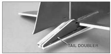
4. Glue the two **tail doublers** to the aft end of the fuse as shown.
