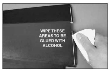
□ □ 1. For the best adhesion on the painted surfaces, we recommend roughing up the painted surfaces to be glued with fine grit sandpaper such as 320-grit. Wiping the areas to be glued with a paper towel dampened with denatured alcohol will reduce the gloss of the paint and also improve adhesion. If using alcohol, we recommend only making one pass with the towel. Excessive wiping will completely remove the paint from the foam.
