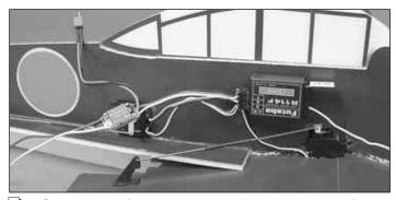
☐ 1. Cut a piece of the included double-sided tape to fit your receiver and stick it to the underside of the receiver case. Connect the ESC, aileron, rudder, and elevator servos to the receiver. Peel the backing from the double-sided tape and secure the receiver to the fuse in the location shown in the photo. Be sure that you have the servo wires positioned so that they do not interfere with the pushrods.
