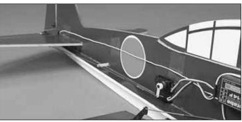
□ 6. The receiver antenna can be taped to the side of the fuse. However, be sure not to let excess wire hang free of this airplane if you plan to fly combat. Use alcohol to dull the painted surfaces where the tape will be applied. Wrap the excess wire through the elevator joiner tube cutout and tape it to the other side of the fuse. For a cleaner look, you can also cut a slit in the fuse and embed the antenna out of sight.
