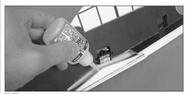
□ □ 2. Apply a bead of thick CA glue to the tops of the wing supports on the left side of the fuse. We recommend using CA accelerator to speed assembly time.
