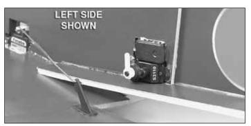
□ 3. Use your radio system to center the elevator and rudder servos. Cut three arms from two four-arm servo horns and install them onto the elevator and rudder servos, with the right one pointing down and the left one pointing up. Enlarge the **outer holes** of the servo horns and the rudder control horn with a 3/64" [1.2mm] drill bit. Enlarge the **inner hole** of the elevator control horn (closest to the elevator) with the same size bit.
