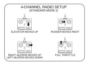
□ 3. Make certain that the control surfaces and the throttle respond in the correct direction as shown in the diagram. If any of the controls respond in the wrong direction, use the servo reversing in the transmitter to reverse the servos connected to those controls. Be certain the control surfaces have remained centered.
