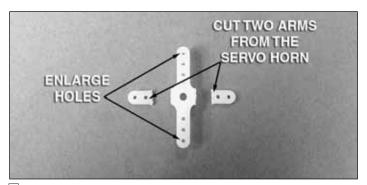
☑ 2. Cut two arms from a four-arm servo horn as shown. Enlarge the outer holes in the remaining servo arms with a 3/64" [1.2mm] drill bit.
