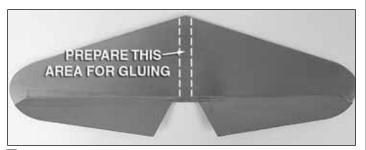
☐ 1. Roughen a 1/8" [3mm] strip down the center of the top and bottom of the **horizontal stabilizer**. Use alcohol to dull the paint at the area to be glued. Do the same to the area around the horizontal stab slot in the fuse.
