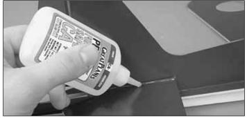
☐ 3. When satisfied, run a bead of thick CA glue along the top and bottom of the stab where it meets the fuse on both sides.
