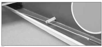
□ 5. Position the **pushrod supports** in the middle of the pushrods and lightly press them into the fuse, creating indentations in the foam. Be sure that the pushrod support location will not create any binding in the pushrod. Use a sharp hobby knife to cut a hole in the foam at the indentations you made. Insert the pushrod supports into the holes and glue them in place.
