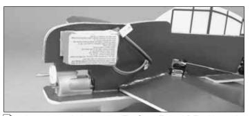
□ 3. In order to balance the FlatOuts Zero ARF without the addition of weight, the battery pack must be secured above the motor. Use the included **hook and loop material** to do so with the "loop" side on the battery. Applying the "loop" side of the hook and loop material to the front side of the battery will allow the battery discharge leads to reach the ESC battery connectors. The discharge leads will pass through the hole in the fuse to connect to the ESC.
