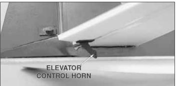
☐ 2. Enlarge the **outer hole** of a control horn using a 3/64" [1.2mm] drill bit. Install the control horn onto the left side of the rudder. Enlarge the **inner hole** (closest to the control horn base) of another control horn using the same drill bit and install it on the bottom of the **right elevator half**.
