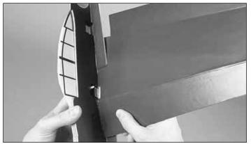
□ □ 3. Insert the **left wing panel** into the slot. The notch at the inside LE of the wing panel will contact the fuse when fully seated. The TE of the wing panel must be aligned with the center of the fuse.
