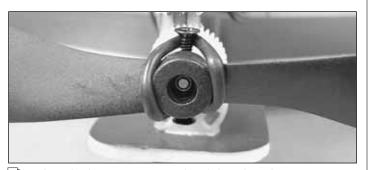
☐ 5. Attach the **prop saver** by tightening the two screws against the flat spots on the prop shaft.
