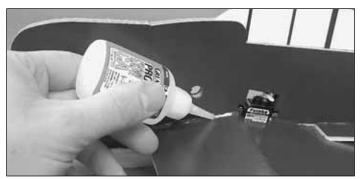
☐ ☐ 4. Apply a bead of CA around the joint between the wing and the fuse on the top and bottom.
