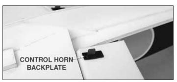
☐ 2. Press the control horn backplates onto the tabs to secure the control horns to the ailerons. Glue the backplates to the control horn tabs with a drop of CA.
