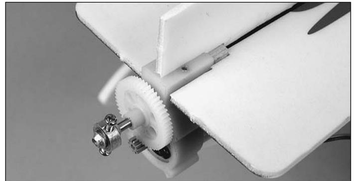
❑ 5. Drill a 1.5mm [1/16"] pilot hole at an angle from the top of the gearbox through the balsa block and carbon tubes. Make sure the motor mount block does not rotate while drilling. Secure the gearbox and block with a 2 x 8mm [5/64" x 5/16"] wood screw.
