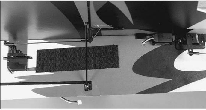
❑ 9. Install the “hook” side of the included hook-and-loop material to the left side of the fuselage where shown. This is where you will mount the battery.
