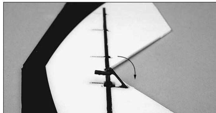
10. Coat the gluing area on the control horn with glue and rotate it down into the precut slot.
