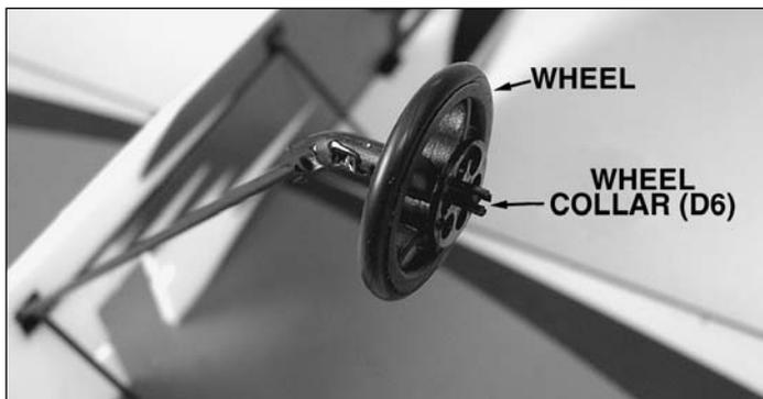
❑ 2. Slide the **wheels** onto the axles, and secure them with a **wheel collar (D6)**. The flat side of the wheel collar should be toward the wheel. Secure the wheel collar with a drop of glue in the *teeth* opposite the wheels. Align the wheels with the centerline and secure the axles and supports with a drop of glue through the holes in both sides of the axle supports.
