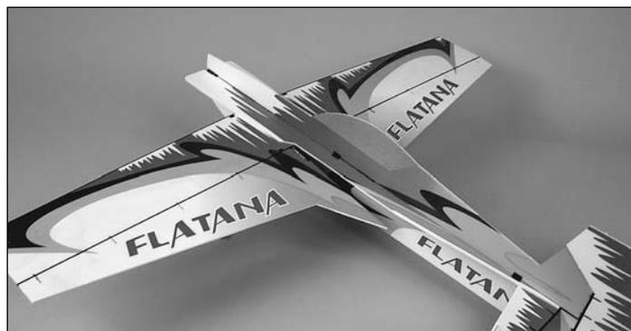
❑ 21. Snap the ailerons onto the wing TE.
