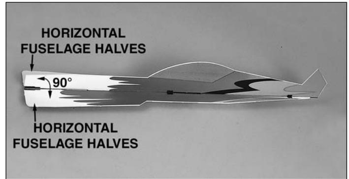
6. Glue the left and right horizontal fuselage halves to the fuselage tube. Make sure they are perpendicular to the upper vertical fuselage.
