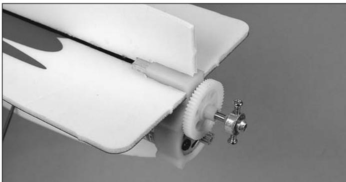
❑ 4. Slide the **motor/gearbox assembly** over the motor mount block.
