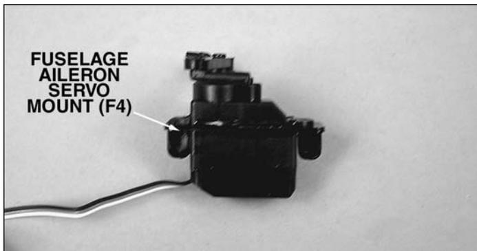
❑ 4. Install the servo arm on the aileron servo in the position shown. Both arms should be offset forward by the same angle. Glue the aileron servo into a **fuselage aileron servo mount (F4)**.
