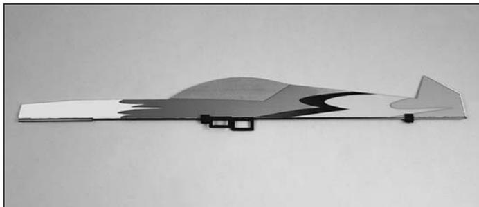
4. Position the servo mounts and fuselage joiners so that they align with the precut slots in the upper vertical fuselage half.
