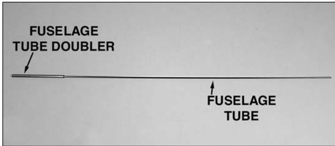
2. Glue the 5.5 x 115mm [7/32" x 4-17/32"] **fuselage tube doubler** over the 3 x 679mm [1/8" x 26-47/64"] **fuselage tube**. One end should be flush. From now on, this assembly will be referred to as the fuselage tube.
