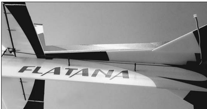
□ 12. Using the pushrod as a guide, drill two evenly-spaced 2.4mm [3/32"] holes through the fuselage for the pushrod guides. Glue the base of each pushrod guide into the holes.
