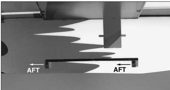
❑ 17. Installing them from the **right** side, glue two more supports into the slots in the fuselage. Note that these first two supports should be positioned **aft** in the slots, and that the holes in the supports should be angled downward and outward (again, to accommodate the angles of the landing gear and the struts).
