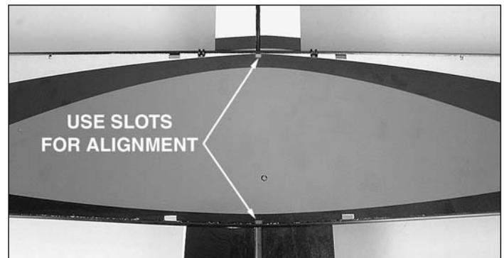
8. Glue the wing into position with the leading edge of the wing against the rear end of fuselage doubler tube. Align the notches in the wing with the fuselage tube.
