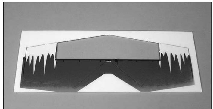
5. Using the **Expert Tip** that follows, permanently join the elevator halves by gluing in the elevator joiner tube.
