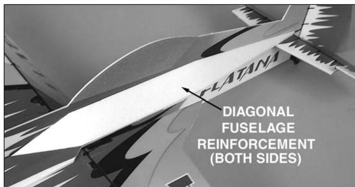
❑ 22. Using an Easy-Touch bar sander with 220-grit sandpaper, sand a bevel into the edges of the fuselage diagonal reinforcements at a 45° angle toward the inside. Glue the **diagonal fuselage reinforcements** into position where shown. Align the lower edges with the edges of the horizontal fuselage halves. Be careful not to twist the fuselage as you glue the parts down.
