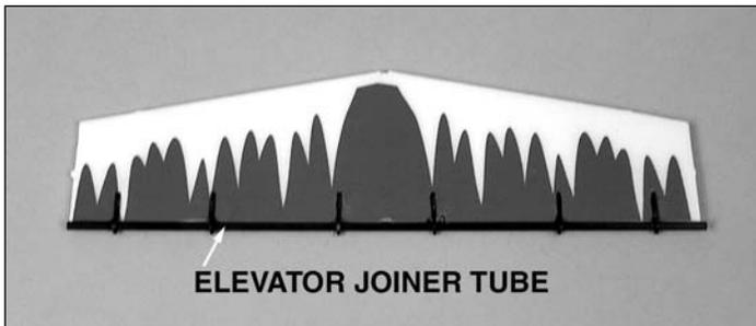
2. Following the **Expert Tip** below, use foam-safe CA and accelerator to glue six **clip hinges (C2)** into the stabilizer, using the 3 x 209mm [1/8" x 8-7/32"] **elevator joiner tube** as a guide.
