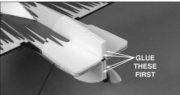
❑ 2. Glue the vertical fuselage doublers into position first, then glue the horizontal fuselage doublers into position.
