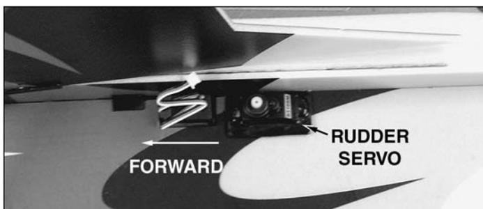
❑ 7. Glue the rudder servo into the **rear** servo mount in the left side of the fuselage. The output shaft should be forward.
