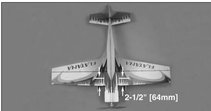
❑ 1. Use a felt-tip pen or 1/8" [3mm]-wide tape to accurately mark the C.G. on the top of the wing on both sides of the fuselage. The C.G. is located 2-1/2" [64mm] back from the leading edge of the wing at the fuselage.
