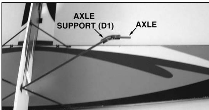
❑ 1. Install a 2 x 17mm [5/64" x 21/32"] **axle** and **axle support (D1)** onto each landing gear leg. Make sure that the axles are perpendicular to the centerline.
