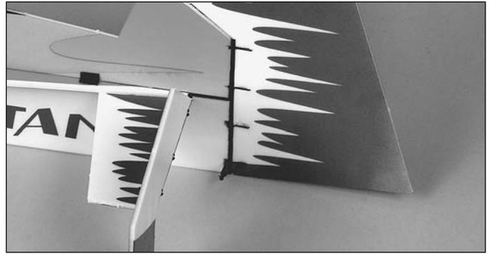
❑ 13. Snap the rudder onto the rudder post.
