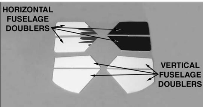
❑ 1. Cut the **horizontal** and **vertical fuselage doublers** from their foam sheets.
