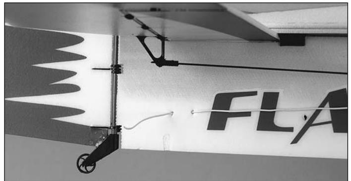
□ 15. Drill two 1.5mm [1/16"] holes through the fuselage where shown. "Stitch" the receiver antenna through these holes.
