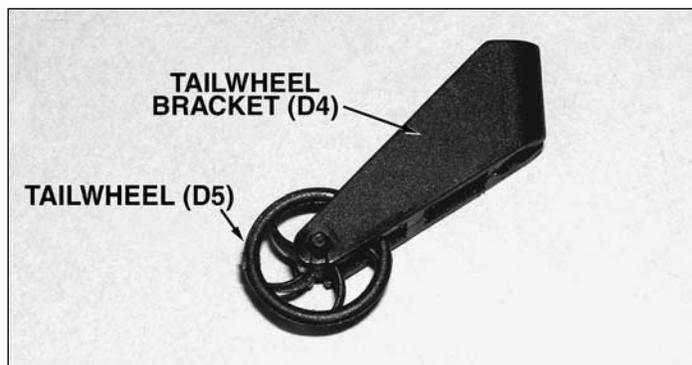
❑ 4. Snap the **tailwheel (D5)** into the **tailwheel bracket (D4)**.
