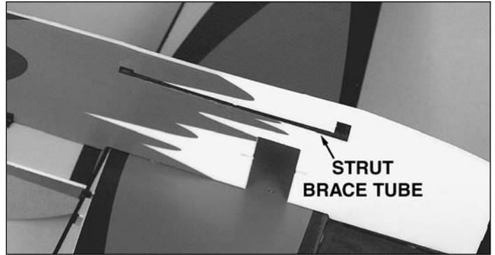
❑ 14. Glue the 3 x 111mm [1/8" x 4-3/8"] **strut brace tube** into the fuselage.
