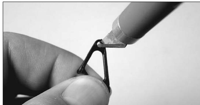
**A.** Using a sharp #11 hobby knife, remove any flashing from the inside of the hole you are installing the Z-bend clevis into. Do this by rotating the blade in the hole while applying gentle pressure. Be careful not to remove too much material—your goal here is to remove small ridges of flashing, not to make the hole larger.
