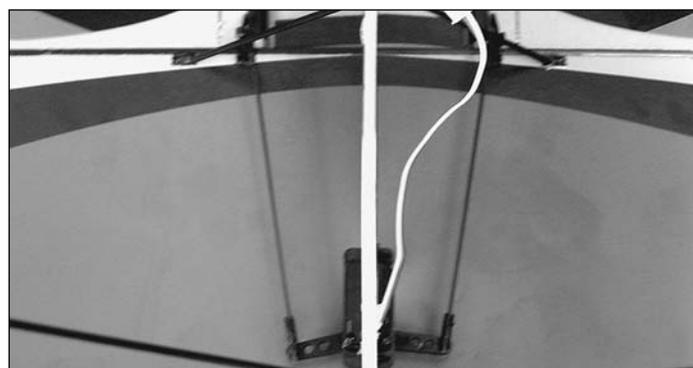
❑ 10. Slide a 1 x 95mm [3/64" x 3-3/4"] **aileron pushrod** through the clevises in the aileron horns and servo arms. Adjust the clevises until the ailerons are centered with the servo centered. When you have the alignment correct, secure the pushrod with a drop of glue where the pushrod enters the clevis. Keep glue away from the end of the clevis where it pivots in the arm or horn.
