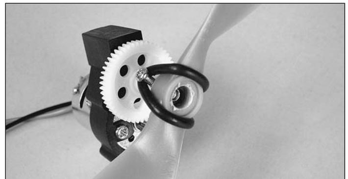
❑ 7. Secure the prop to the prop saver with one of the included O-rings.
