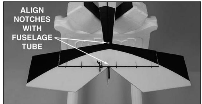
7. Glue the stabilizer into position with the leading edge of the stab butted against the rear fuselage joiner. Align the notches in the stab with the fuselage tube.
