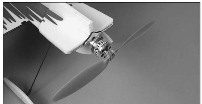
❑ 5. Mount the motor and propeller using the hardware and instructions that came with your motor.
