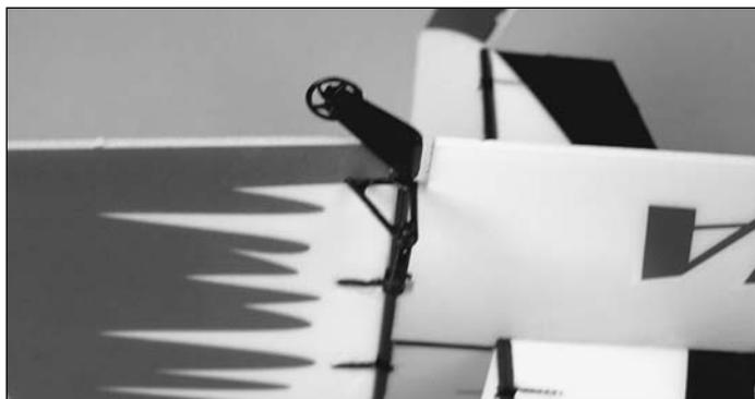
❑ 5. Slide the tailwheel bracket over the rudder and rudder post. Glue the bracket to the rudder **only**. **Do not** glue the bracket to the rudder post.
