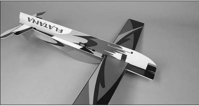
❑ 9. Glue the lower vertical fuselage half to the fuselage tube. Make sure to keep it parallel with the upper half and perpendicular to the horizontal fuselage.
