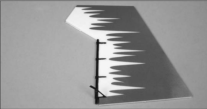
❑ 10. Using the 3 x 106mm [1/8" x 4-11/64"] **rudder post tube** as a guide, glue three clip hinges and a clip hinge control horn to the **rudder**.
