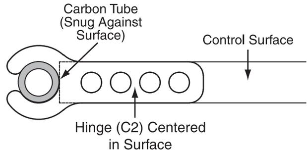
C. One at a time, coat the sides of the rest of the hinges and glue them into the slots.
