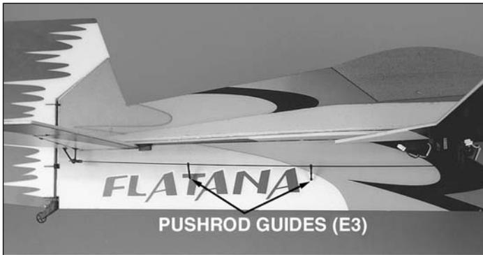
□ 11. Slide two **pushrod guides (E3)** onto the 1 x 365mm [3/64" x 14-3/8"] **elevator pushrod** and slide the pushrod through the clevises on the elevator servo arm and control horn. Adjust the clevises until the elevator is centered with the servo centered. Secure the clevises with a drop of glue on each clevis where the pushrod enters it.
