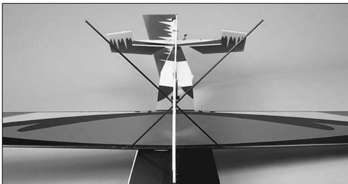
❑ 19. Slide the 2 x 220mm [5/64" x 8-7/8"] **landing gear legs** through the landing gear supports in the front of the wing and fuselage. Ensure that the wing is parallel with the stab and horizontal fuselage and perpendicular to the vertical fuselage. Once satisfied with the alignment, secure the landing gear legs with a drop of glue on both sides of each joint.
