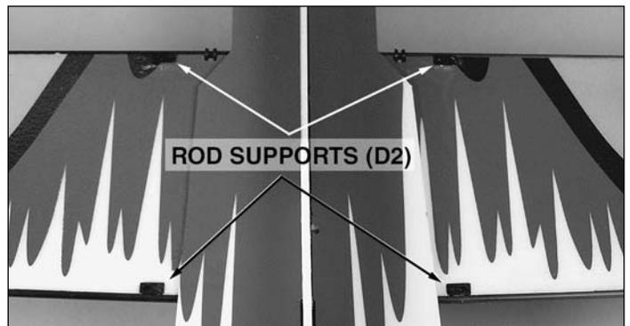
❑ 16. Installing them down through the top of the wing, glue four rod supports (D2) into the slots in both sides of the
