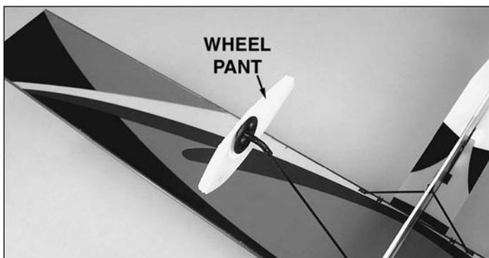
❑ 3. Make two wheel pants by gluing the **inner** and **outer wheel pant parts** together. Be sure to make a **right** and a **left**. Glue the inside of both wheel pants to the wheel collars.
