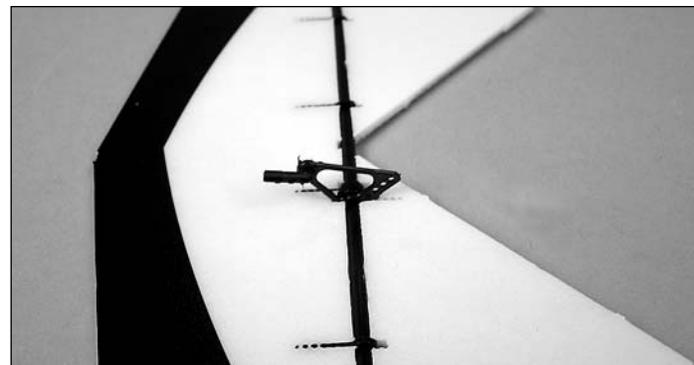
9. Clip the control horn onto the joiner tube aligned with the precut slot.
