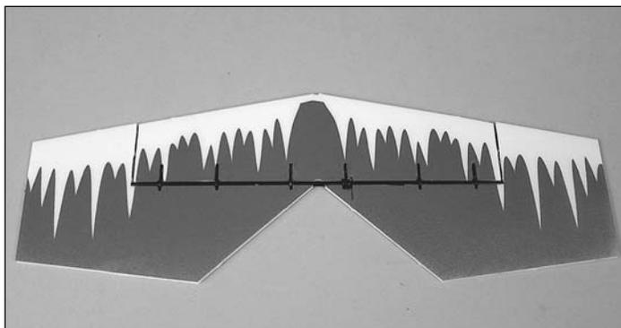
7. Join the elevators to the stab by snapping the clip hinges to the joiner tube.
