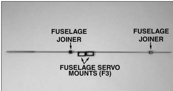
3. Slide a **fuselage joiner**, two **fuselage servo mounts (F3)**, and another fuselage joiner onto the fuselage tube. With the tube doubler forward, and the servo mounts hanging down, the front servo mount should have its flat surface on the right, and the rear servo mount should have its flat surface on the left.
