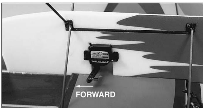
❑ 5. With the output shaft forward, glue the aileron servo into the cutout under the wing.
