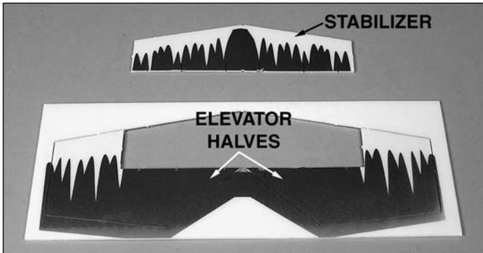
1. Cut the **stabilizer** free from the foam sheet using a hobby knife with a *sharp* #11 blade. **DO NOT** cut the **elevator halves** free at this time.
