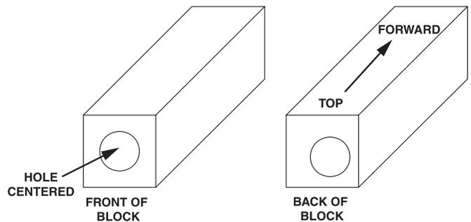
□ 1. The 10 x 10 x 27mm [25/64" x 25/64" x 1-1/16"] **hardwood motor mount block** must be mounted in the correct orientation. Identify the top, aft end of the block as shown in the sketch so you will know how it is to be installed.
