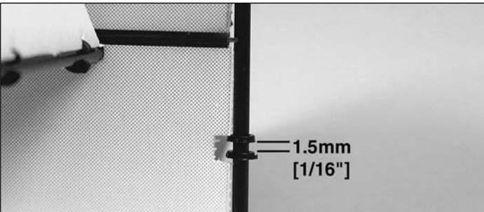
❑ 11. Remove the rudder post tube from the rudder. Slide two hinge retainer rings onto the bottom of the rudder post. Align the rings with the slot in the TE of the fuselage. Secure each ring with a drop of glue on the outside. Be careful not to get glue between the rings.
