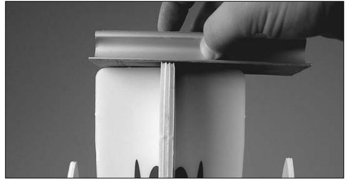
❑ 3. Use a 220-grit bar sander to **lightly** sand the front of the fuselage even. Be careful not to change the built-in thrust angles.
