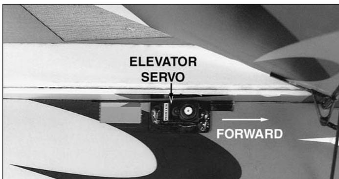
❑ 6. Glue the elevator servo into the **front** servo mount in the right side of the fuselage. The output shaft should be forward.
