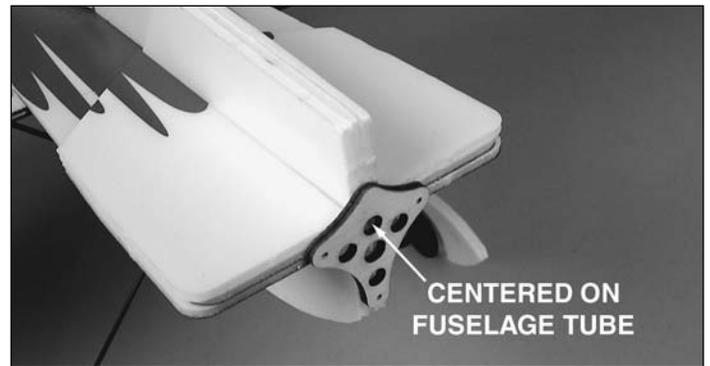
❑ 4. If installing an ElectriFly RimFire motor, glue the included 3mm [1/8"] plywood **firewall** to the nose so that the two pilot holes are centered on the horizontal fuselage, and the top hole is centered on the fuselage tube. **Note:** If installing another brand of outrunner motor, you will need to cut your own firewall to match its mount pattern. The motor and firewall should be mounted so that the thrust line is offset 9mm [11/32"] below the center of the fuselage tube.
