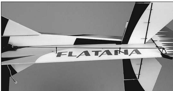
□ 13. Install the 1 x 360mm [3/64" x 14-11/64"] **rudder pushrod** the same way.
