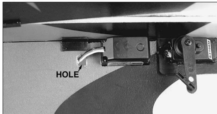
❑ 8. Select two single-sided servo arms to fit the elevator and rudder servos you are using. Insert a Z-bend clevis into the outer hole of each arm. Mount the servo arms so that they point straight down with the servos centered. Cut a small hole in the fuselage to allow the elevator servo wire to pass through to the right side of the fuselage.
