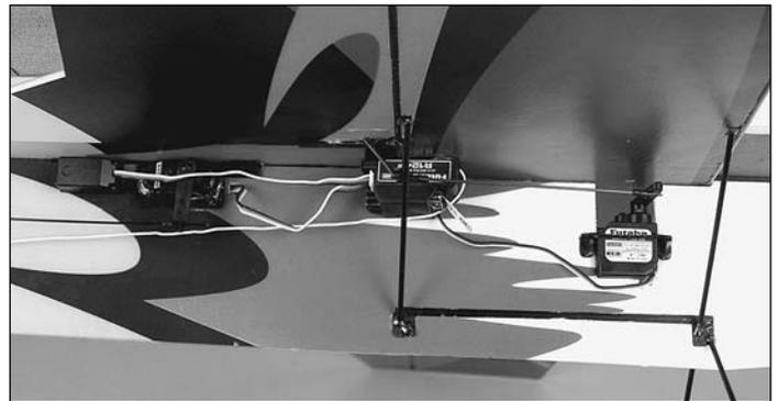
□ 14. Connect all three servos to the receiver. Mount the receiver to the bottom of the left horizontal fuselage with double-sided foam tape. Make sure the receiver is far enough forward so that it does not interfere with aileron motion.
