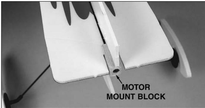
❑ 2. **Without using any glue**, slide the motor mount block over the fuselage tube. Be certain the block is in the correct position so there will be **down** and **right** thrust. **Do not** glue the motor mount block onto the fuselage tube.
