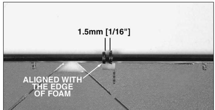
4. Without removing the elevator halves from the foam sheet, slide two **hinge retainer rings (C3)** onto the elevator joiner tube. Align the rings with the cutout in the right elevator half. There should be a 1.5mm [1/16"] gap between the two rings. Secure both rings to the tube with a drop of glue on the outside of the gap. Do not get any glue between the rings.
