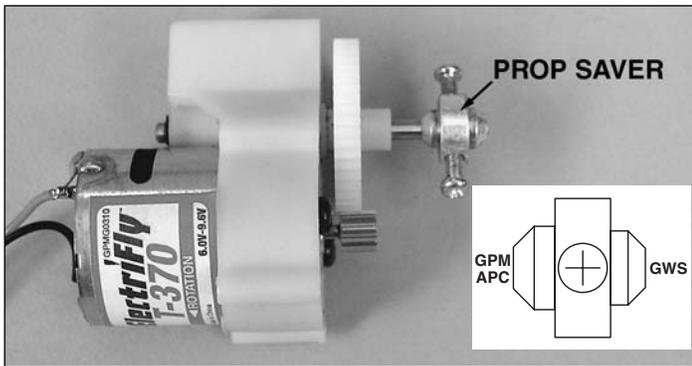
❑ 3. If using the included propeller, install the **prop saver** onto the gearbox shaft with the large-diameter cone forward. If using a GWS prop, install the prop saver with the small-diameter cone forward. Tighten the screws, making sure they engage the flat spots on the shaft.
