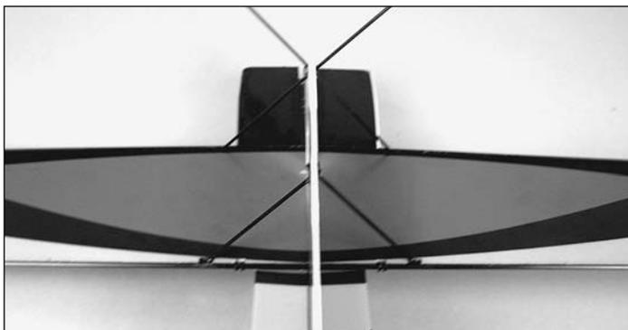
❑ 20. Slide the 2 x 86mm [5/64" x 3-3/8"] **wing struts** through both sets of supports in the back of the wing and
