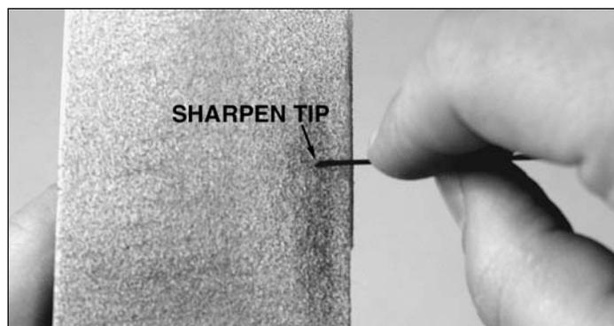
❑ 9. Using an Easy-Touch bar sander with 220-grit sandpaper, sharpen the ends of all the 1mm [3/64"] carbon **pushrods**. This will make it much easier to install them through the Z-bend clevises.
