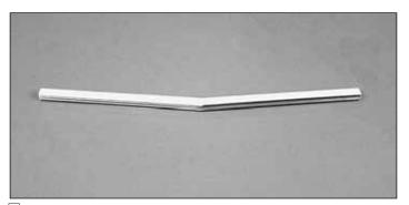
□ 2. Using epoxy, glue the joiner plates together. The two aluminum plates are glued between the two hardwood plates. Allow the epoxy to fully cure before proceeding.
