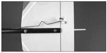
□ 11. Attach the elevator control horn and pushrod the same way as the rudder control horn. The elevator control horn is positioned 1/4" [6.4 mm] from the fuselage boom as shown. Ensure that the holes in the control horn align with the hinge line.
