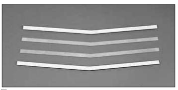
□ 1. Locate the two hardwood and two aluminum wing joiner plates.
