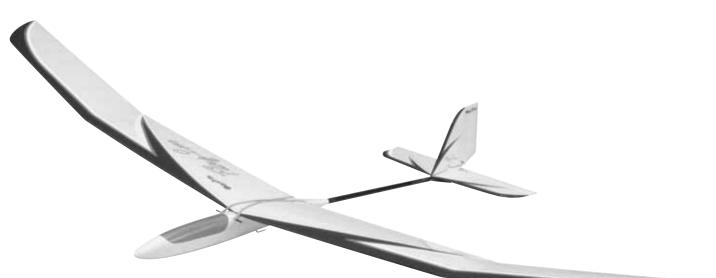
**Wingspan:** 78.5 in [1995 mm] **Wing Area:** 477 sq in [30.8 dm<sup>2</sup>] **Weight:** 19 - 21 oz [540 - 595 g] **Wing Loading:** 5.7 - 6.3 oz/sq ft [18 - 19 g/dm<sup>2</sup>] **Length:** 40 in [1015 mm] **Radio:** Minimum 2-channel with two micro, mini or standard size servos
