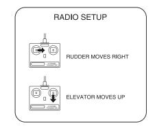
□ 3. Make certain that the control surfaces respond in the correct direction as shown in the diagram. If any of the controls respond in the wrong direction, use the servo reversing switch in the transmitter to reverse the servos connected to those controls. Be certain the control surfaces have remained centered. Adjust if necessary.
