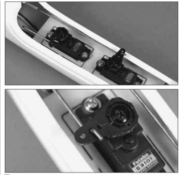
□ 6. Remove the servo arms and insert the Z-bend into the second hole out from center on the arms. Reattach the servo arms and servo arm screws.
