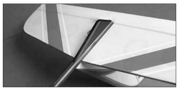
□ 8. Insert the tail skid post into the slot cut in the tail of the fuselage and glue in place using CA as shown.
