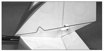
□ 8. Using pliers, bend the pushrod wire into the shape of a "V" as shown. This "V" can be modified after installation to adjust trim. Do the same for the elevator pushrod.
