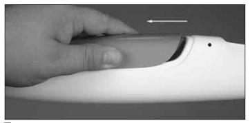
□ 1. Slide the **canopy** forward till the rear wire is visible.
