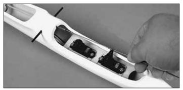
□ 5. Insert each wire into the pushrod guide tubes in the fuselage.
