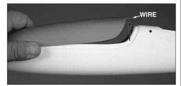
□ 2. Lift the rear of the canopy till the wire is clear of the **fuselage**.
