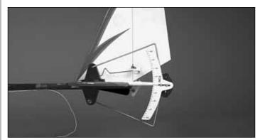
Use a Great Planes AccuThrow (or a ruler) to accurately measure and set the control throw of each control surface as indicated in the chart that follows. If your radio does not have dual rates, we recommend setting the throws at the **low rate** setting.
