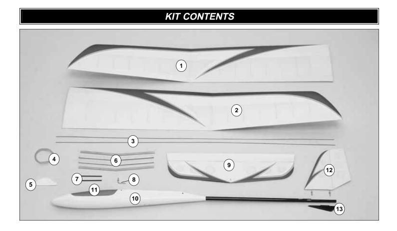
**Kit Contents** Left Wing Panel 8. Tow Hook Parts Not Shown 1. 2. Right Wing Panel 9. Stab Nylon Control Horns & Backplates (2) 2 x 1/2" [13 mm] Machine Screws (2) 40" [1016 mm] Pushrods (2) 3. 10. Fuselage 1/16" [1.6 mm] Wheel Collar 4. Rubber Bands 11. Canopy 5. TE Support 12. Fin #2 Lock Nut Aluminum Wing Joiner Plates (2) & 13. Plastic Tail Skid Halves (2) #2 Nuts (2) 6. #2 Flat Washers (2) Hardwood Wing Joiner Plates (2) 7. Carbon Fiber Wing Dowels (2)
