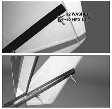
□ 4. Secure the tail assembly to the fuselage using two #2 hex nuts and #2 flat washers as shown. Be sure not to overtighten the nuts as the stab could become damaged. Apply a drop of Threadlocker to each hex nut to prevent it from backing off.
