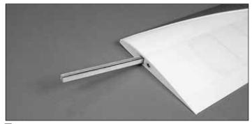
□ 3. Test fit the **wing joiner** into the slots in the wing halves. Sand the joiners as required to get a good fit. **Note:** If the root rib angles aren't exactly the same, that's OK. The difference can be filled with a little epoxy when the wings are joined. The proper dihedral angle and the gluing of the wing joiner are more important than the fit of the two wing panels.
