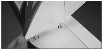
□ 2. Insert the **fin posts** into the holes in the stab as shown. These two parts joined together will be referred to as the **tail assembly** from this point.
