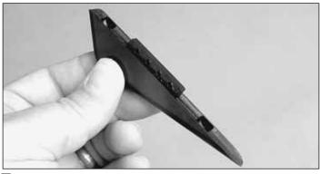
□ 7. Glue the two tail skid pieces together as shown using CA.
