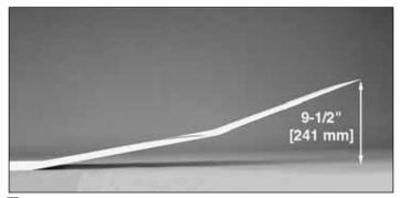
□ 5. With the **inner left wing section** flat on your workbench and the center joint on the wax paper, raise the right wing tip 9-1/2" [241 mm] to properly set the dihedral. Block the raised right wing at the desired height and make a mental note of the position needed for it to maintain that dihedral.
