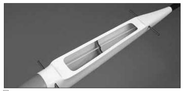
■ 8. Glue the carbon fiber **wing dowels** into the fuse with a small amount of thin CA. Be sure the length of the carbon on each side is equal.
