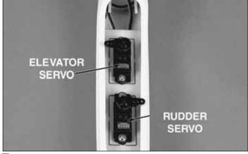
□ 3. With the servos centered, install a servo arm onto each servo. Trim the arms as shown.
