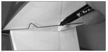
$\Box$  9. Make a mark on the pushrod where it crosses the control horn. Make a 90° bend at this mark and insert the pushrod into the second hole on the control horn.
