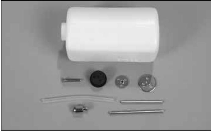
❑ 1. Locate the parts for the fuel tank. You will need only one long and one short aluminum tube. Cut the silicone fuel tube to a length of 3-1/2" [89mm].
