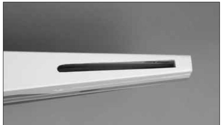
2. Locate the slot for the vertical fin on the top of the fuselage and remove the covering.
