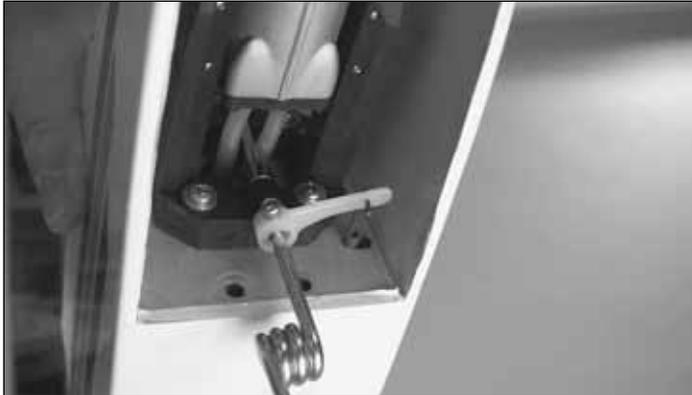
❑ 8. Locate the 1/16" x 17-1/2" [1.6 x 444mm] **non-threaded wire pushrod** and make a 90 degree bend 1/2" [13mm] from one end. Drill a 5/64" [2mm] hole through the **center** hole in the nose gear steering arm. Insert the straight end of the steering pushrod into the pushrod tube (from the firewall), into the pushrod connector on the rudder servo. Don't cut the wire or tighten the setscrew yet. Work the bent end of the wire into the steering arm as shown in the photo.
