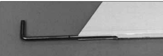
3. Carefully cut grooves into the leading edges of the elevator halves to allow the joiner to recess into the leading edge.
