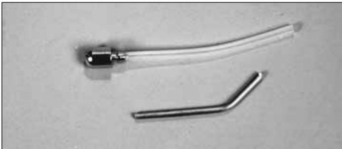
❑ 2. Push one end of the fuel tube onto the clunk. On the long aluminum tube, put a bend of about 40 degrees 1" [25.4mm] from one end.
