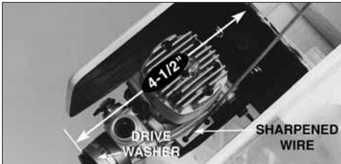
❑ 5. Position the engine so that the drive washer is 4-1/2" [114mm] from the firewall. Using one of the 17-1/2" [444mm] push rods, sharpen the non-threaded end using a file or sandpaper. Use this sharpened wire to scribe the four mounting holes onto the rails. Use a 7/64" [2.8mm] drill bit to drill pilot holes through the rails for the #6 sheet metal screws.
