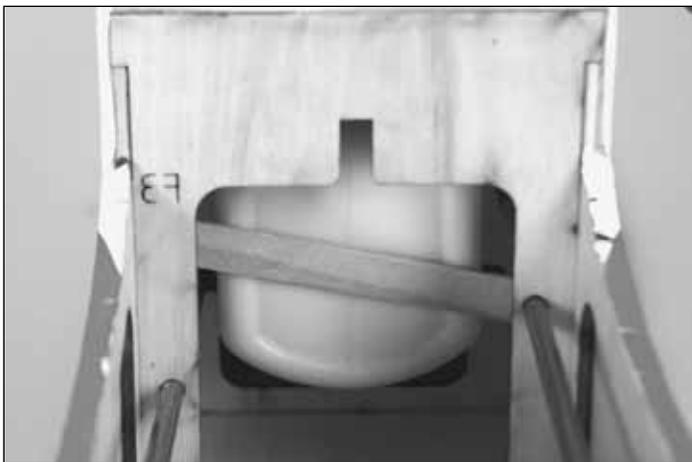
❑ 3. Secure the rear of the tank with a stick to prevent it from moving in flight. The photo shows an epoxy mixing stick glued with 6-minute epoxy.
