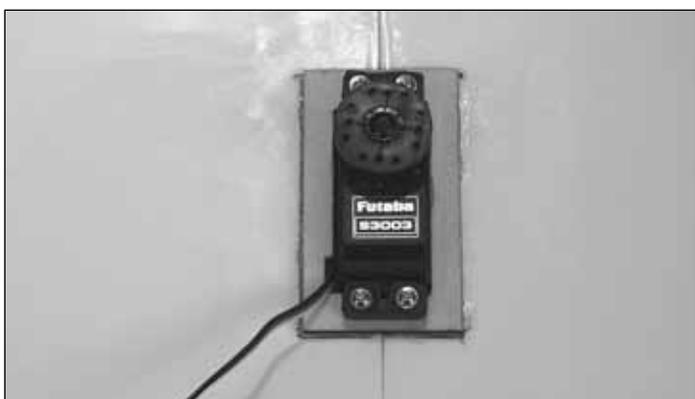
❑ 4. Cut a notch in the aileron servo tray so the wire from the servo can pass through. Install the aileron servo with the output arm towards the trailing edge of the wing. Connect it to the receiver, turn on the radio, then center the servo horn.
