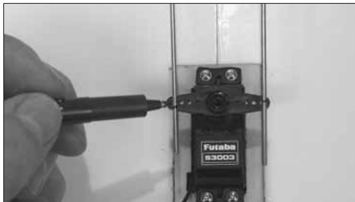
❑ 5. Thread a nylon **clevis** 13 revolutions onto the threaded end of both **6" [152mm] wire pushrods**. Install a **silicone retainer** onto each clevis. Connect each clevis to its torque rod horn. Center the ailerons, then mark the pushrods at the point where they meet the holes on the servo arm. Make a 90 degree bend down in the wires at this mark.
