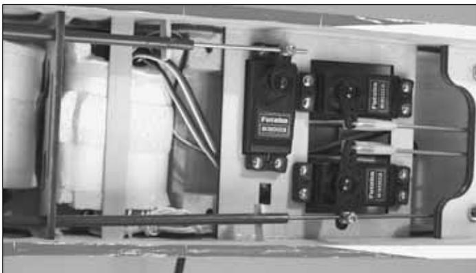
❑ 10. Use an epoxy mixing stick (or a Popsicle stick) to make small stand-offs to secure the ends of the throttle and nose wheel steering pushrod tubes. Glue them in place with epoxy or medium CA. Avoid getting any glue inside the tubes. Note the stick holding the receiver in place in the photo. Once the model has been properly balanced, use two more sticks between the fuselage sides to hold the receiver and battery securely in place.
