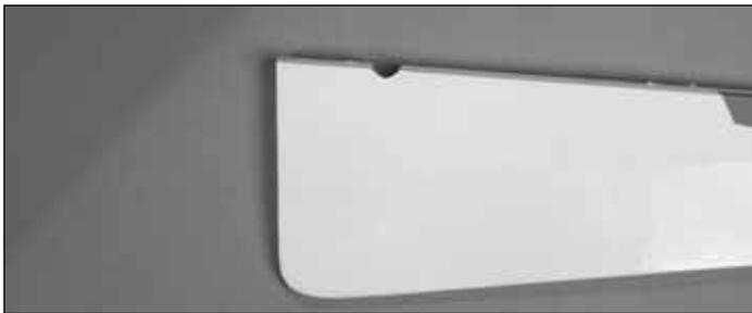
❑ 6. Temporarily install the rudder to determine where to notch the rudder to allow clearance for the elevator joiner. Press the rudder gently to leave an impression of the joiner on the rudder. Remove the rudder and cut a notch that is 1/16" [1.6mm] above and below the impression. The notch should be cut 1/4" [6.4mm] deep.
