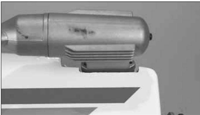
❑ 4. Make any needed cutouts for the muffler to allow for at least 1/4" [6.4mm] clearance around the muffler. Be sure to fuelproof any exposed wood around the needle and muffler cutouts. Install the engine, making sure the muffler screws are on the engine. Install the muffler on the engine. You may need a muffler extension for your motor.
