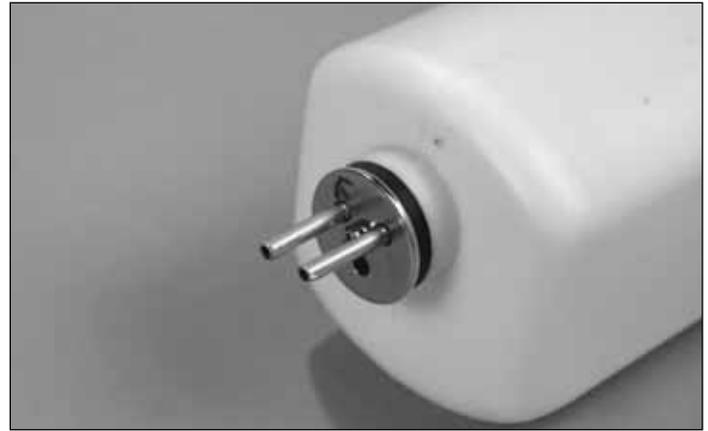
❑ 4. Push the stopper assembly into the tank and check the fit of the parts. The end of the bent tube should just touch the top of the tank. Rotate the tank around with the stopper facing up. The clunk should not touch the back of the tank. When the parts fit properly, tighten the screw on the stopper assembly. Mark the tube that is connected to the clunk. In the above photo, we marked the tube on the right side of the tank with an "F", for fuel.
