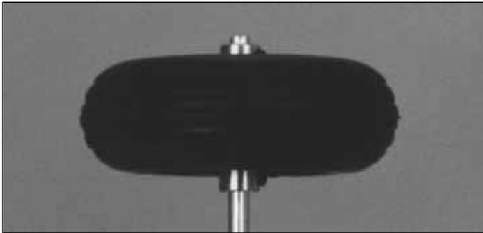
1. Install the three **wheels** using the six **5/32" [4mm] wheel collars** and **set screws**. Grind or file a flat spot at the point of the set screw contact for each of the outer collars. This provides a better area for the set screw to "bite" and helps keep the wheels in place.
