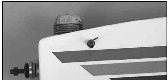
❑ 1. Mark the position of the needle valve for your engine installation. Also, mark the fuselage for any cutouts you will need for the muffler, then remove the engine from the mount. Cut or drill the fuselage side to allow for ease of needle valve adjustments. Leave a space around the needle valve so that any vibrations will not affect the needle setting.
